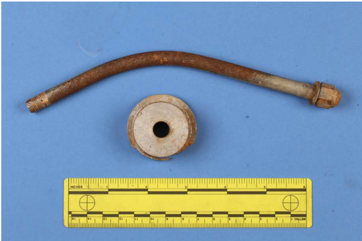
Figure 1: Nose landing gear wheel attach bolt as received.
