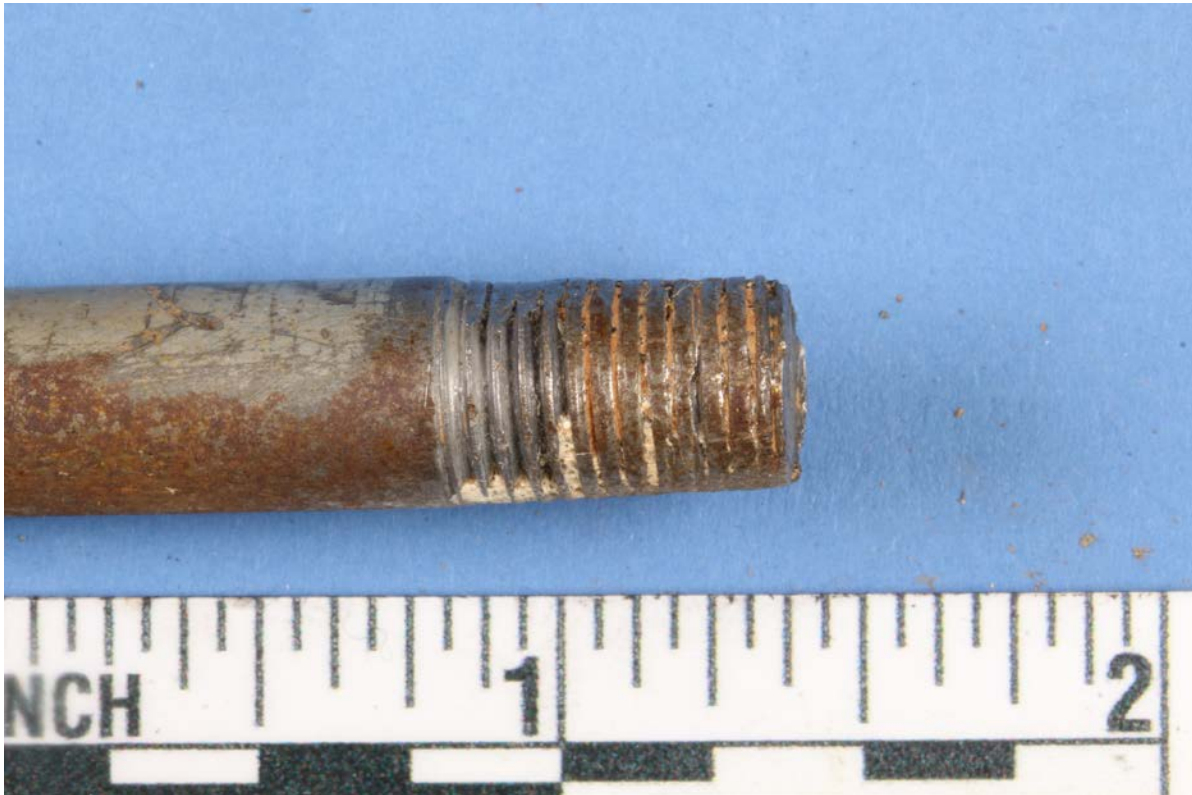
Figure 3: Damaged threads at end of wheel attach bolt (alternate view).
