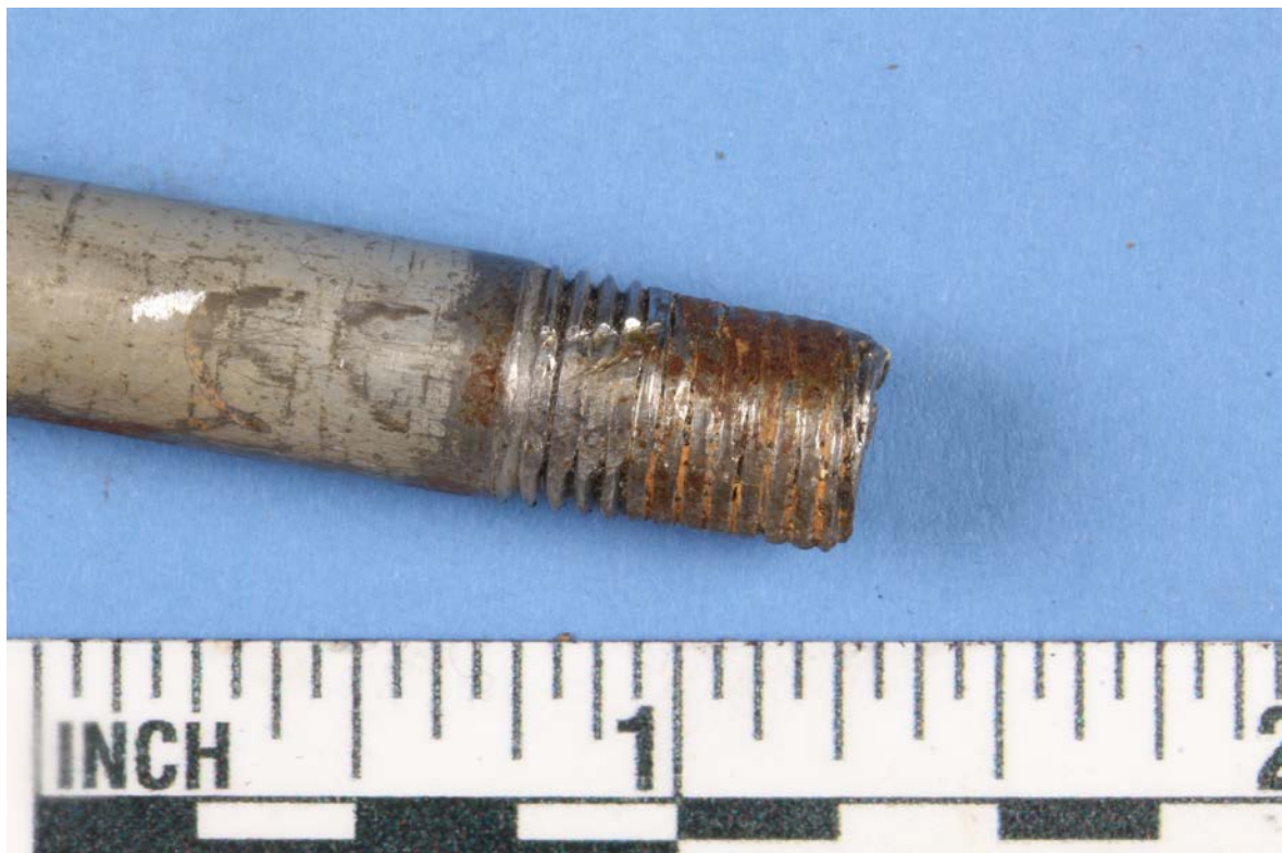
Figure 2: Damaged threads at end of wheel attach bolt.
