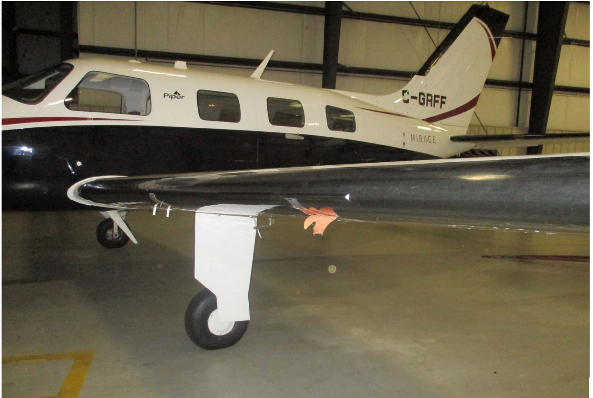
Photo 1 – Photograph of damage on accident airplane from striking stop sign.
