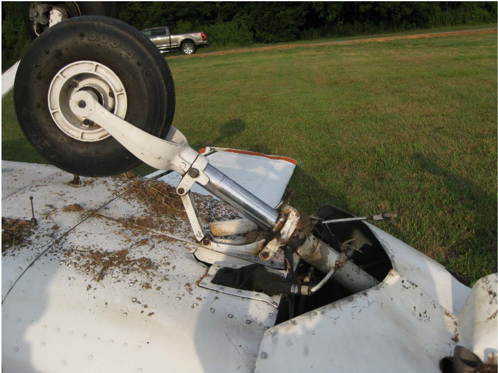
Photo 3 – Nose Gear Damage (FAA Photo)
