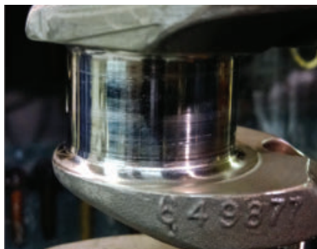
This Continental IO-360 spun a main bearing after cylinder work. Fortunately, the situation was caught at a routine oil change (where the filter was found to have thousands of flakes of bearing metal) literally an hour or two before the engine would have self-destructed in flight.
