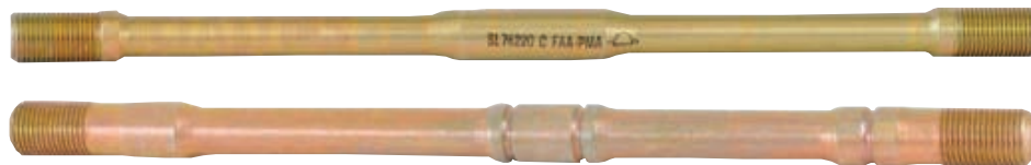
A pair of new through bolts for Lycoming (top) and Continental (bottom) engines. Both have 1/2-inch cad-plated steel threads. The Continental through bolts are stiffer (larger shank diameter) and have grooves for O-rings.
