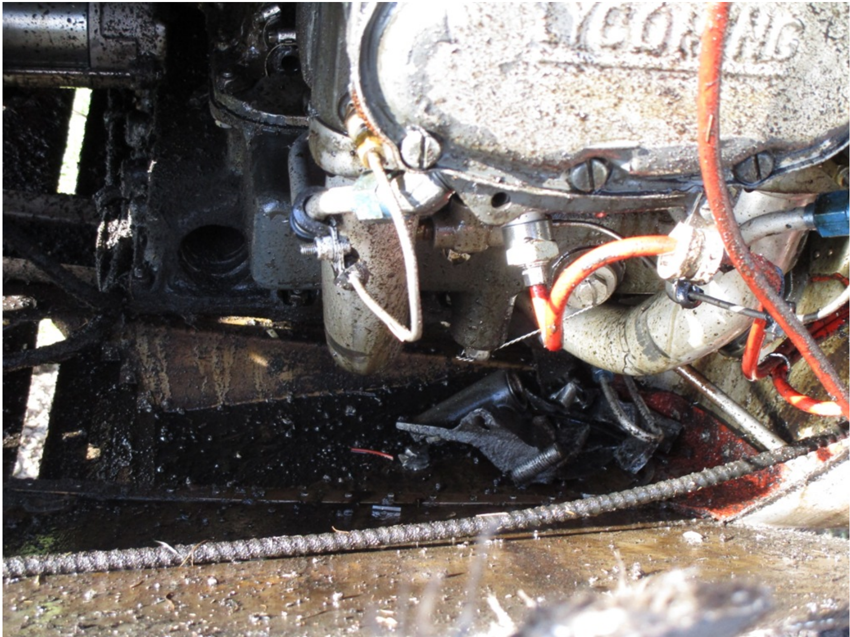
Photo 6 – Broken Sections of Crank Case in Lower Engine Cowling (Photo Credit: FAA)
