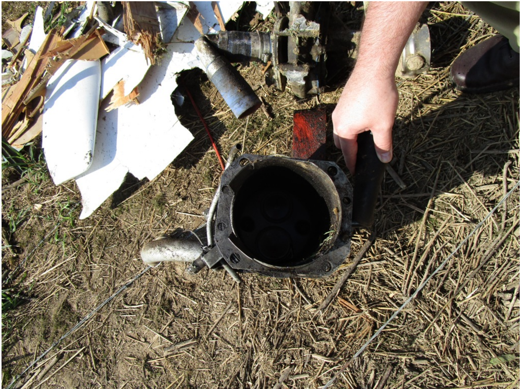
Photo 4 – No. 2 Cylinder Separated from Engine (Photo Credit: FAA)
