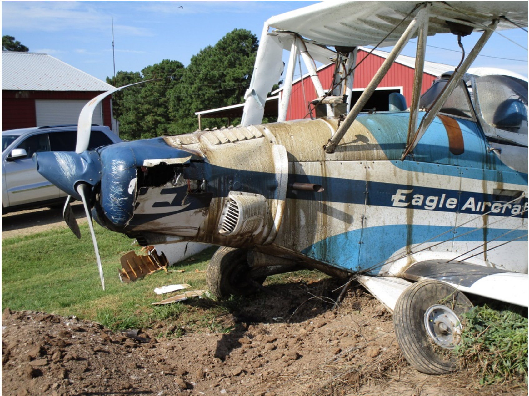
Photo 2 – Hole in Engine Cowling and Oil Residue (Photo Credit: FAA)
