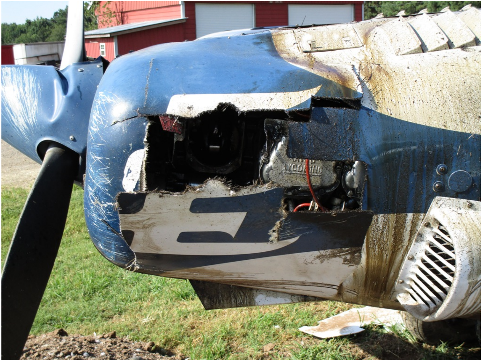
Photo 3 – Hole in Left Side Engine Cowling (Photo Credit: FAA)
