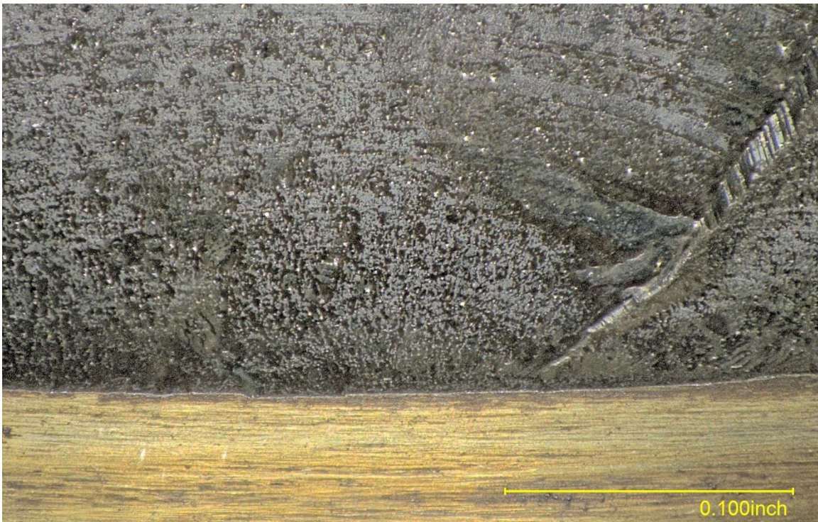
Figure 8 – Closer view of the aft crack initiation sites, with a prominent ratchet mark present on the right.
