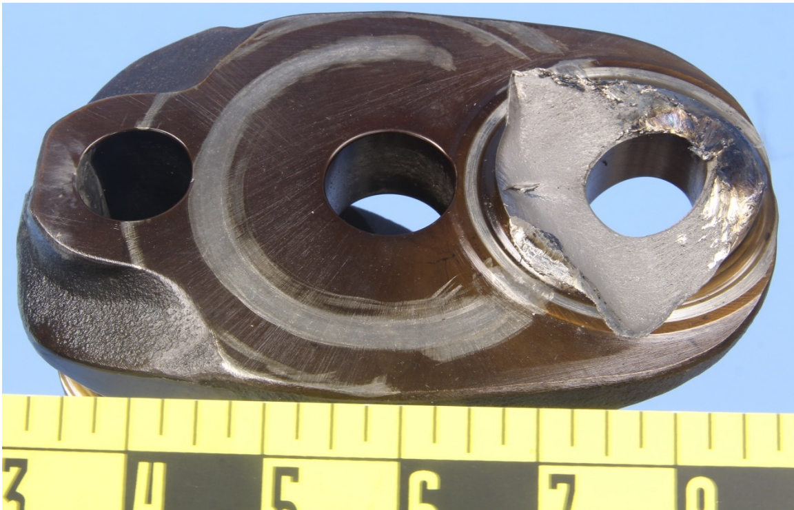
Figure 4 – Angled view of the forward fracture surface.
