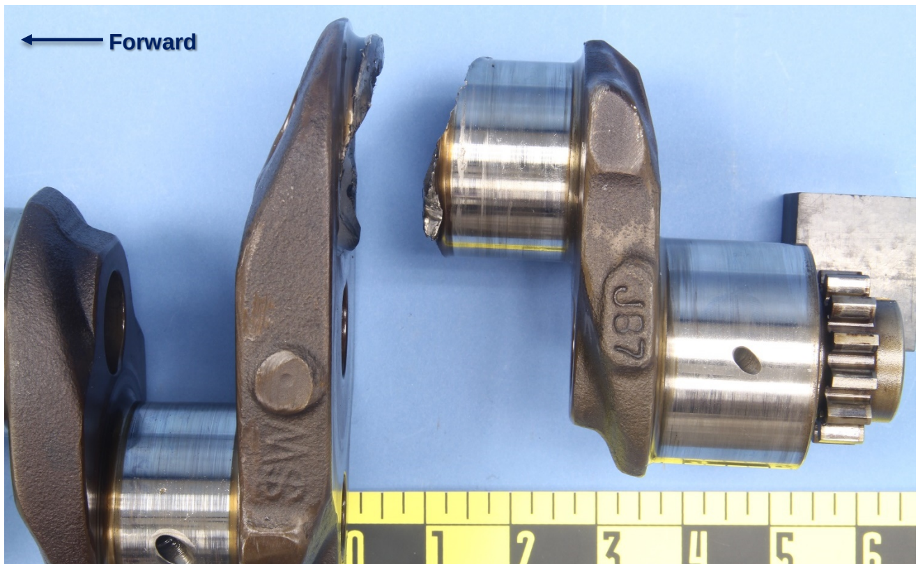
Figure 2 – The mating halves of the fractured #4 cylinder journal of the received crankshaft.
