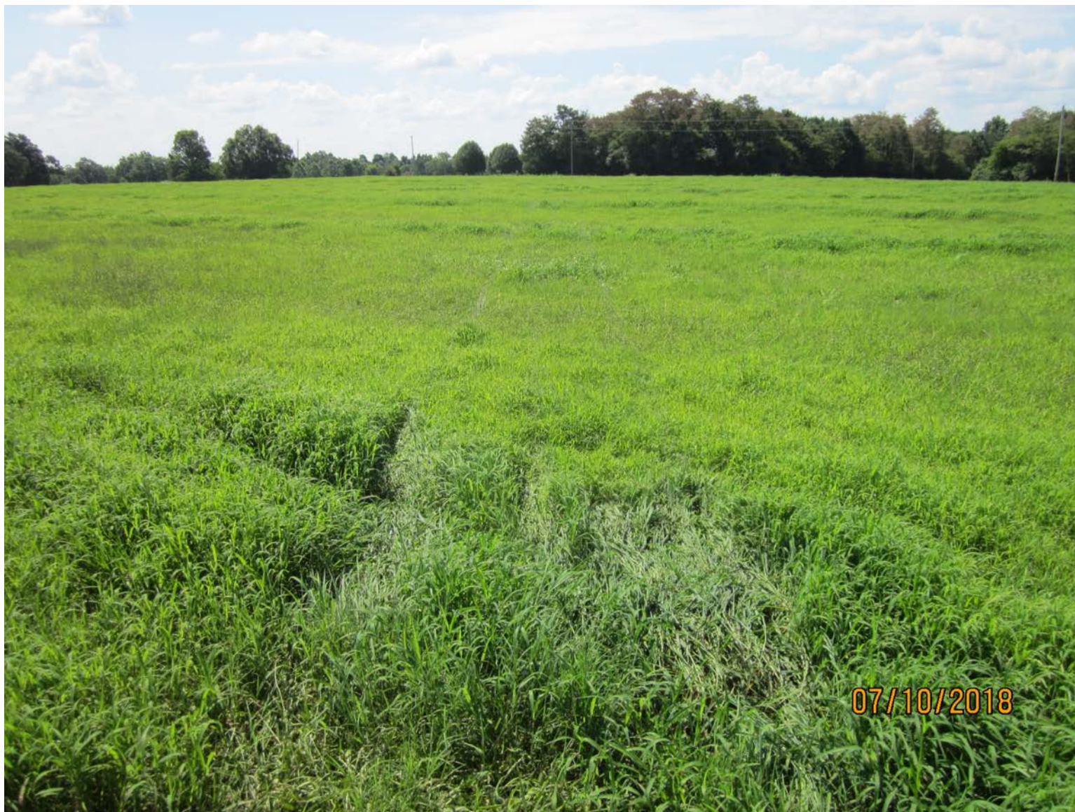
Photo 6 – Landing gear wheel tracks in grass bordering runway looking southeast. Grass is the same type that was found wrapped around landing gear. (Courtesy of FAA)
