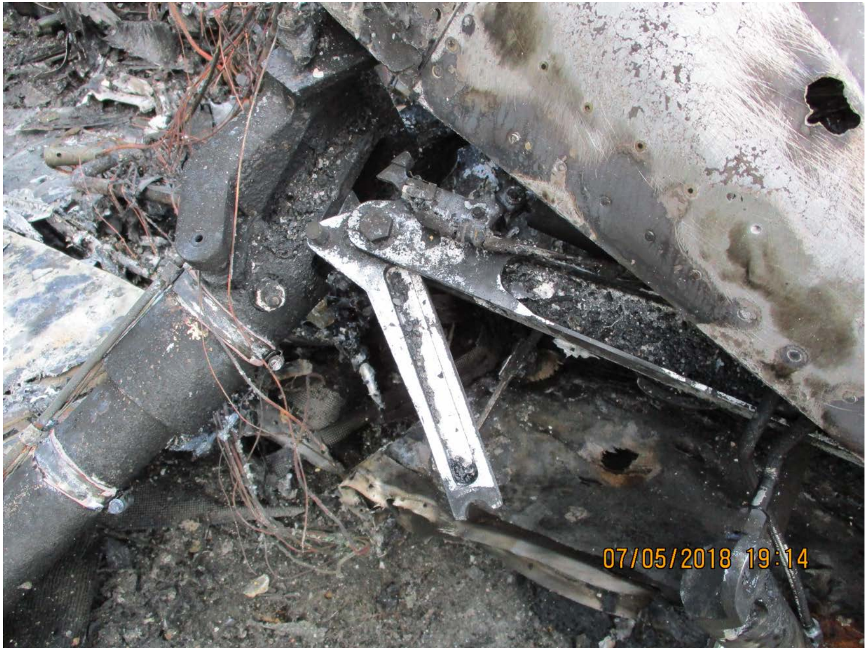
Photo 5 – left main landing gear broken downlock link.
