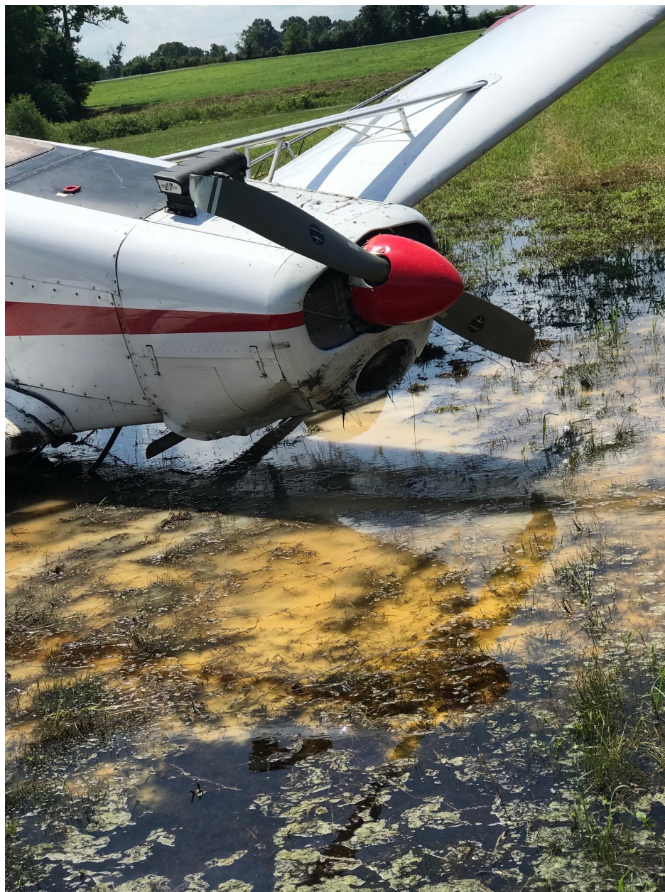
Photo 1 – Close up of front of airplane damage. (Courtesy of FAA)
