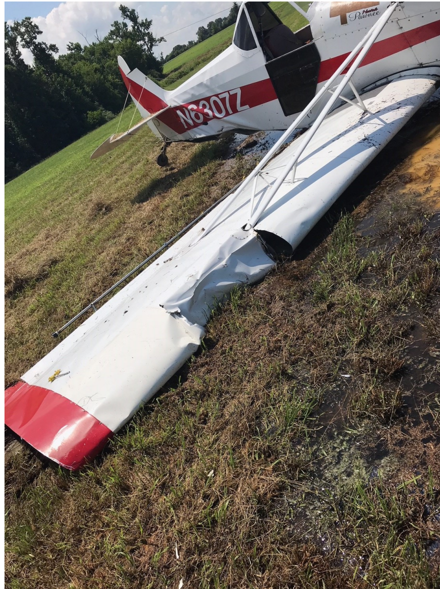
Photo 4 – Right side of airplane showing wing leading edge and fuselage damage. (Courtesy of FAA)
