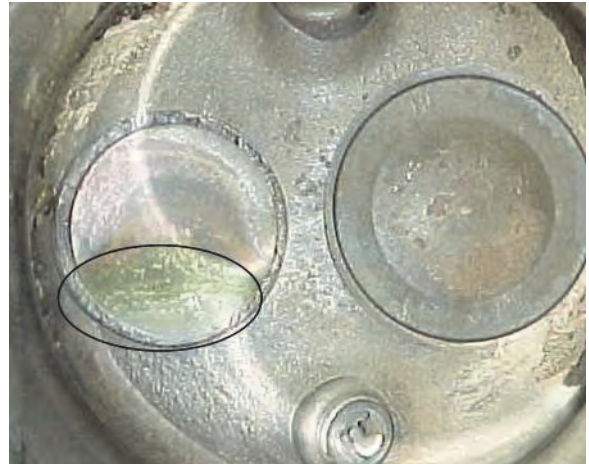
Figure 6-68. Burned Exhaust Valve
