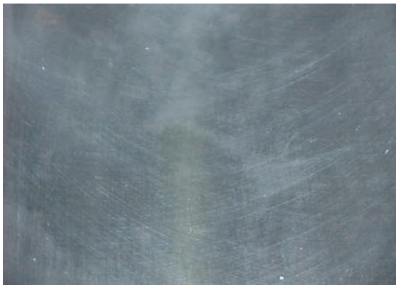
Figure 6-69. Phosphate-Coated Cylinder w/ Revised Hone Pattern
