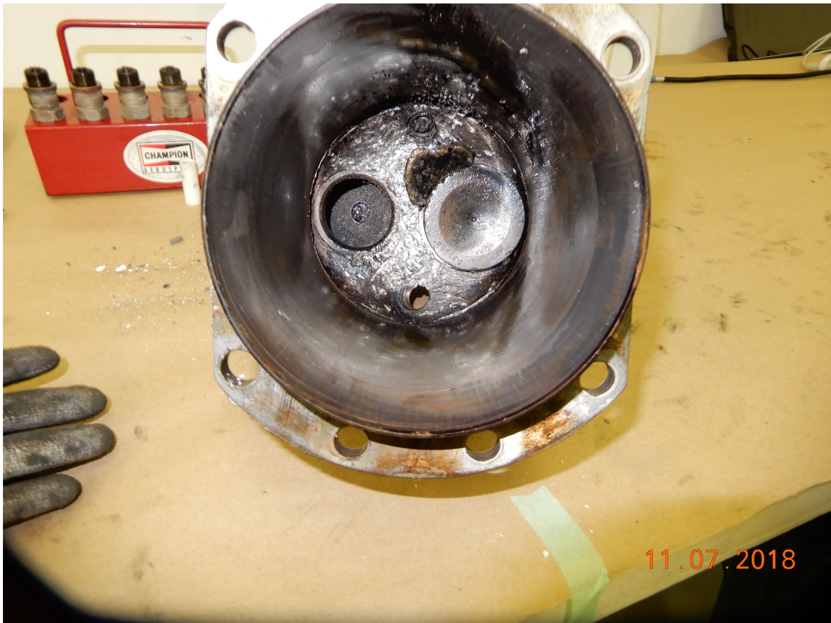
Photo 3 – View of the damage to the No. 3 cylinder.
