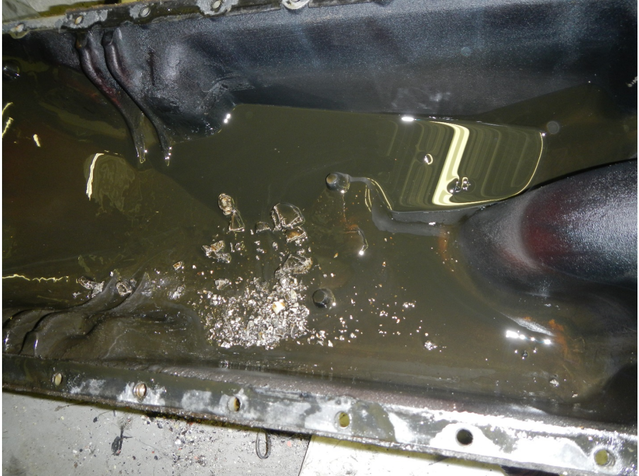
Figure 9: Oil sump contents (Courtesy Continental Motors)
