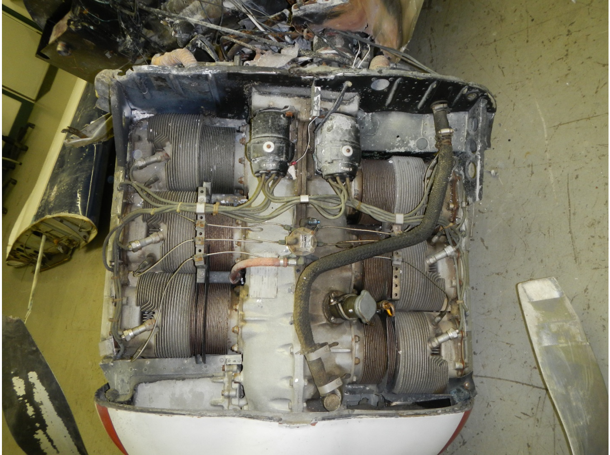
Figure 5: Top of engine with cowling removed (Courtesy Continental Motors)
