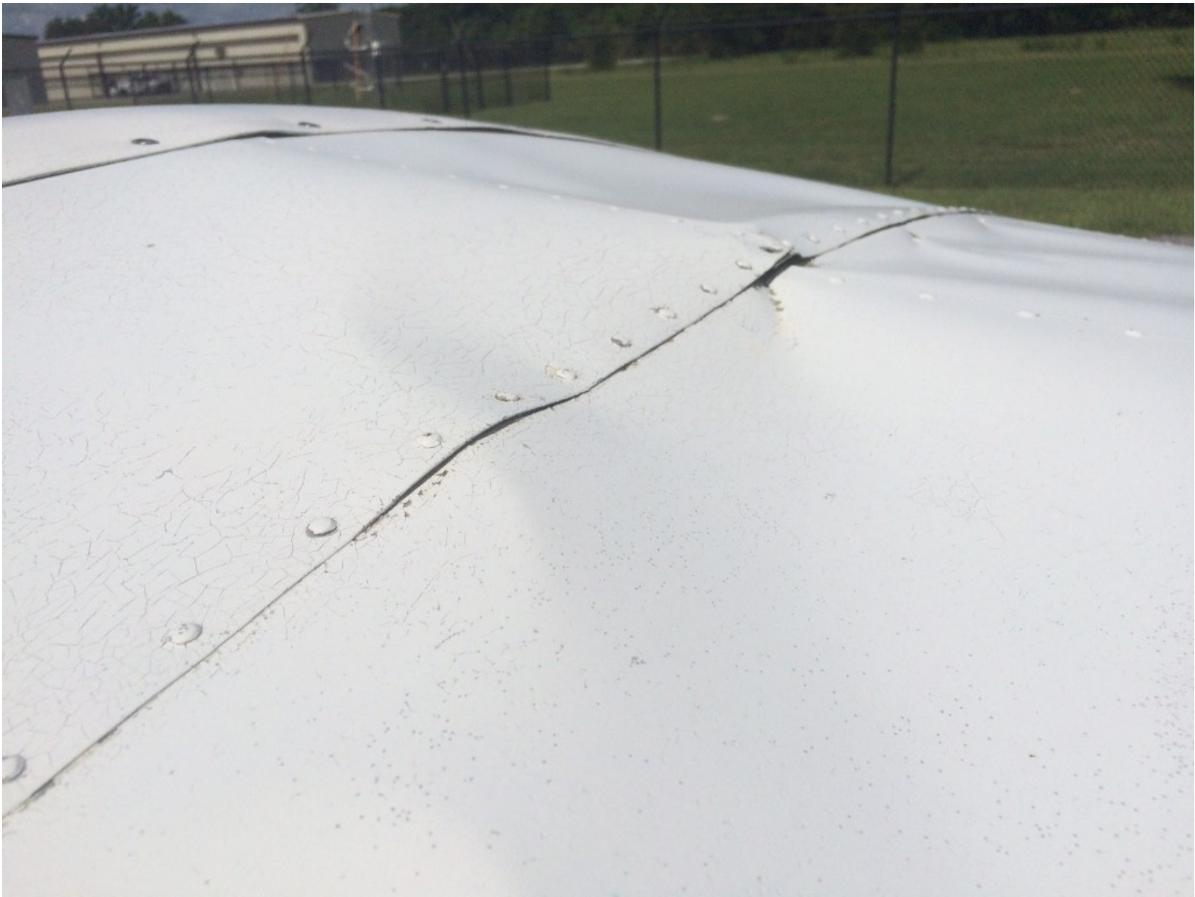
Photo 2 - FAA Digital Photograph. View Depicting the Damage to the Outer Section of the Right Wing.
