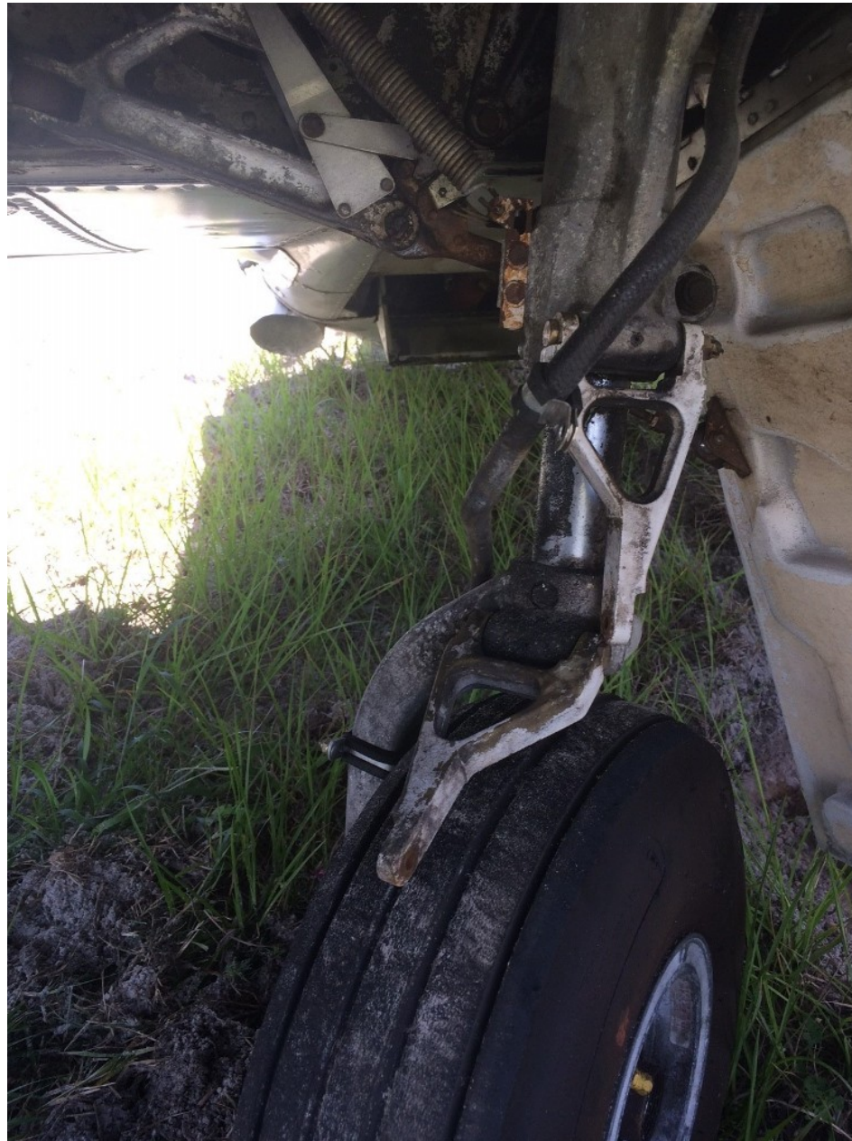
Photo 3 - FAA Digital Photograph. View Depicting the Separated Upper and Lower Undamaged Torque Links of the Right Main Landing Gear
