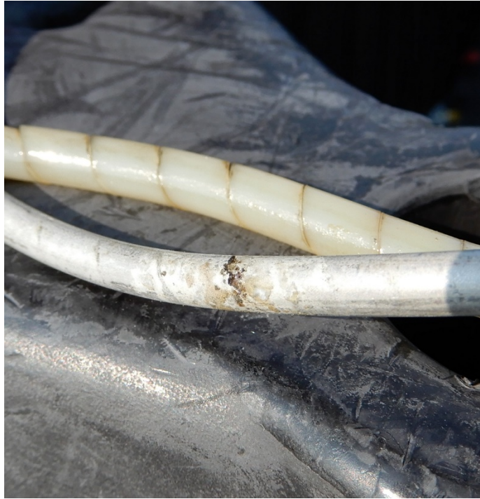
Figure 2. Pitted area in hydraulic line where fluid leaked.
