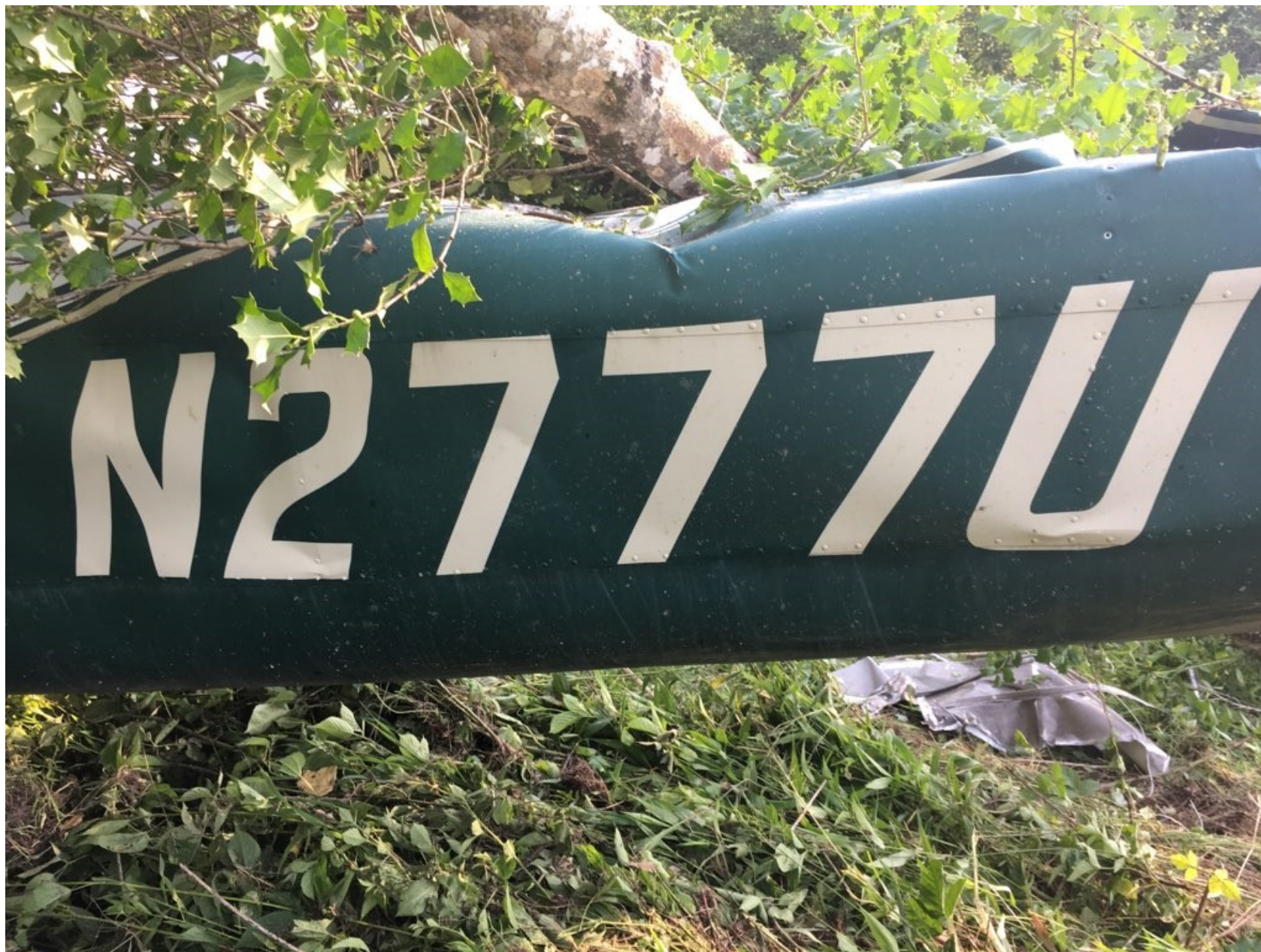
Photo 3 - View of left side of empennage showing buckling
