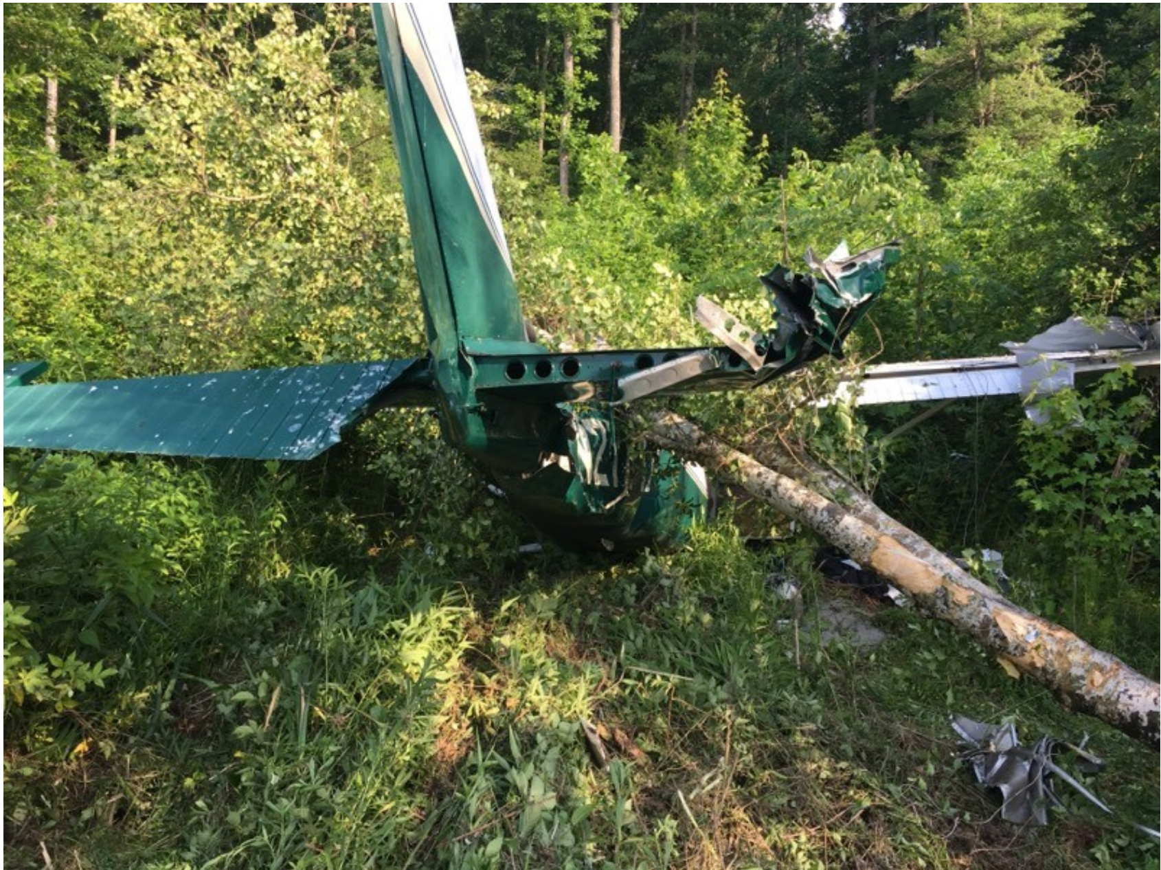
Photo 4 – View of horizontal and vertical stabilizer showing buckling
