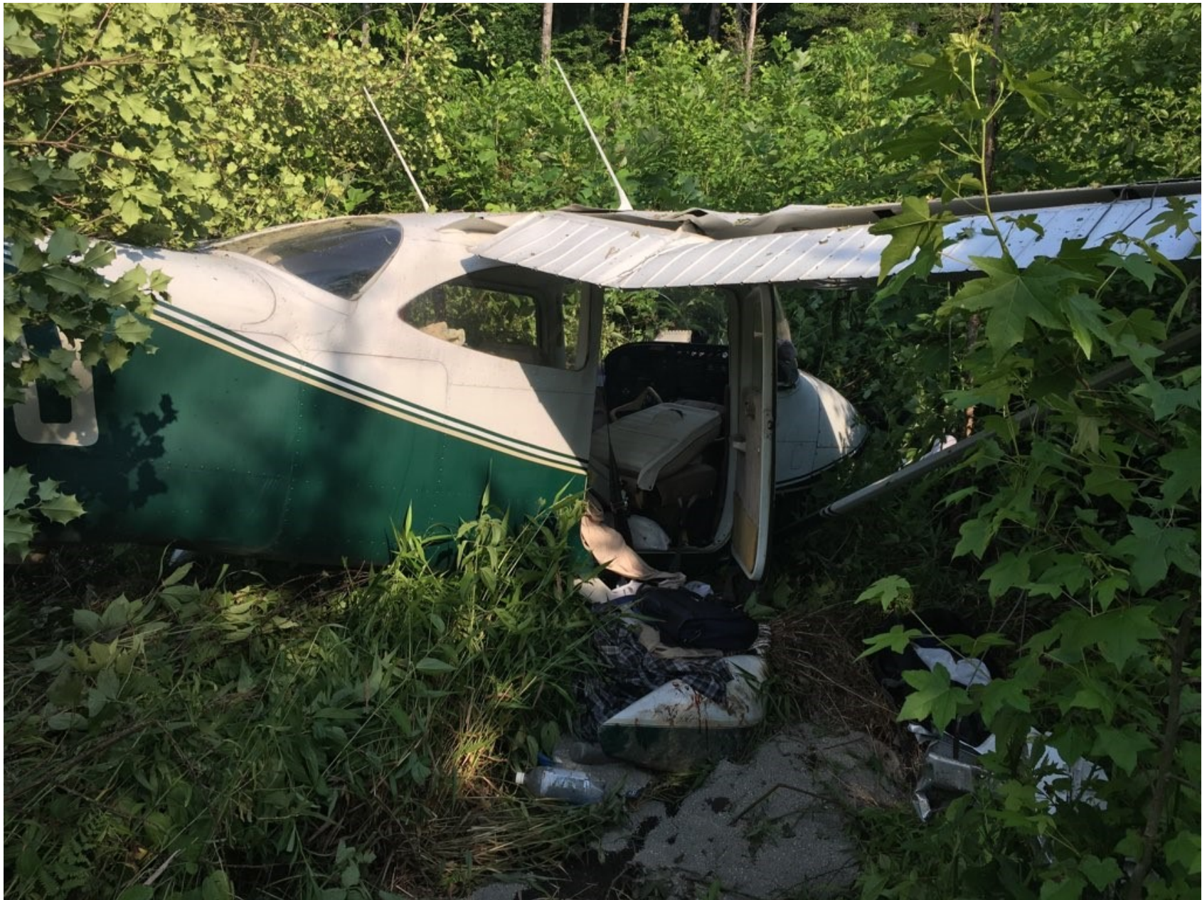
Photo 1 – View of right side of fuselage showing buckling of wing and cabin section
