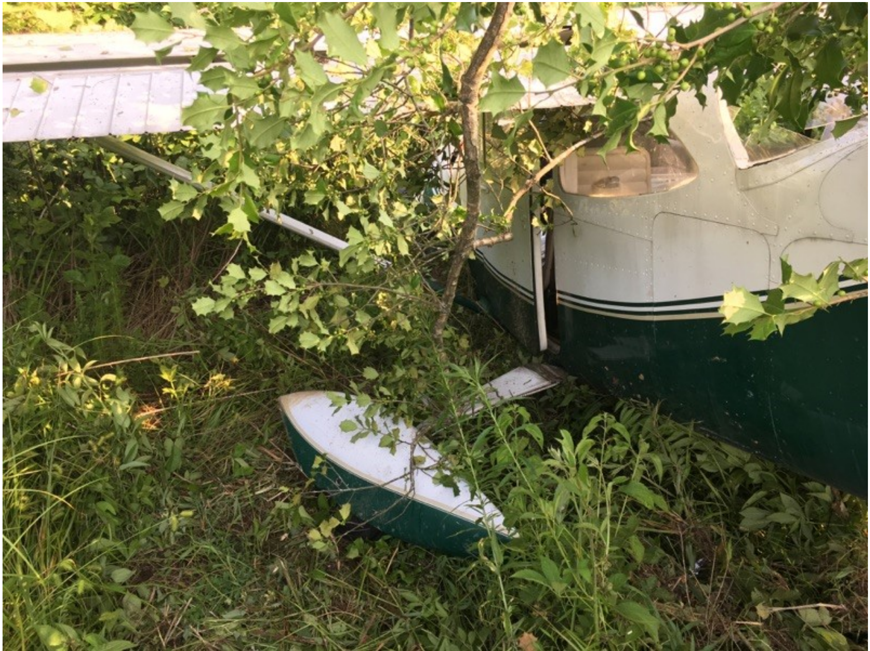
Photo 2 - View of left side of fuselage showing collapsed left main landing gear
