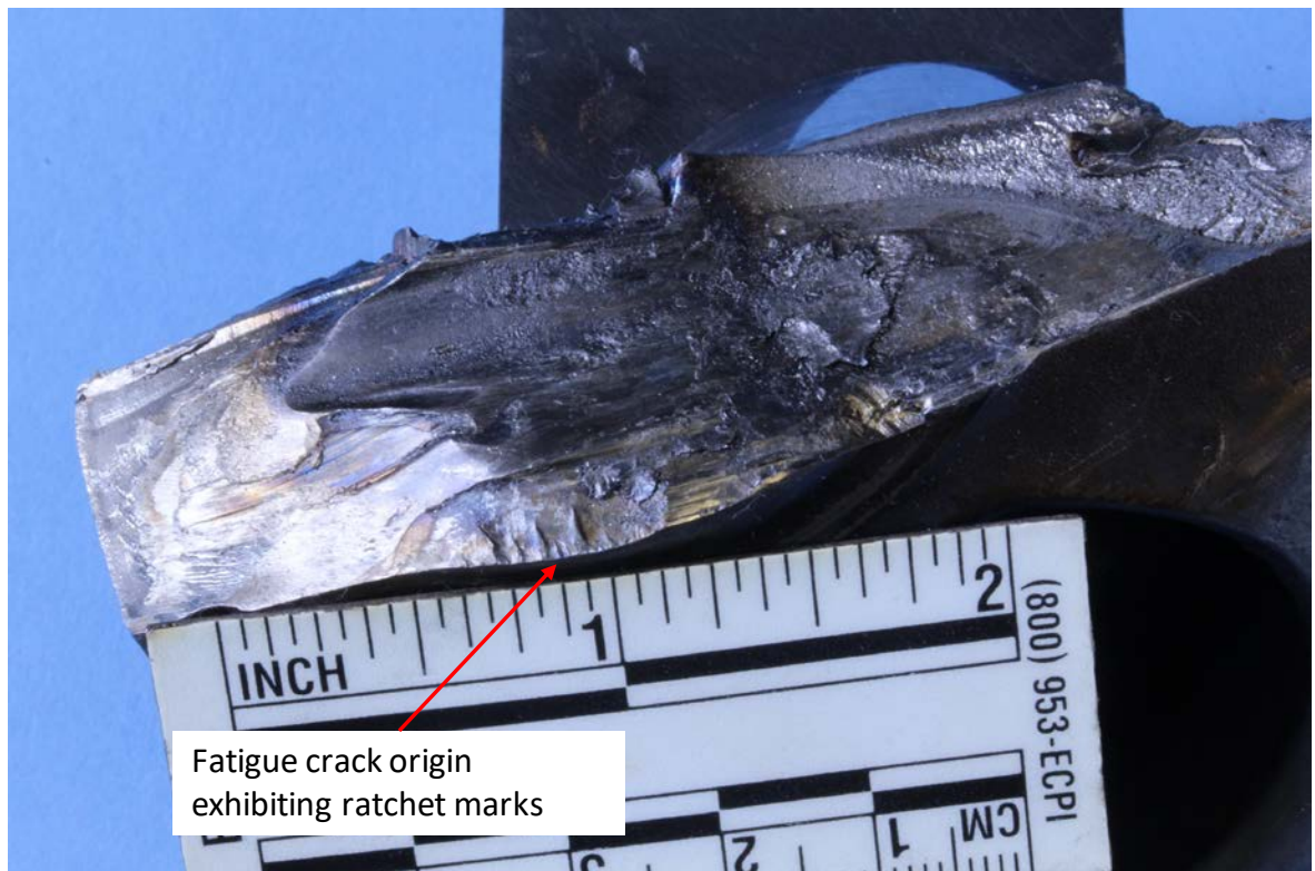
Figure 2: Fracture surface exhibiting ratchet marks at crack origin.
