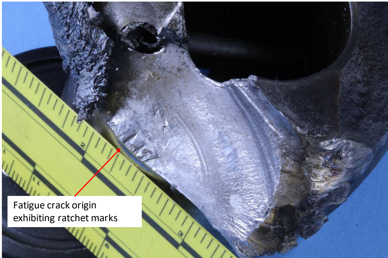
Figure 3: Fracture surface exhibiting ratchet marks and crack arrest marks.
