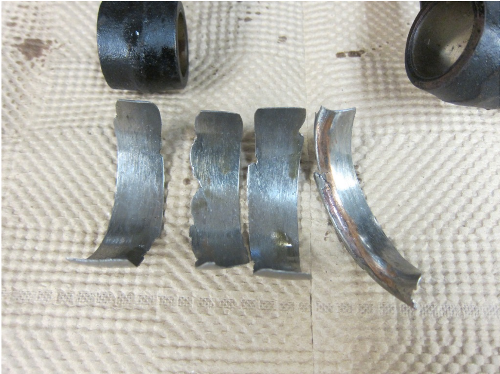
Photo 11 – No. 2 Main Bearing (Photo Credit CAT)
