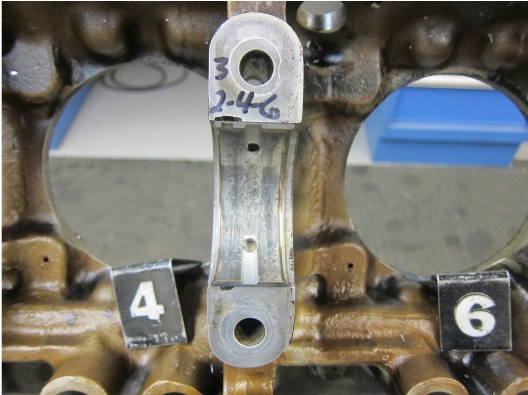
Photo 15 – No. 3 Main Bearing (Photo Credit CAT)
