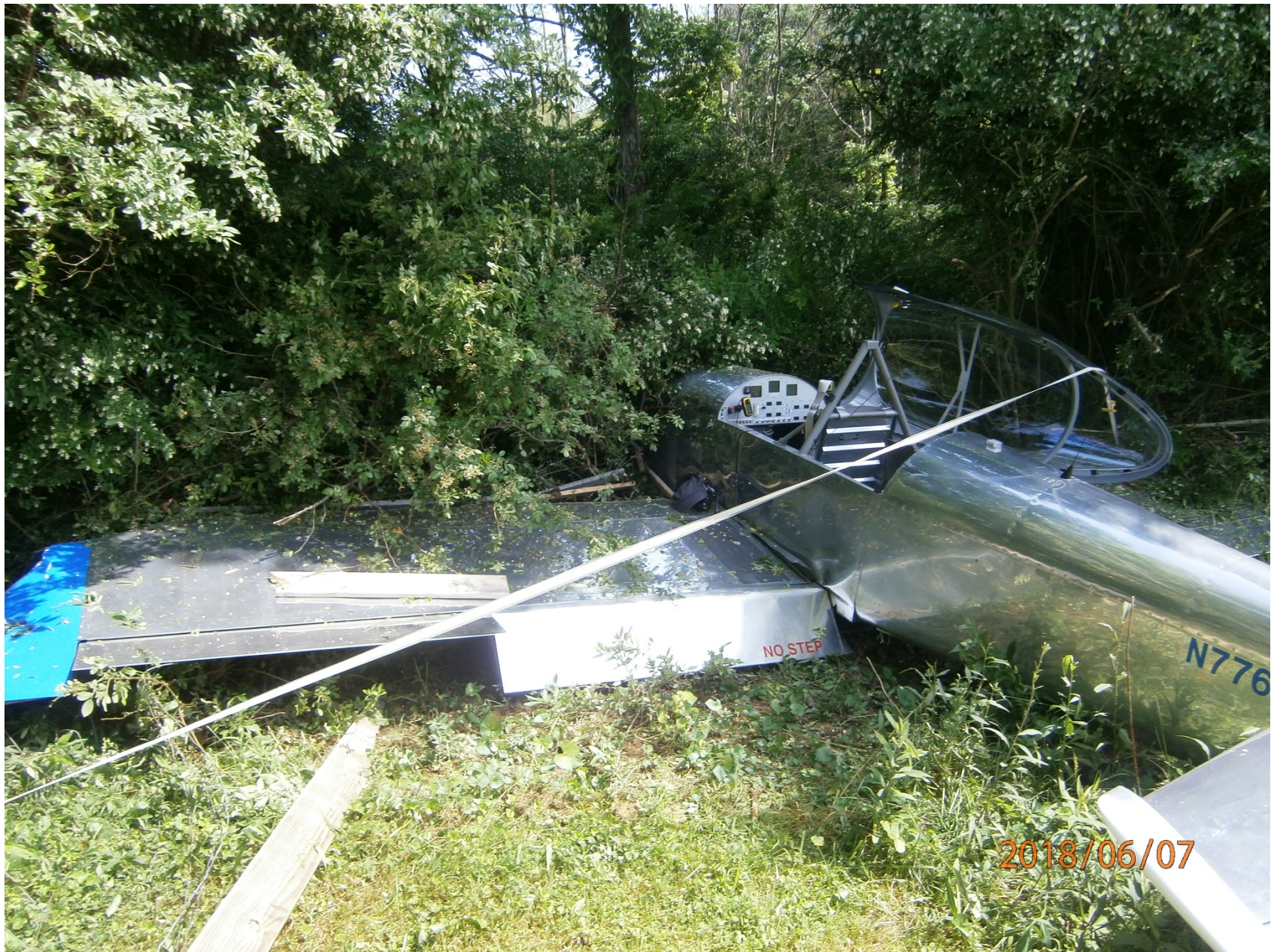
Photo 2 - Substantially Damaged Left Wing and Fuselage (Photo Courtesy of FAA)
