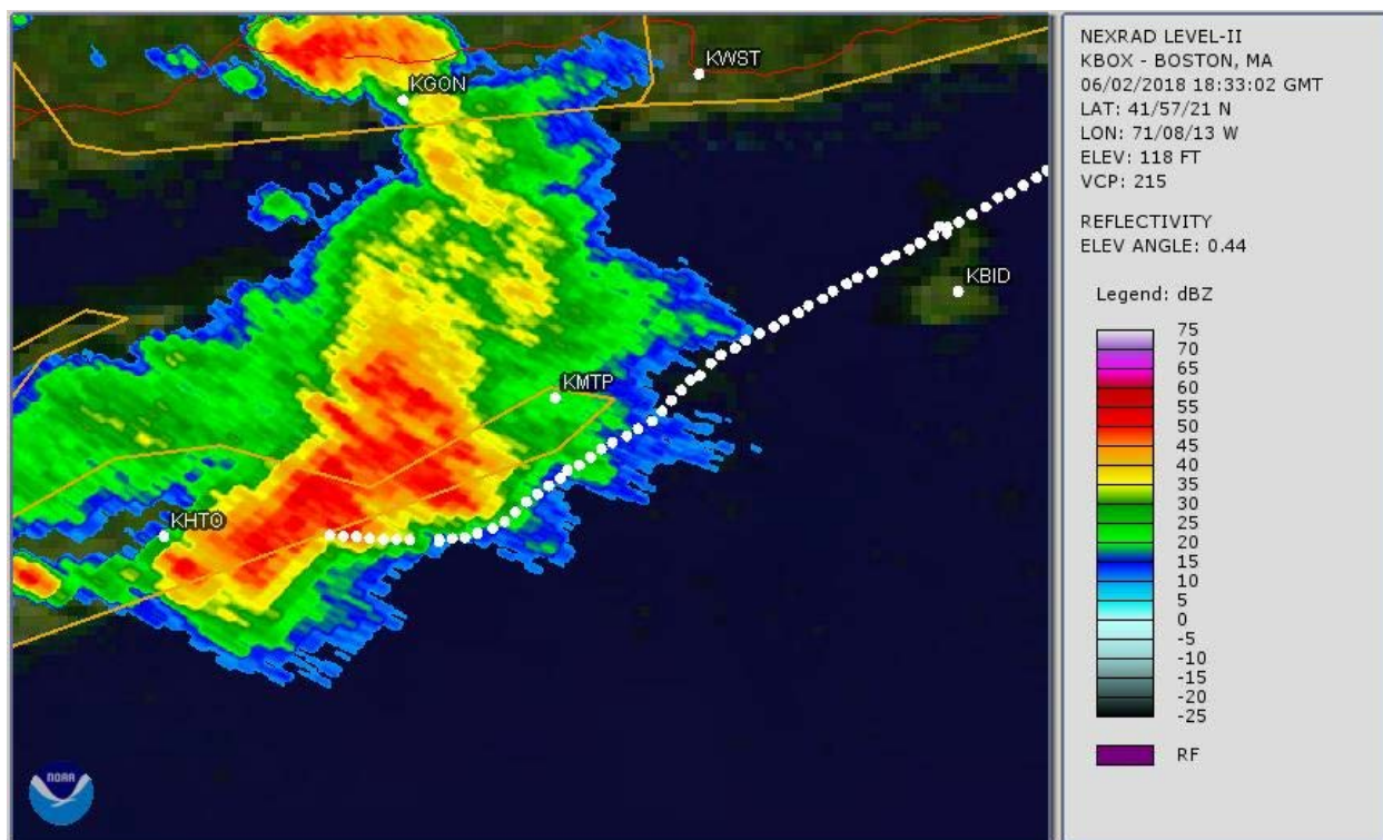
Figure 21 - KBOX WSR-88D 0.44° base reflectivity image at 1433 EDT with flight track
