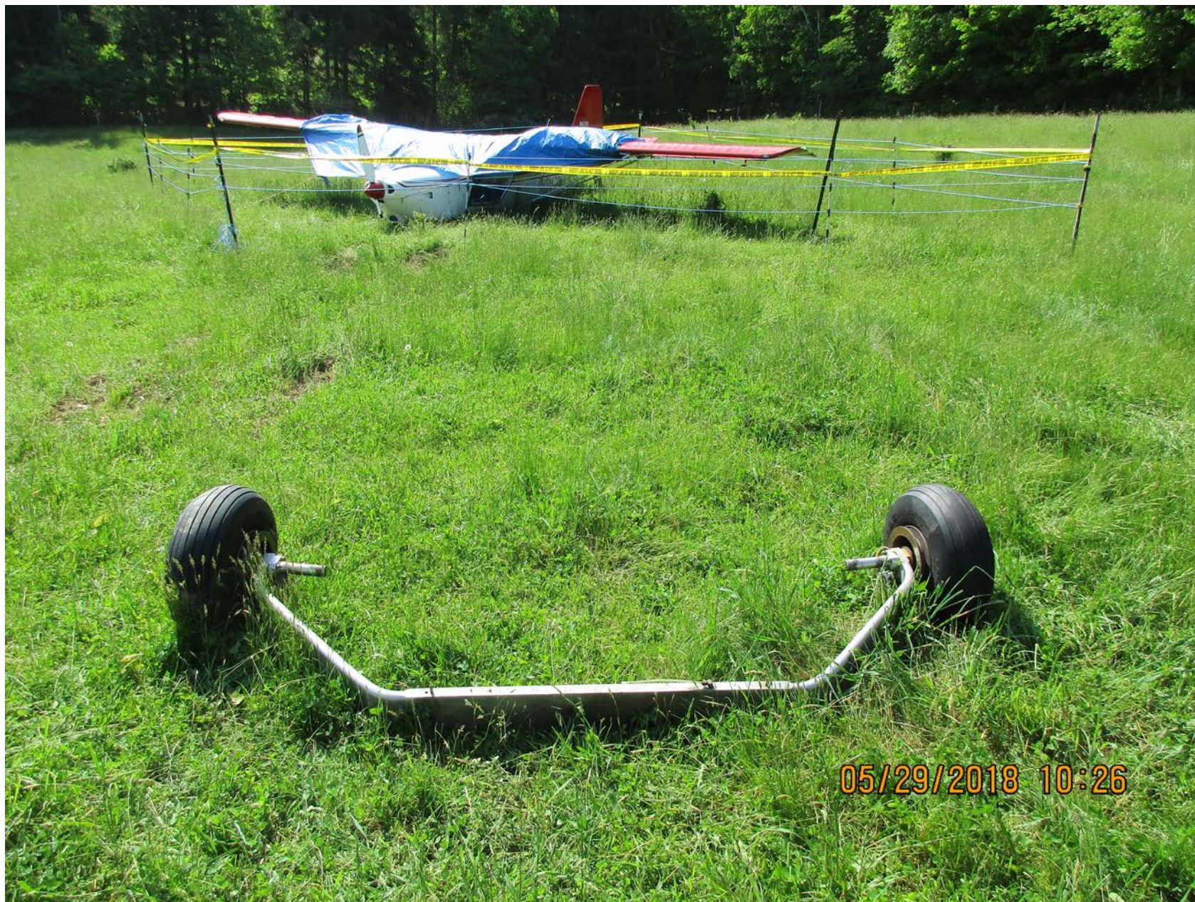
Photo 3 – View of airplane and separated main landing gear (Courtesy of the FAA)
