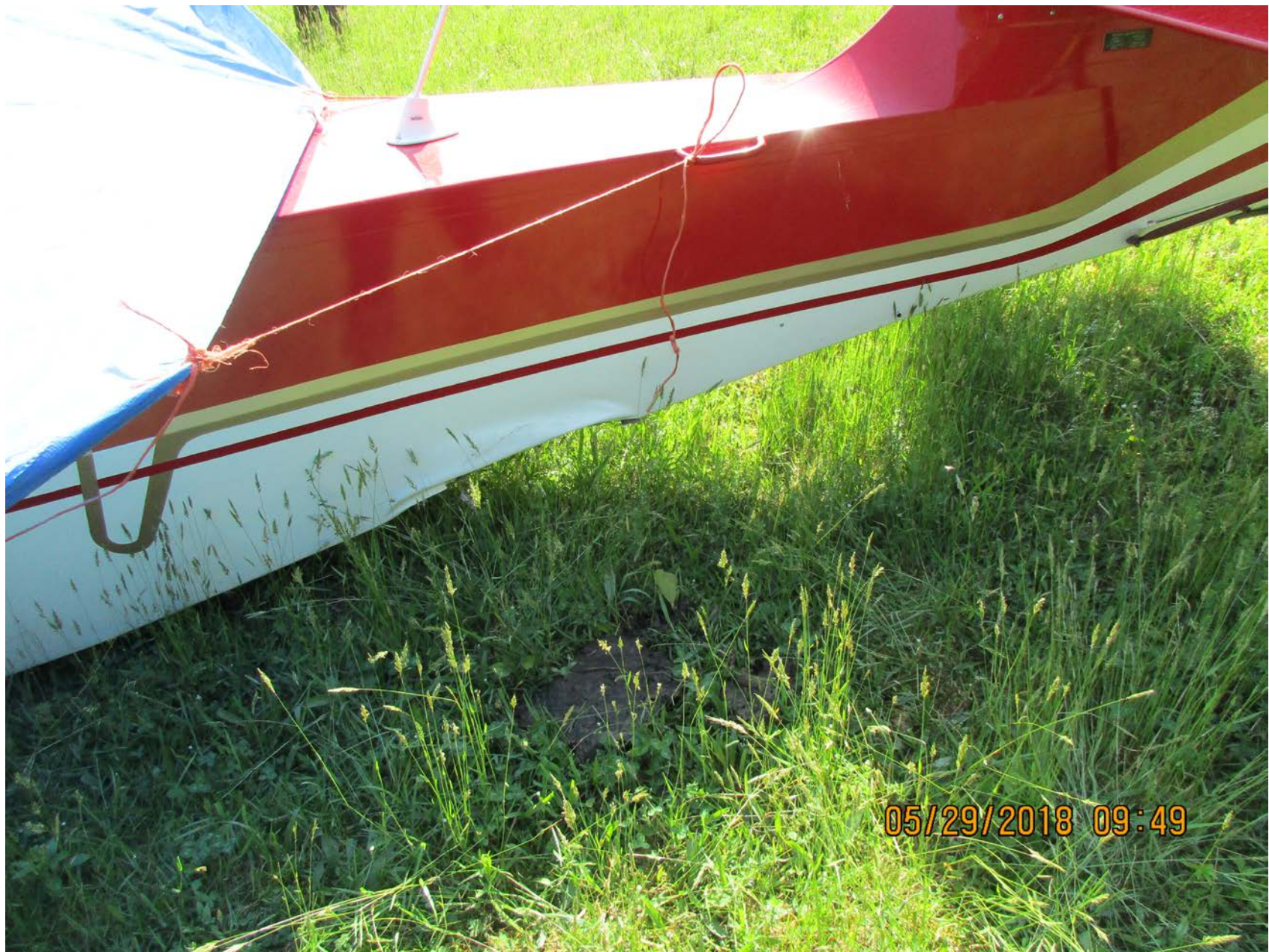
Photo 2 – View of empennage buckling (Courtesy of FAA)
