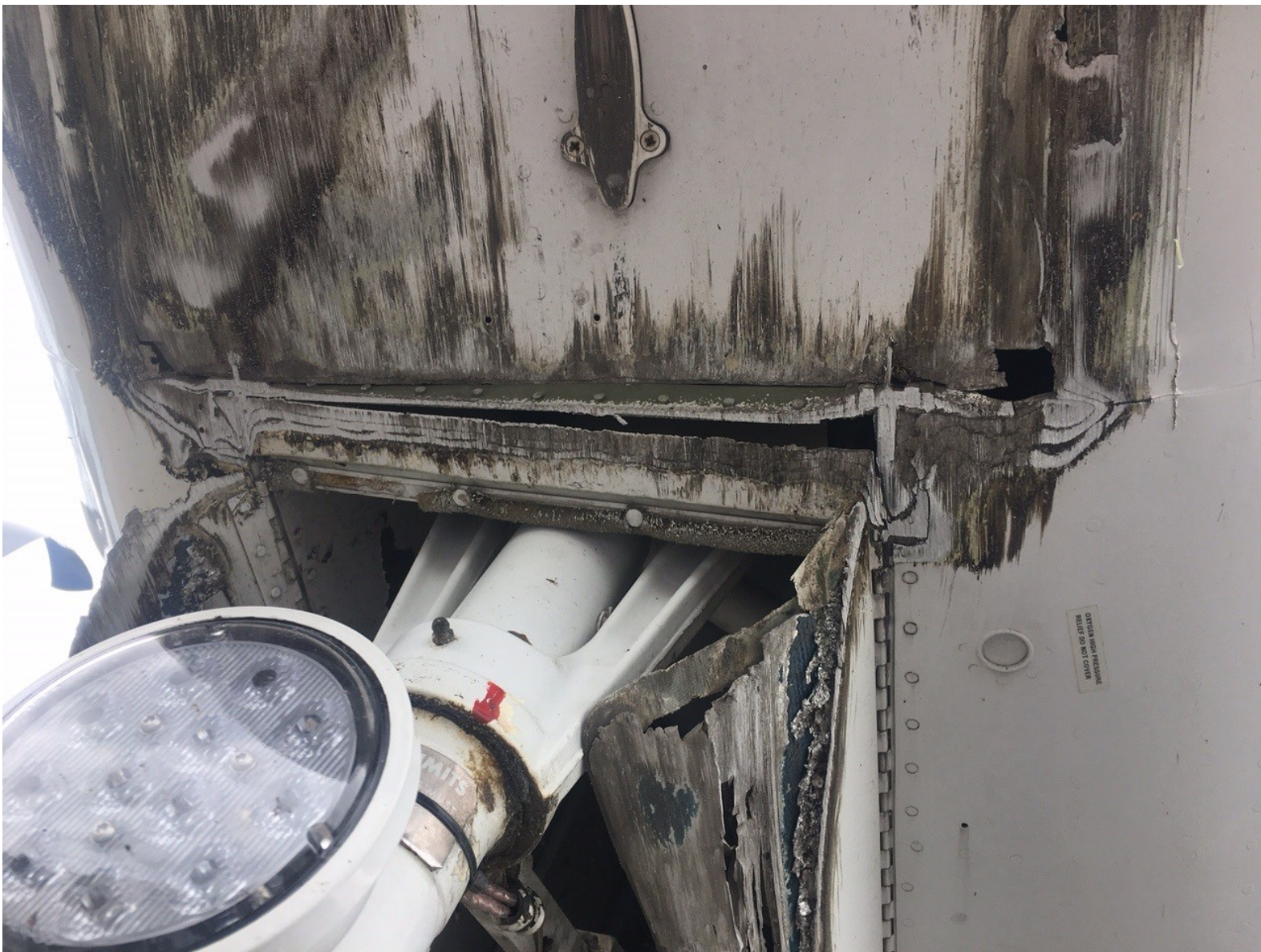
Photo 3 – Closeup view of nose gear and damage. (Courtesy of FAA)
