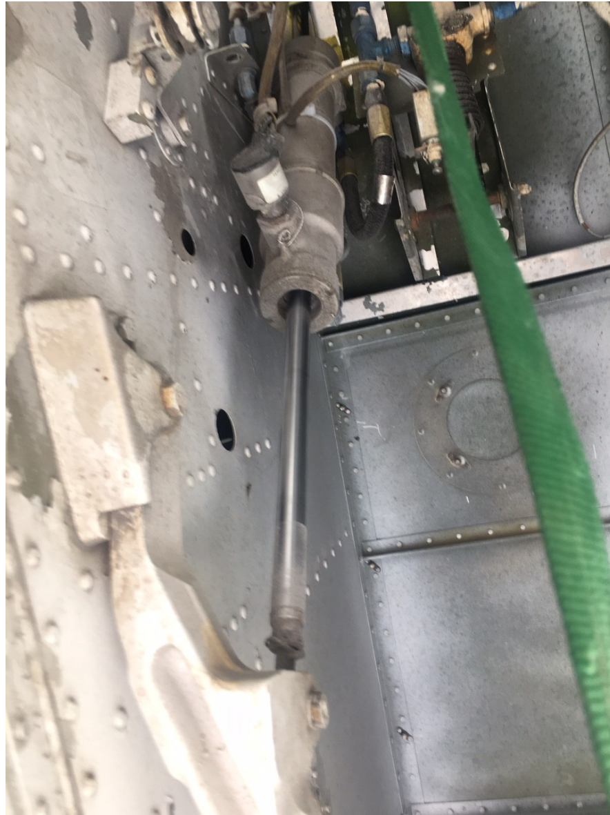
Photo 4 – View of nose gear actuator. (Courtesy of FAA)
