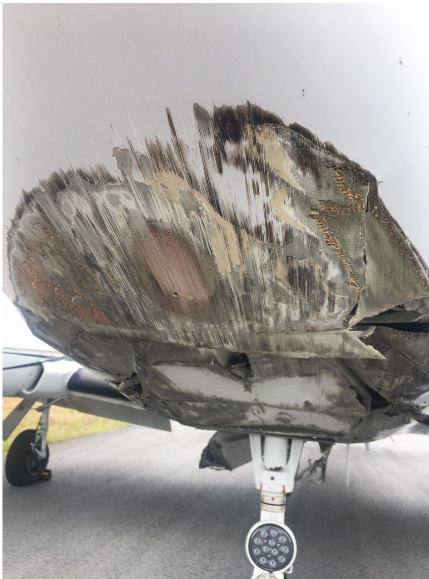
Photo 2 – View of nose gear and surrounding damage. (Courtesy of FAA)
