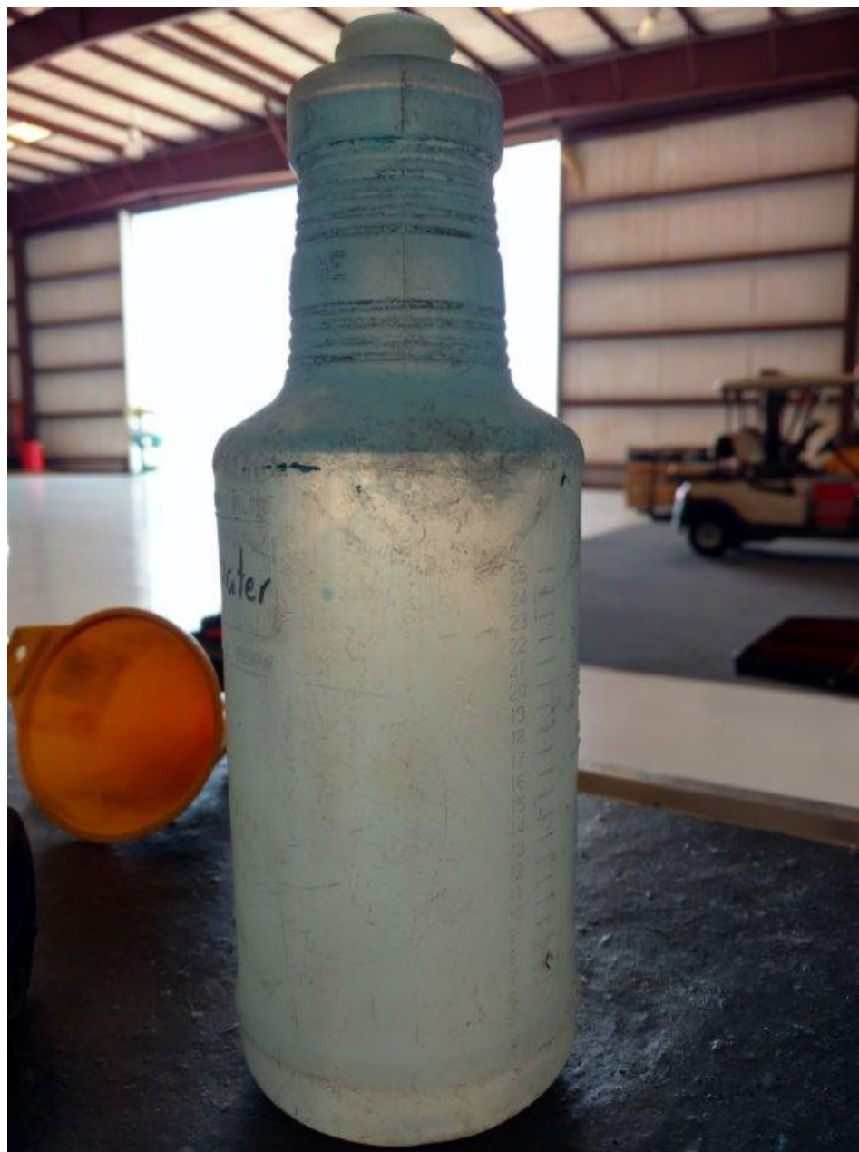
Photo 4 – View of Water/Fuel Drained from Fuel System (FAA)
