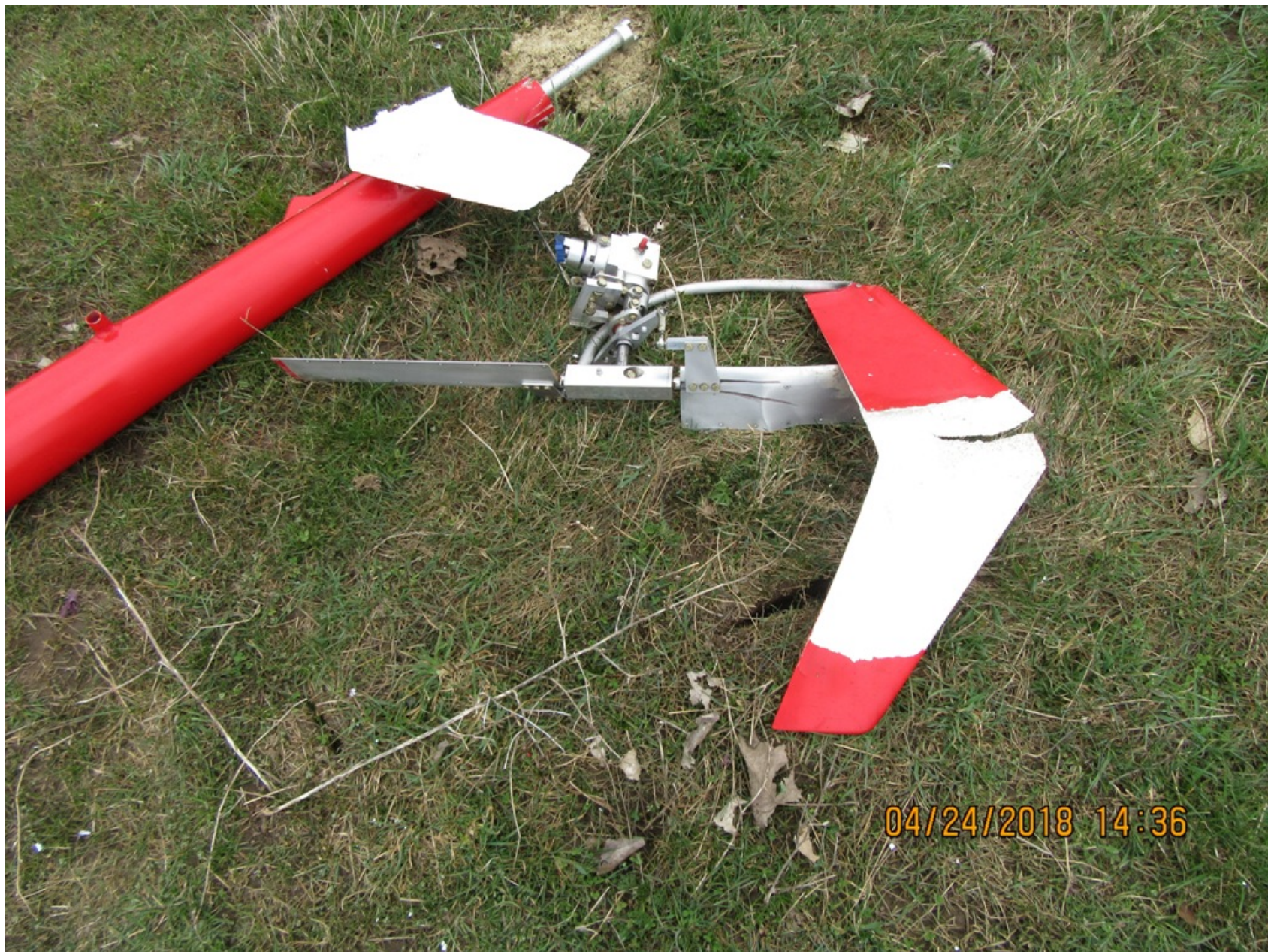
Photo 3 - FAA Digital Photograph. View of a Portion of the Tailboom and Separated tail Rotor Assembly.
