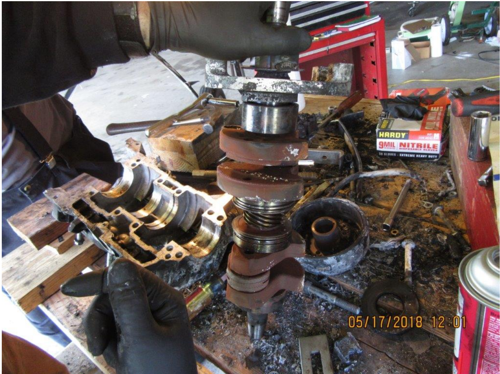
Photo 5 - FAA Digital Photograph. View of the Crankshaft and Engine Crankcase Half During the Engine Examination.
