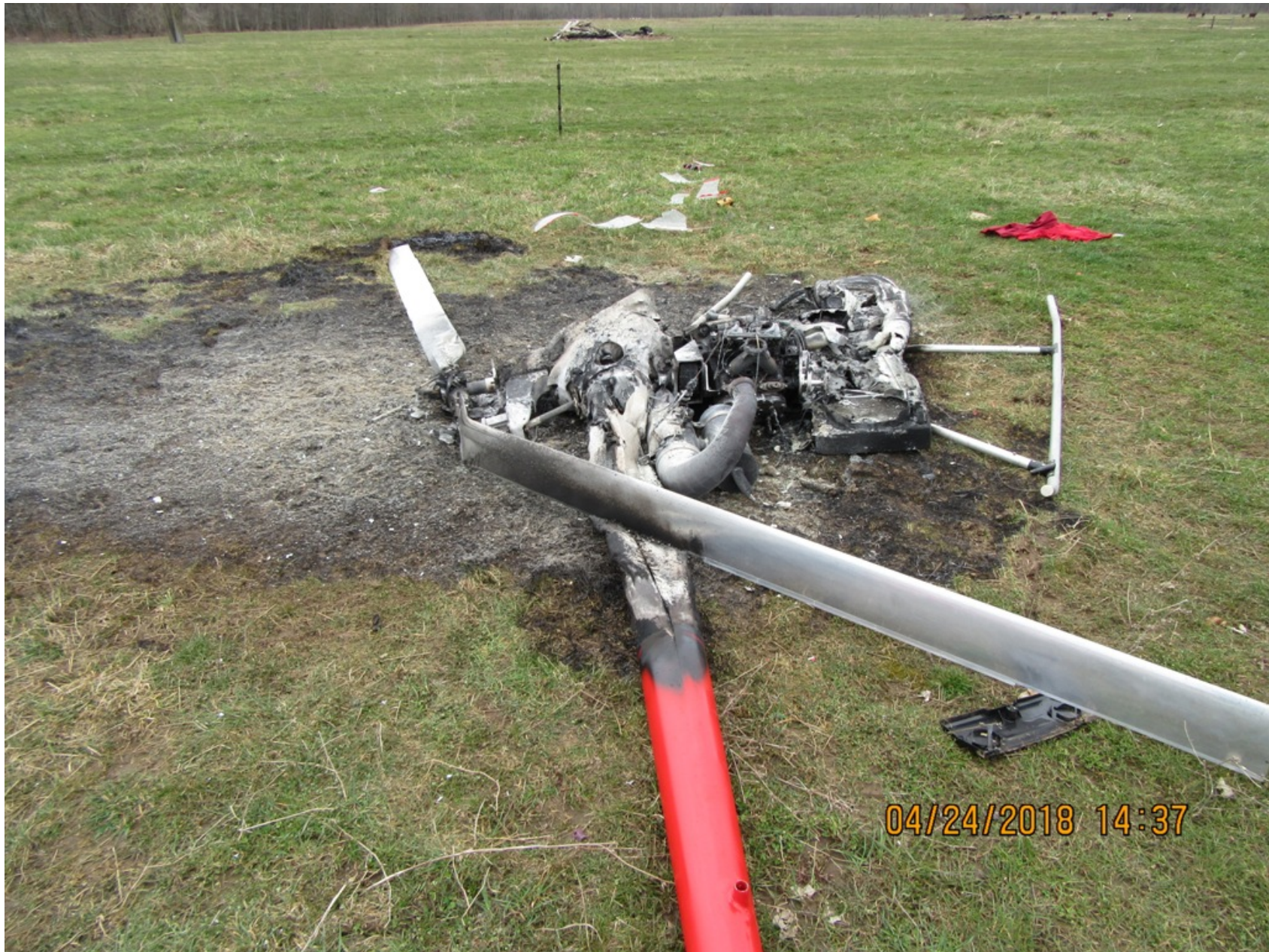
Photo 2 - FAA Digital Photograph. View of the Wreckage at the Accident Site. The Helicopter was Resting on Its Left Side. Note the Fire Damage to the Helicopter and Surrounding Area.
