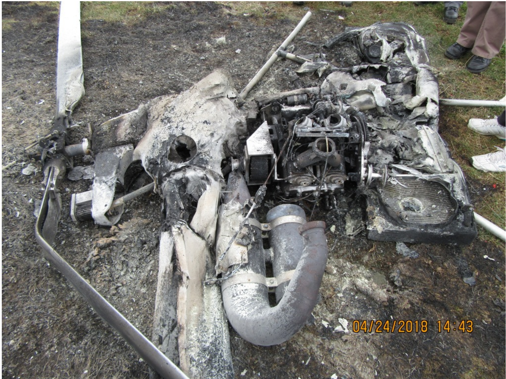
Photo 4 - FAA Digital Photograph. View of the Engine Assembly and Portion of Both Main Rotor Blades. Note the extensive fire damage to the Engine.
