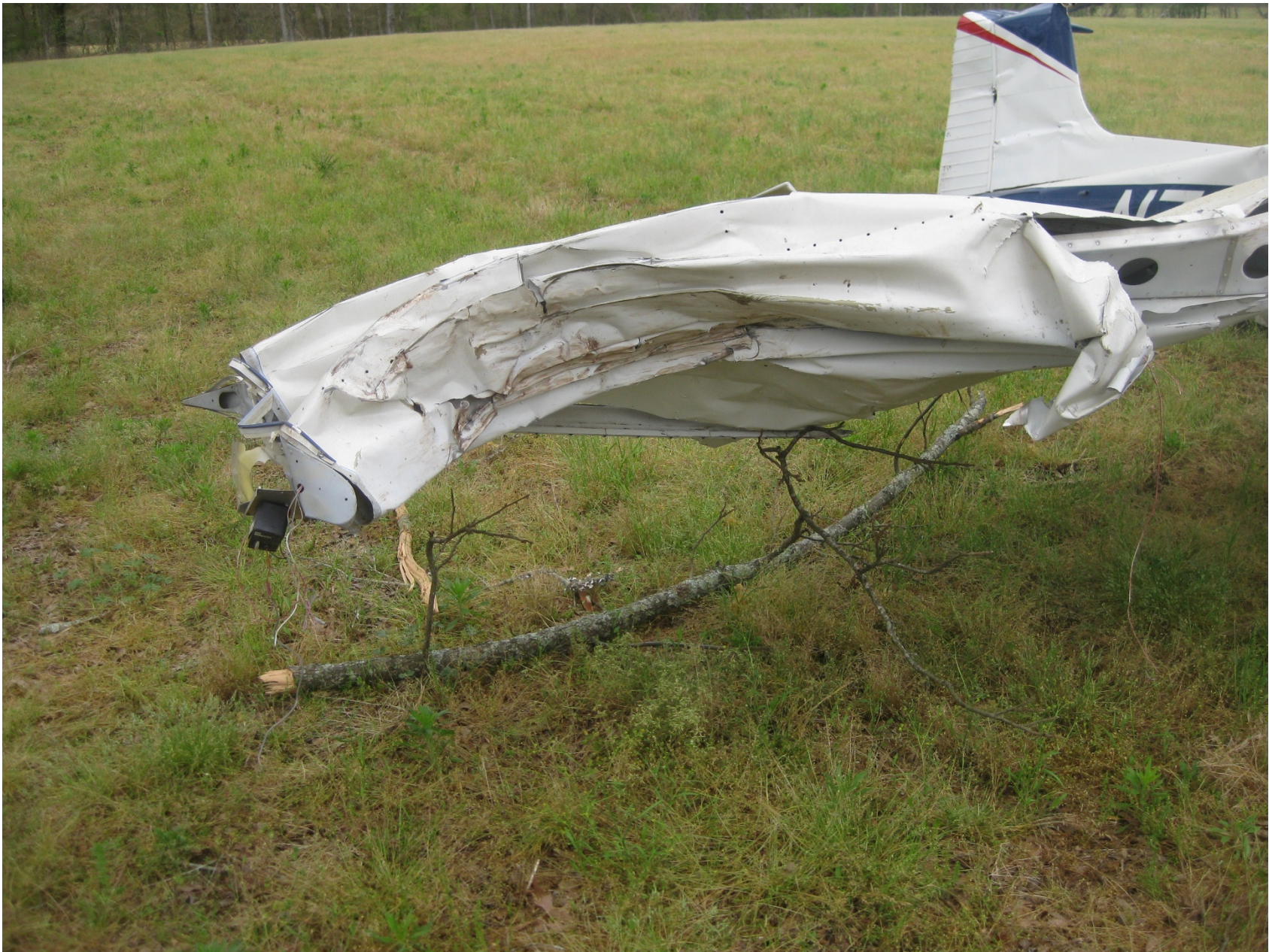
Photo 4 – View of right wing damage (Courtesy of FAA)
