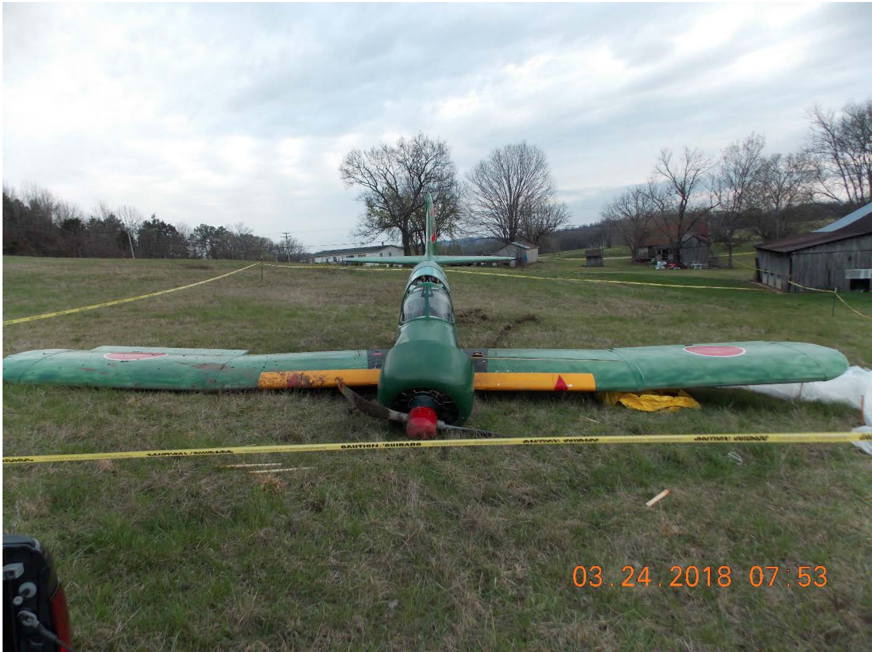
Photo 2 – View of front of airplane damage looking aft towards ground scars. (Courtesy of FAA)
