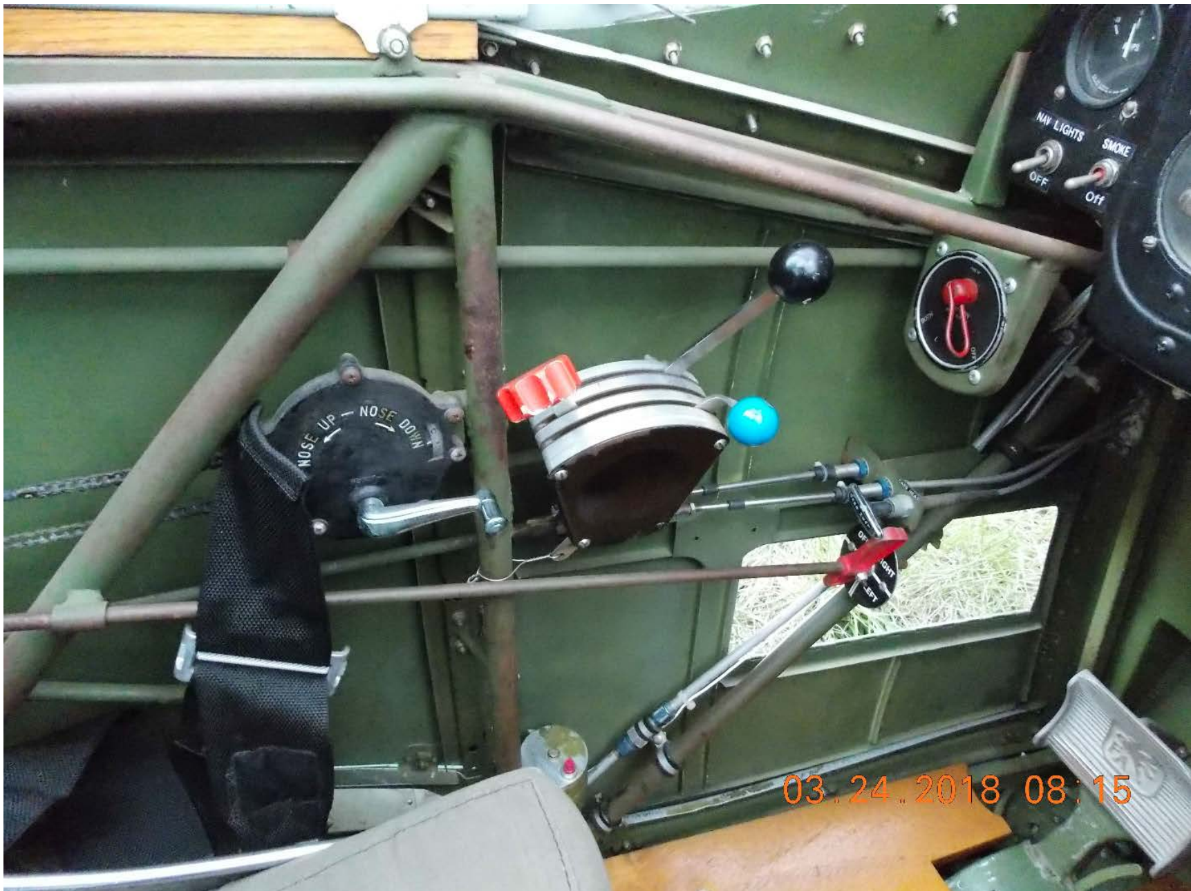
Photo 5 – View of left side of cockpit showing throttles and fuel selector handle. (Courtesy of FAA)
