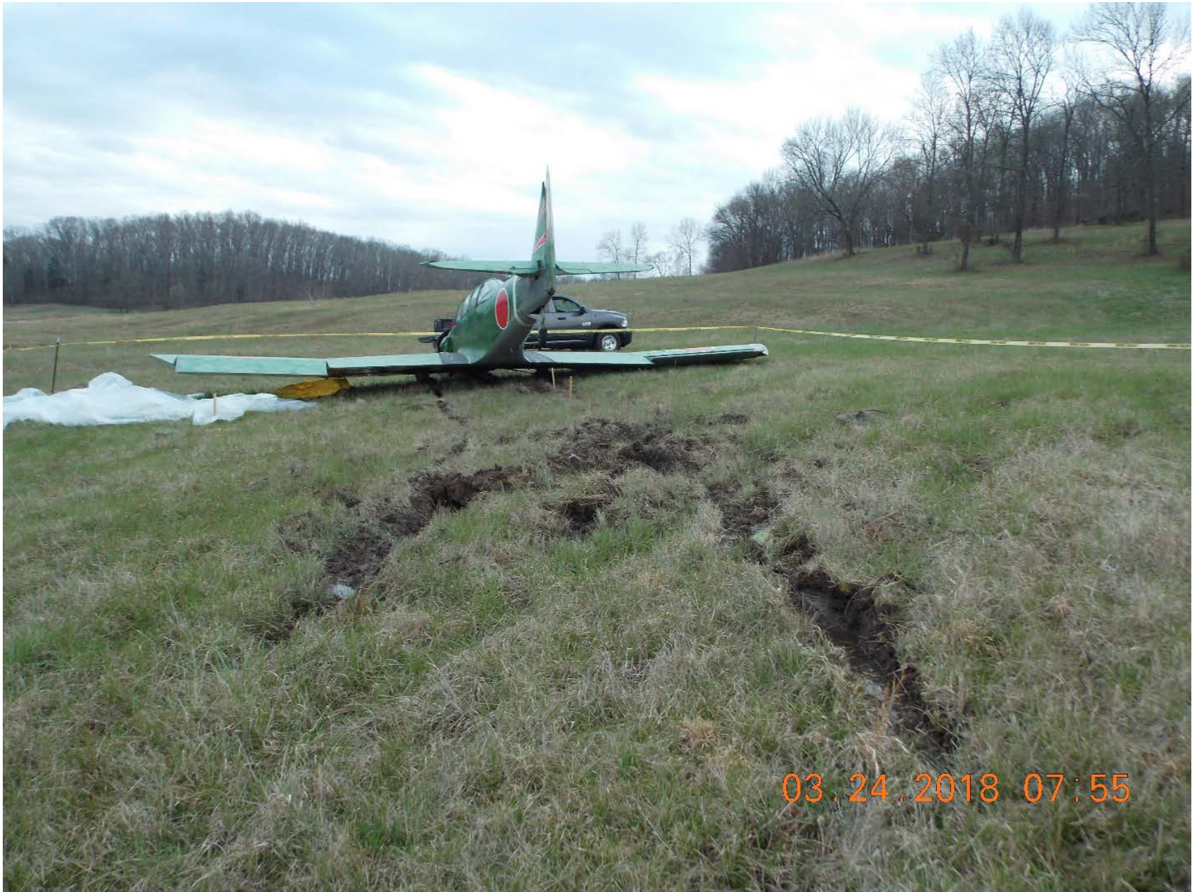
Photo 1 – View of ground scars leading to airplane. (Courtesy of FAA)
