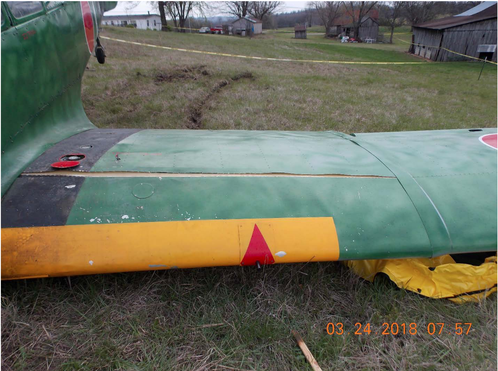
Photo 3 – Left fuel tank and wing damage. (Courtesy of FAA)
