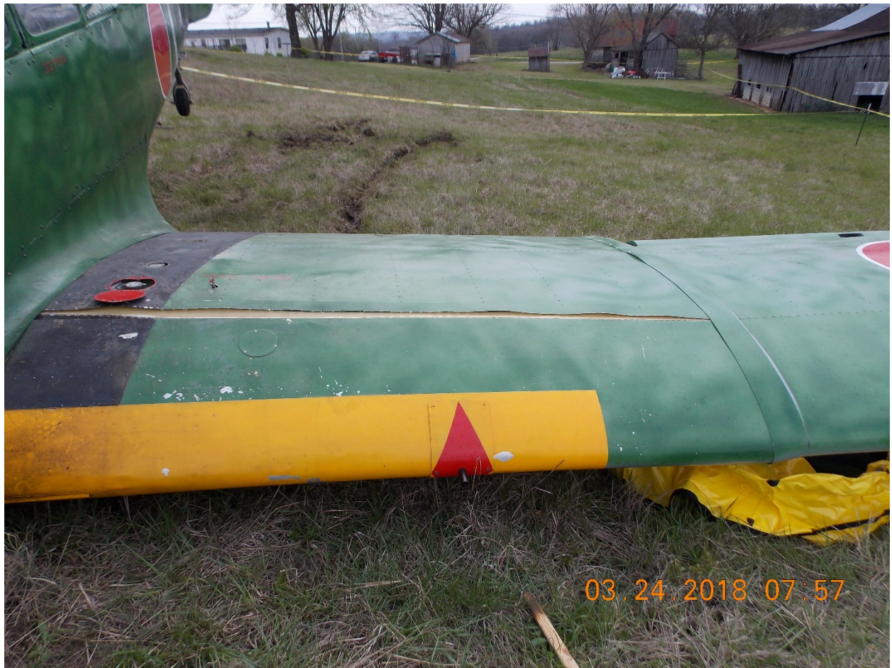
Left Wing fuel tank ruptured.
