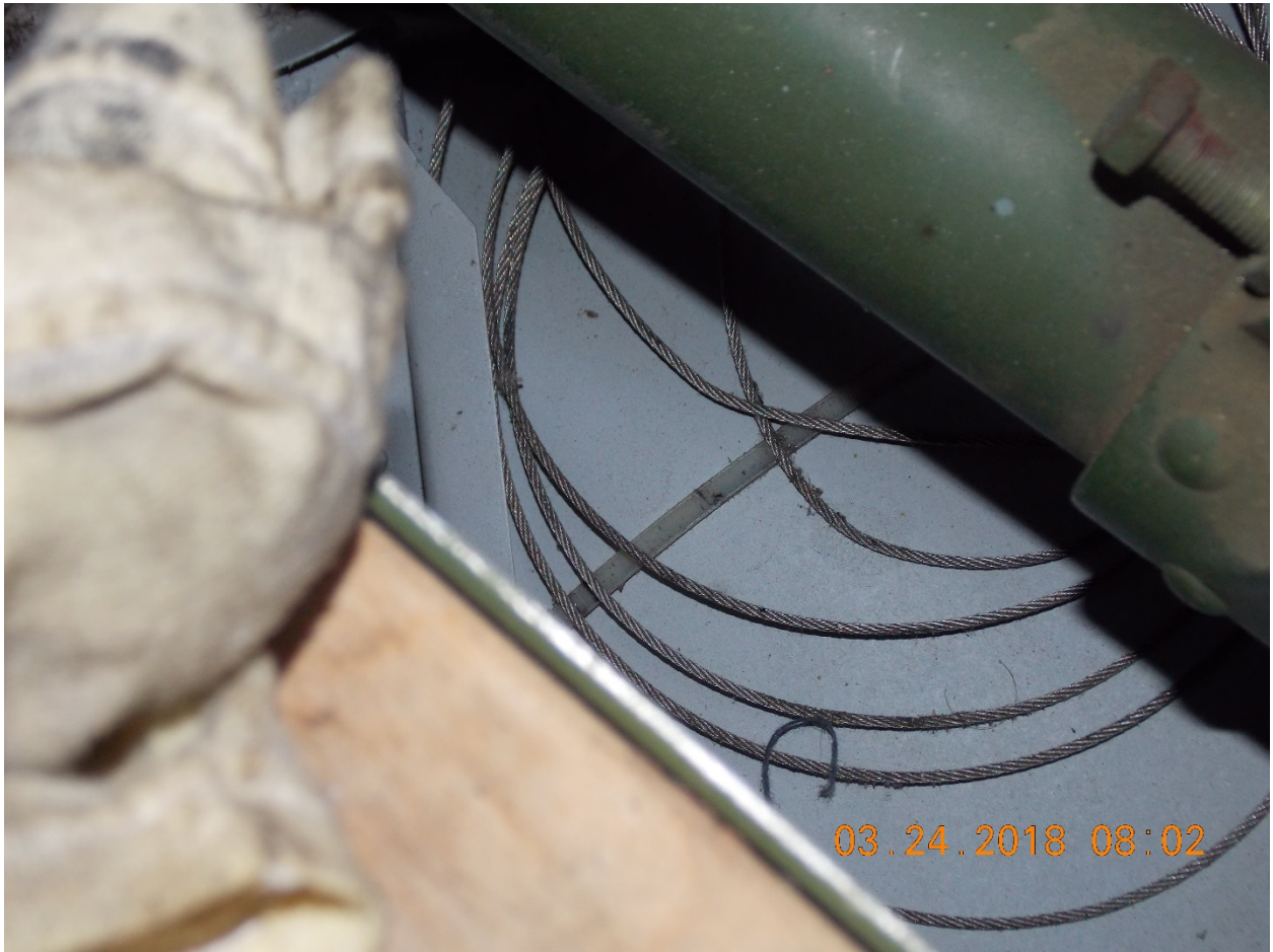
Coiled cable found under rear seat flight controls.
