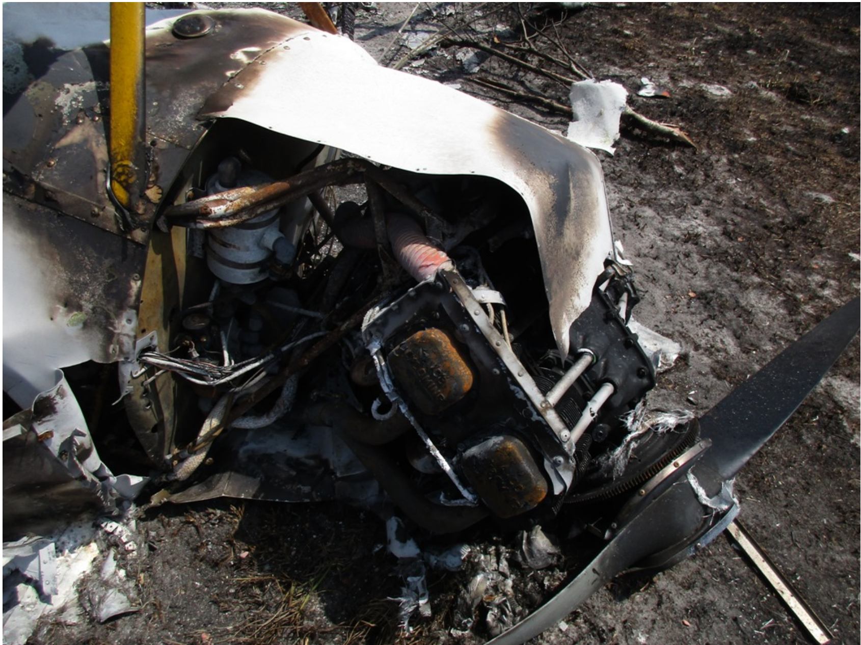
Photo 5 – Engine and Propeller (FAA Photo)
