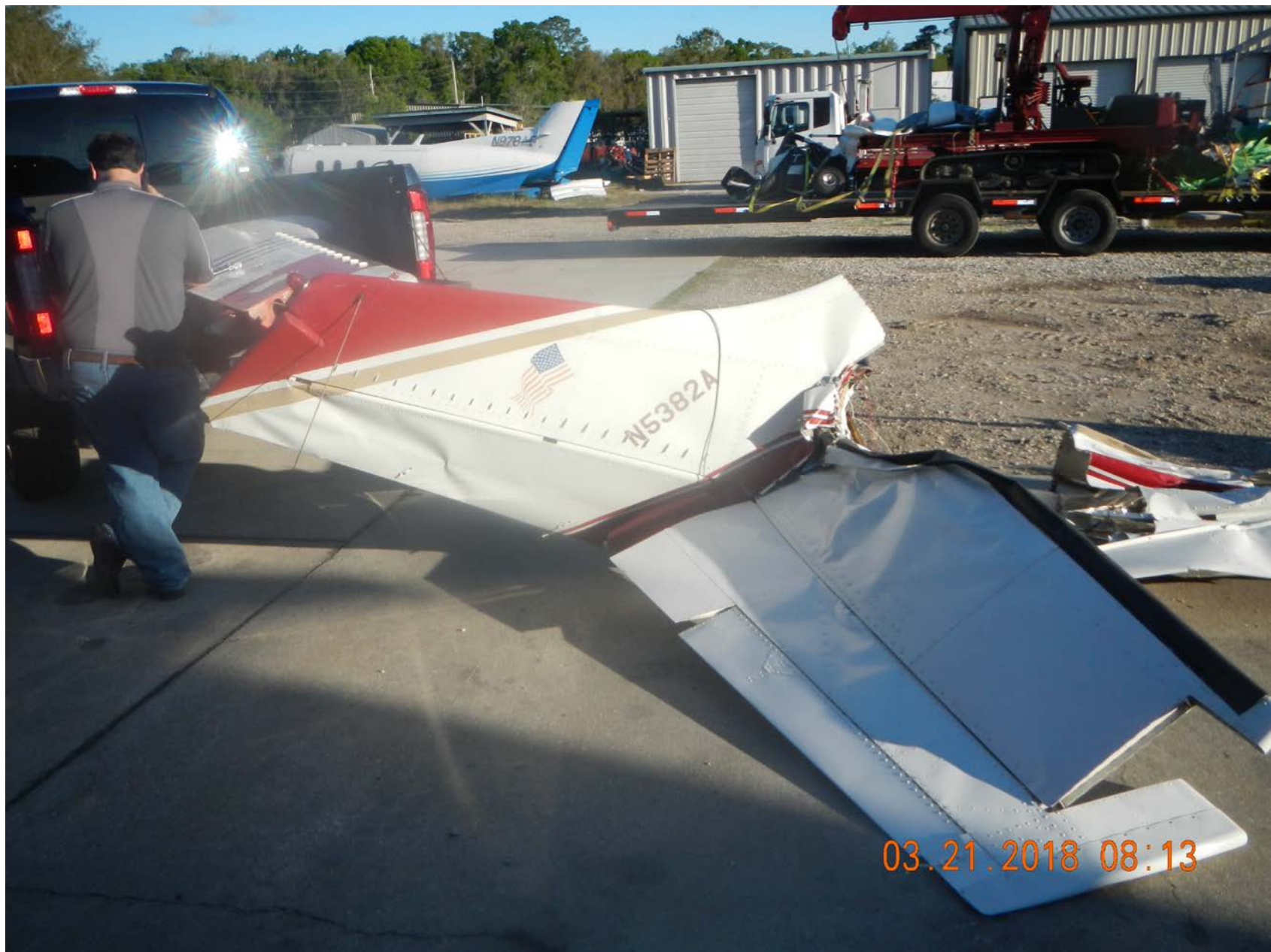
Photo 2 – View of separated empennage with buckling and crush damage on horizontal stabilizer
