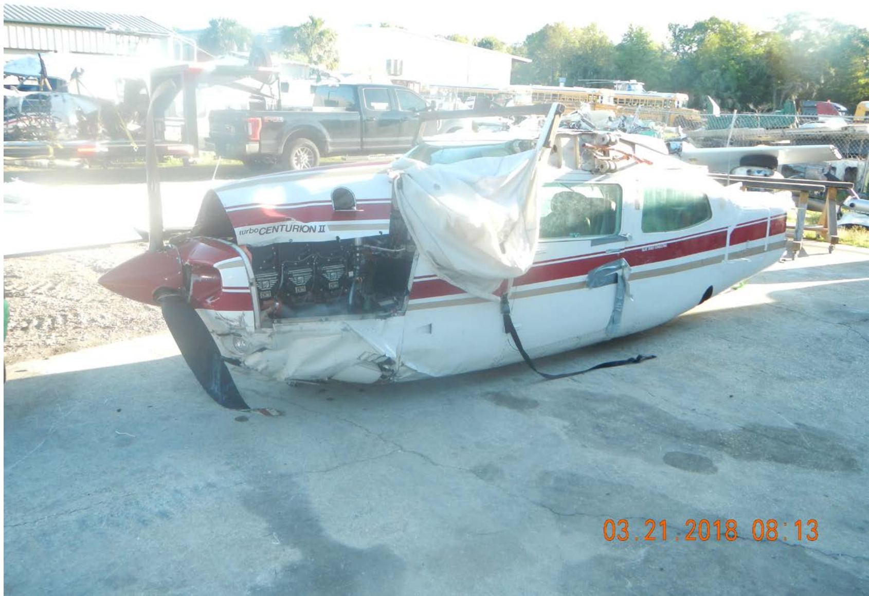
Photo 1 – View of fuselage showing crush damage
