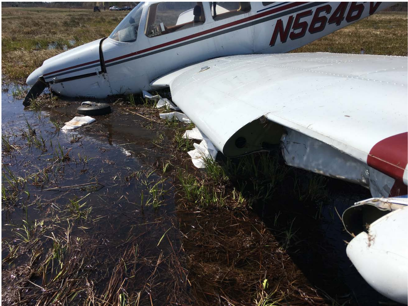
Photo 2 – View of Wing Leading Edge Damage (FAA)
