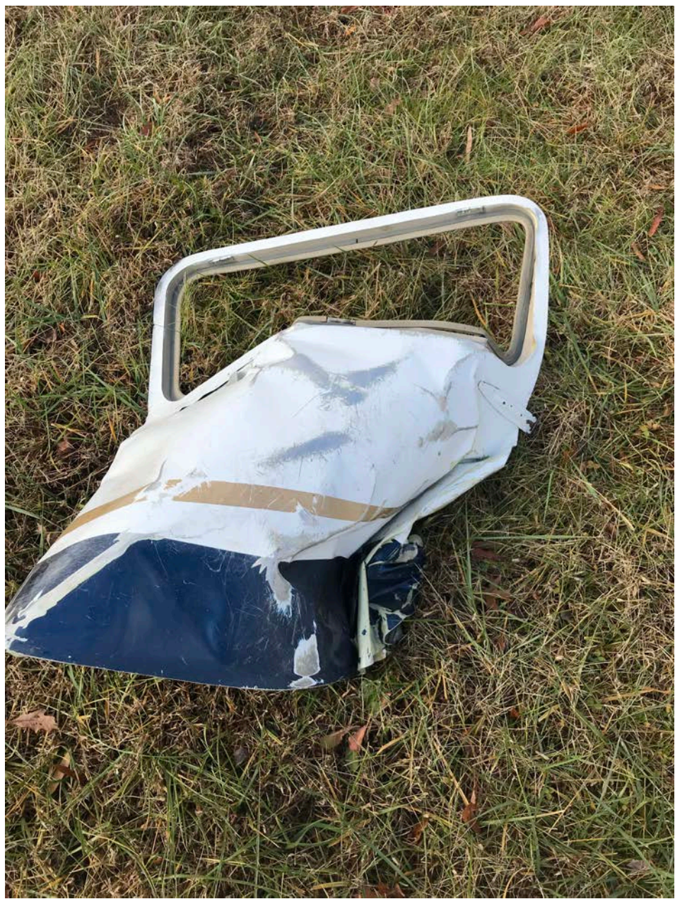
Photo 5 – View of recovered outer side of crush damaged passenger door
