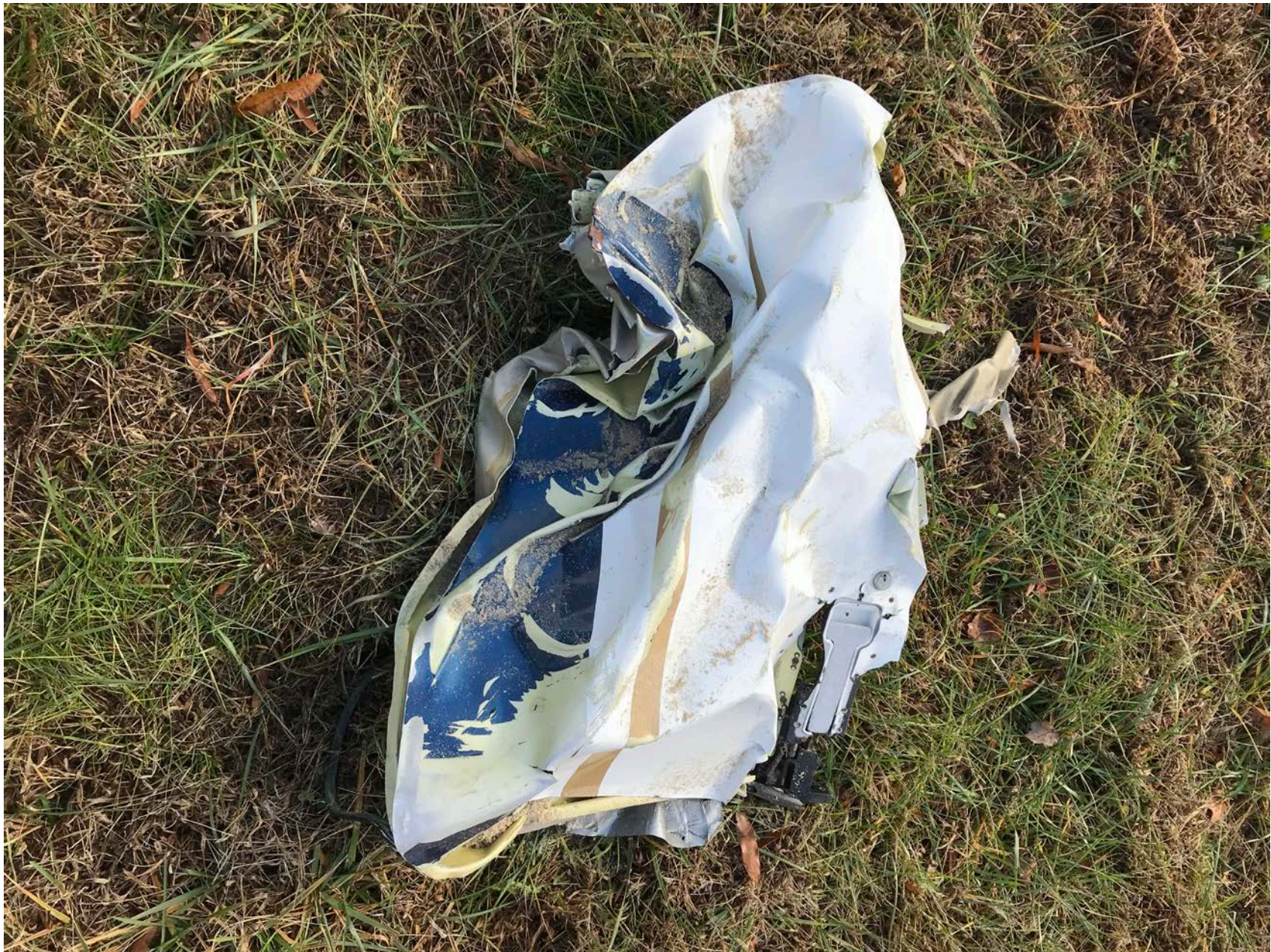
Photo 3 – View of recovered outer side of crush damage pilot's side door
