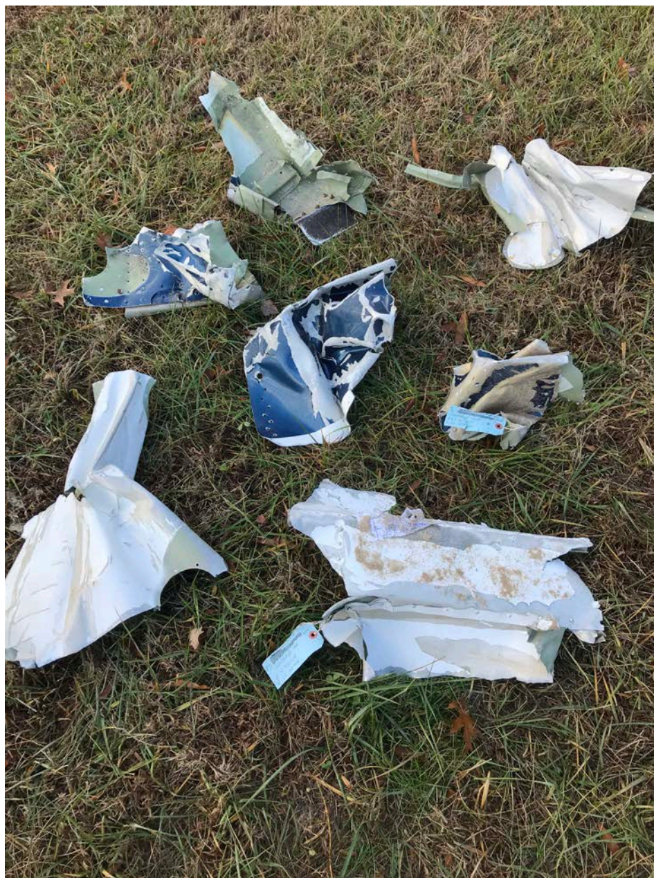
Photo 9 – View of recovered various fuselage skin pieces all showing crush damage
