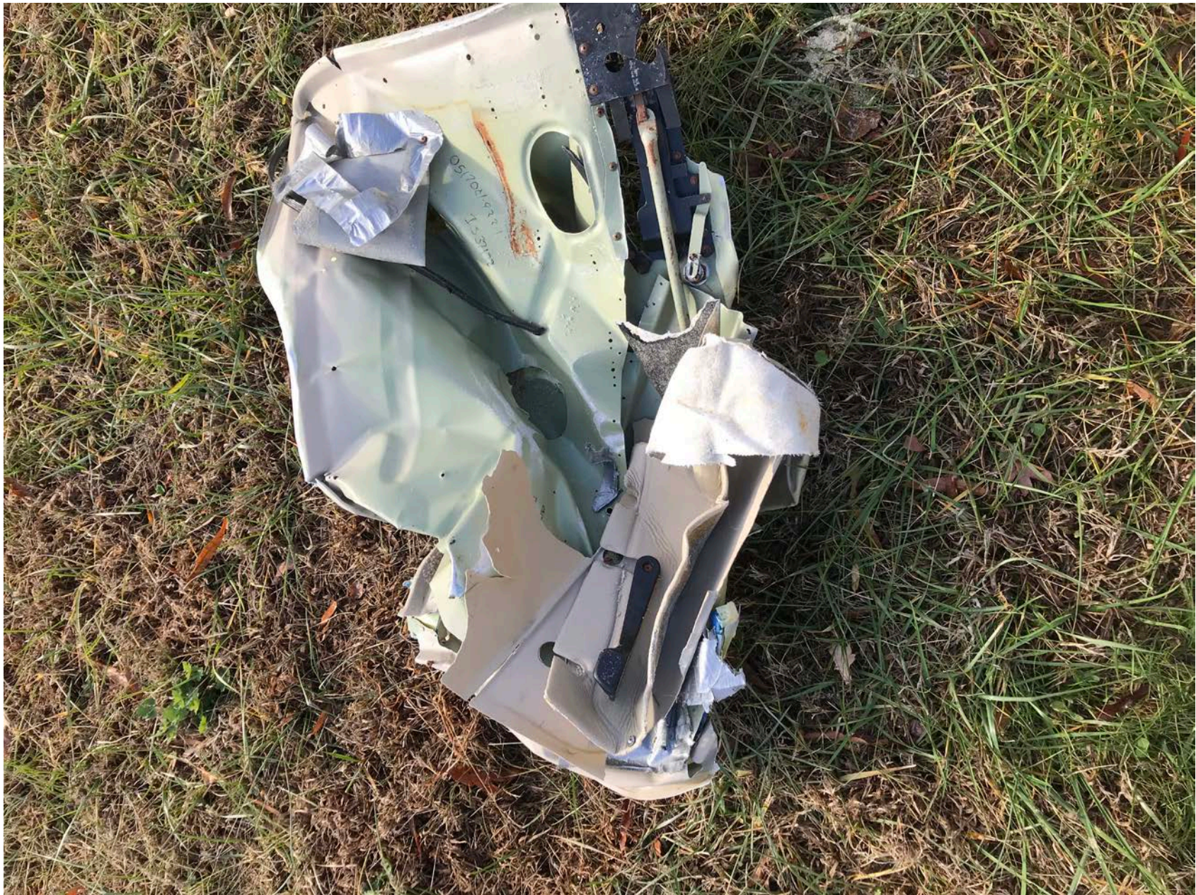
Photo 4 – View of inner side of recovered crush damaged pilot's door
