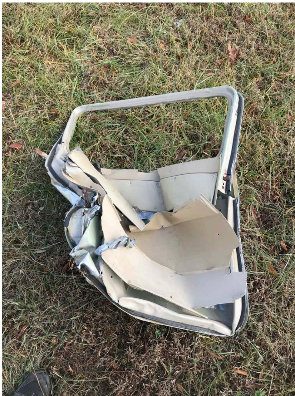
Photo 6 – View of inside of crush damage passenger door
