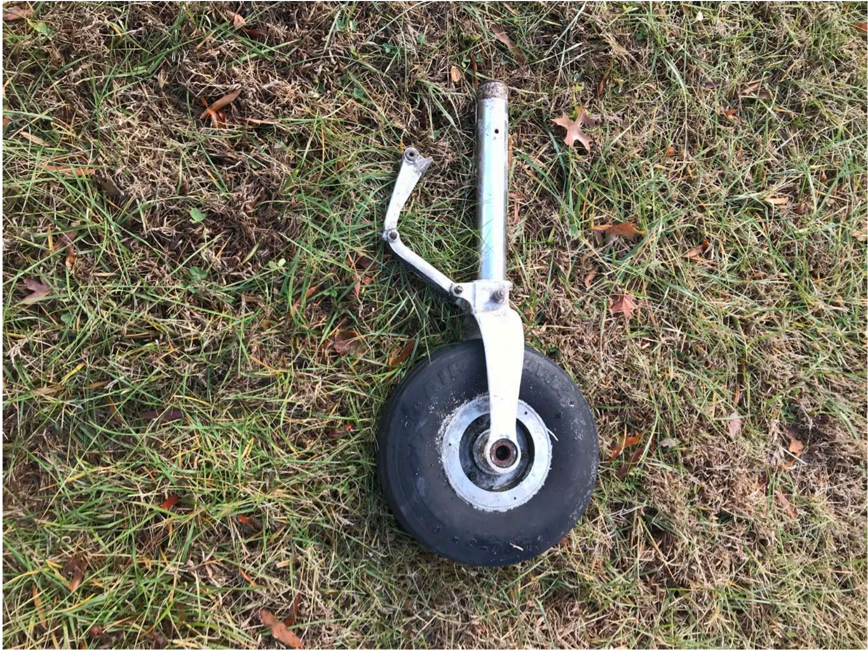
Photo 10 -View of recovered nose gear wheel attached to broken strut
