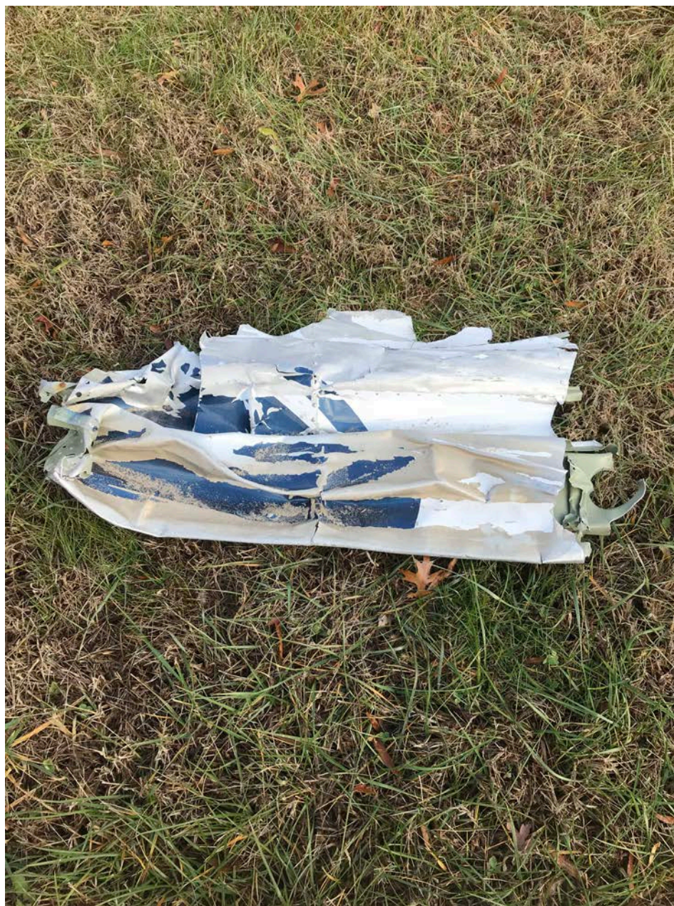
Photo 8 – View of recovered small part of leading edge of wing showing crush damage
