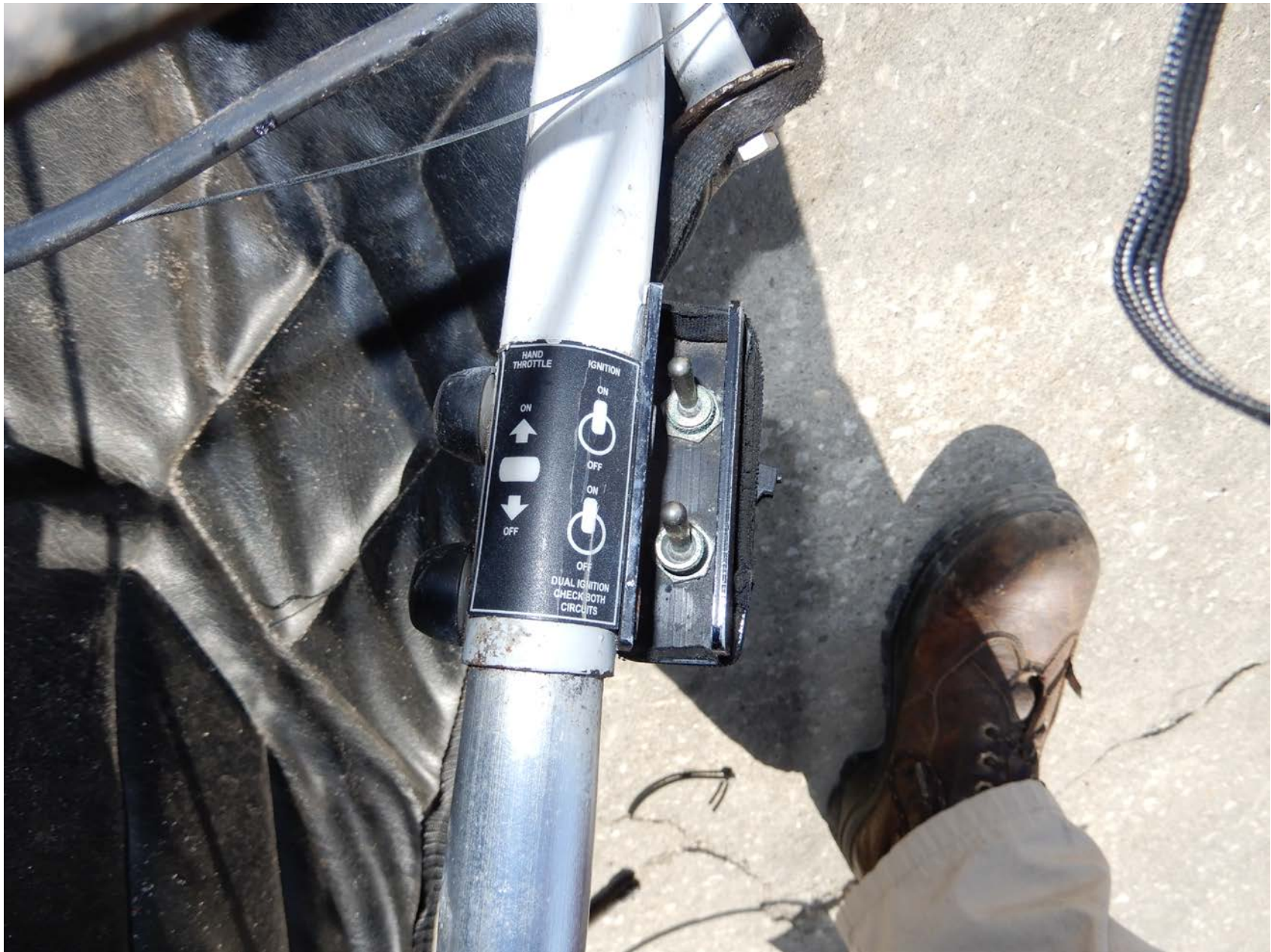
Photo 12 – Close Up of Ignition Switches
