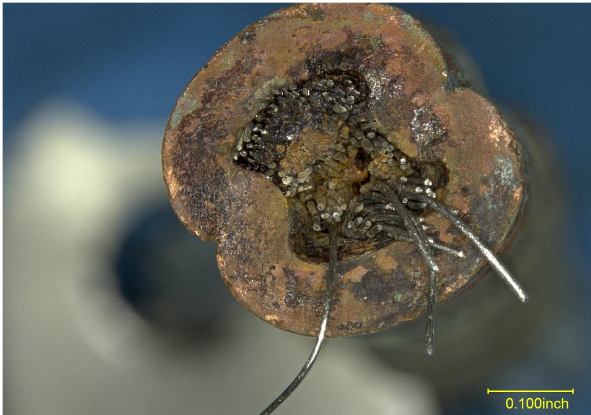
Figure 4 – View of the cable bundle fracture surface, after cleaning to remove corrosion.
