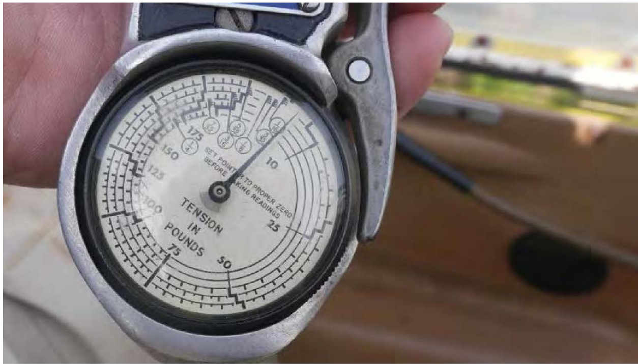
Figure 1: FAA Digital Photograph. View of the actual tensionometer reading that day during examination of the elevator flight control cable.
