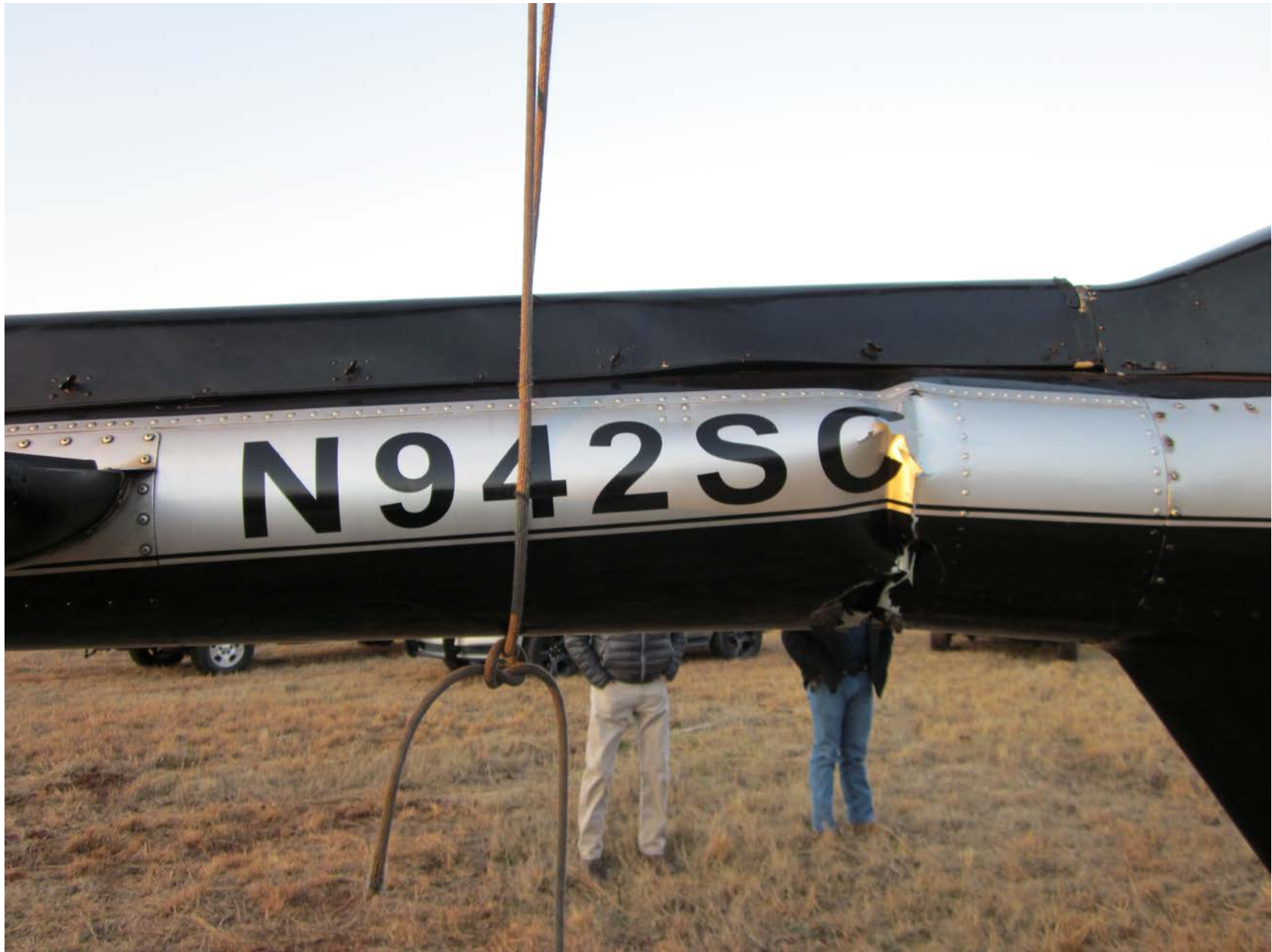
Photo 2 – View of Tailboom Deformation (FAA)
