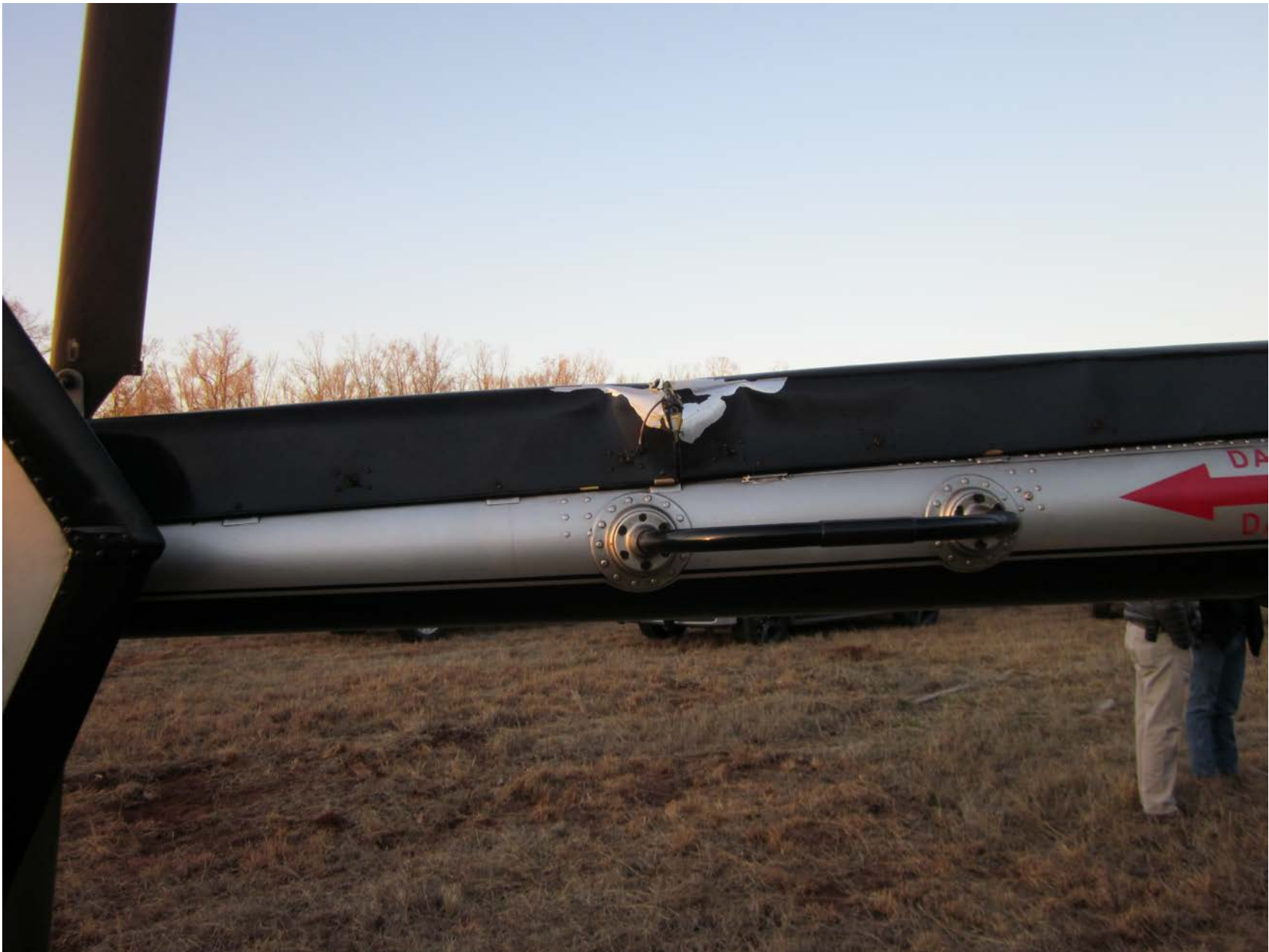
Photo 3 – View of Tailrotor Driveshaft Cover Damage (FAA)
