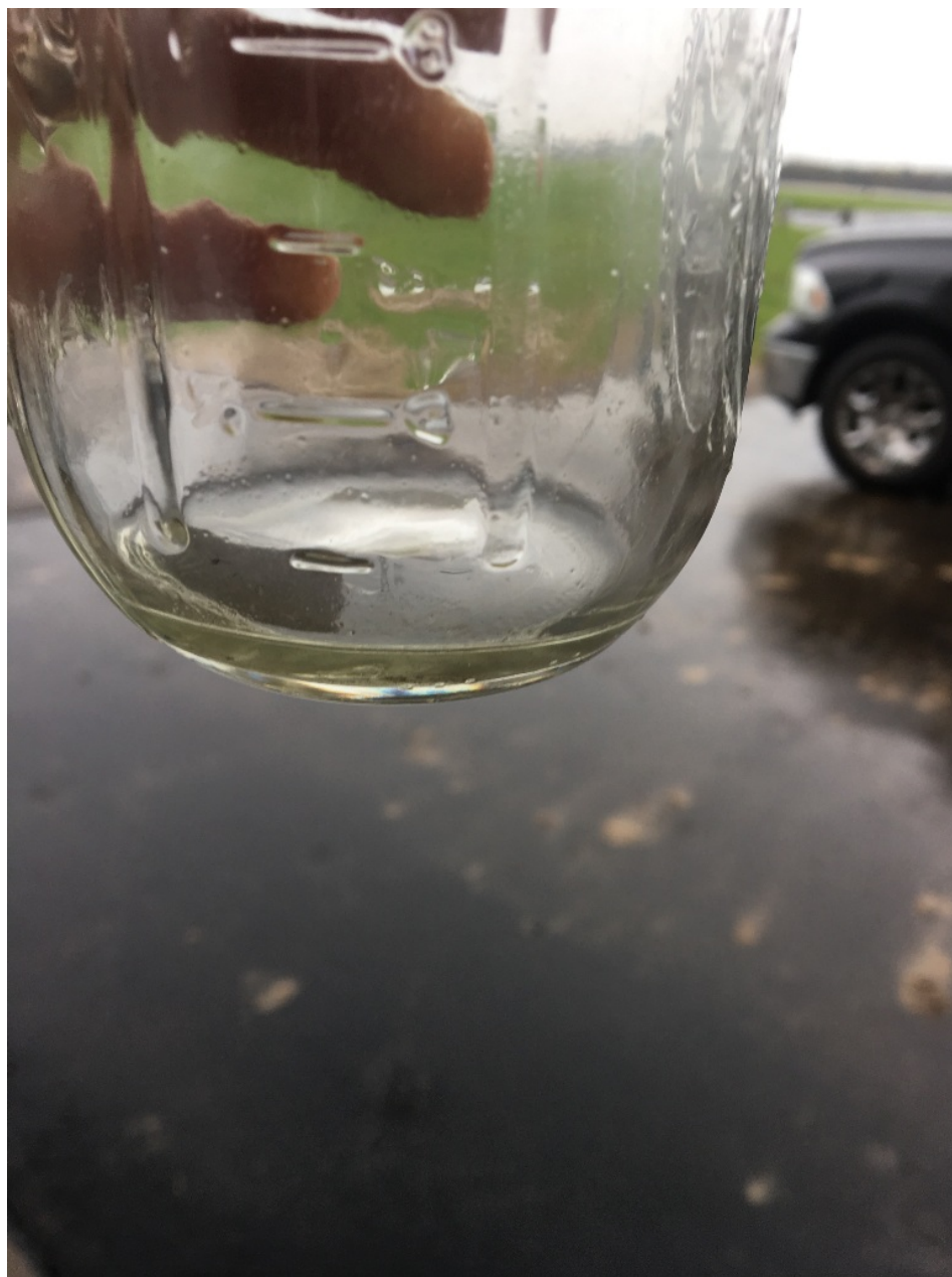
Photo 3 – Fuel Found in the Main Fuel Line From the Electric Boost Pump to the Fuel Controller
