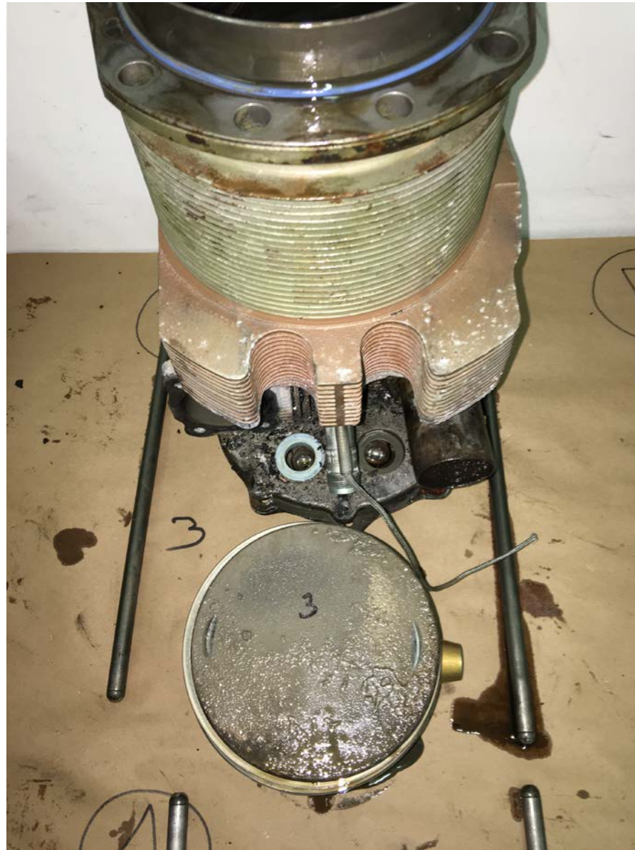
Photo 10 – Number 3 cylinder assembly showing piston valve impact damage.
