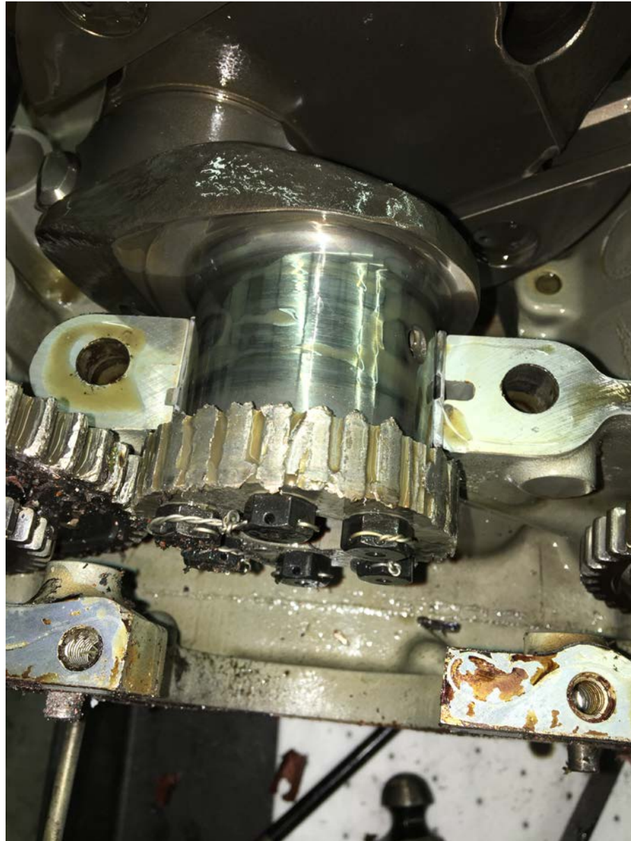
Photo 11 – Crankshaft gear damage after engine case disassembly.
