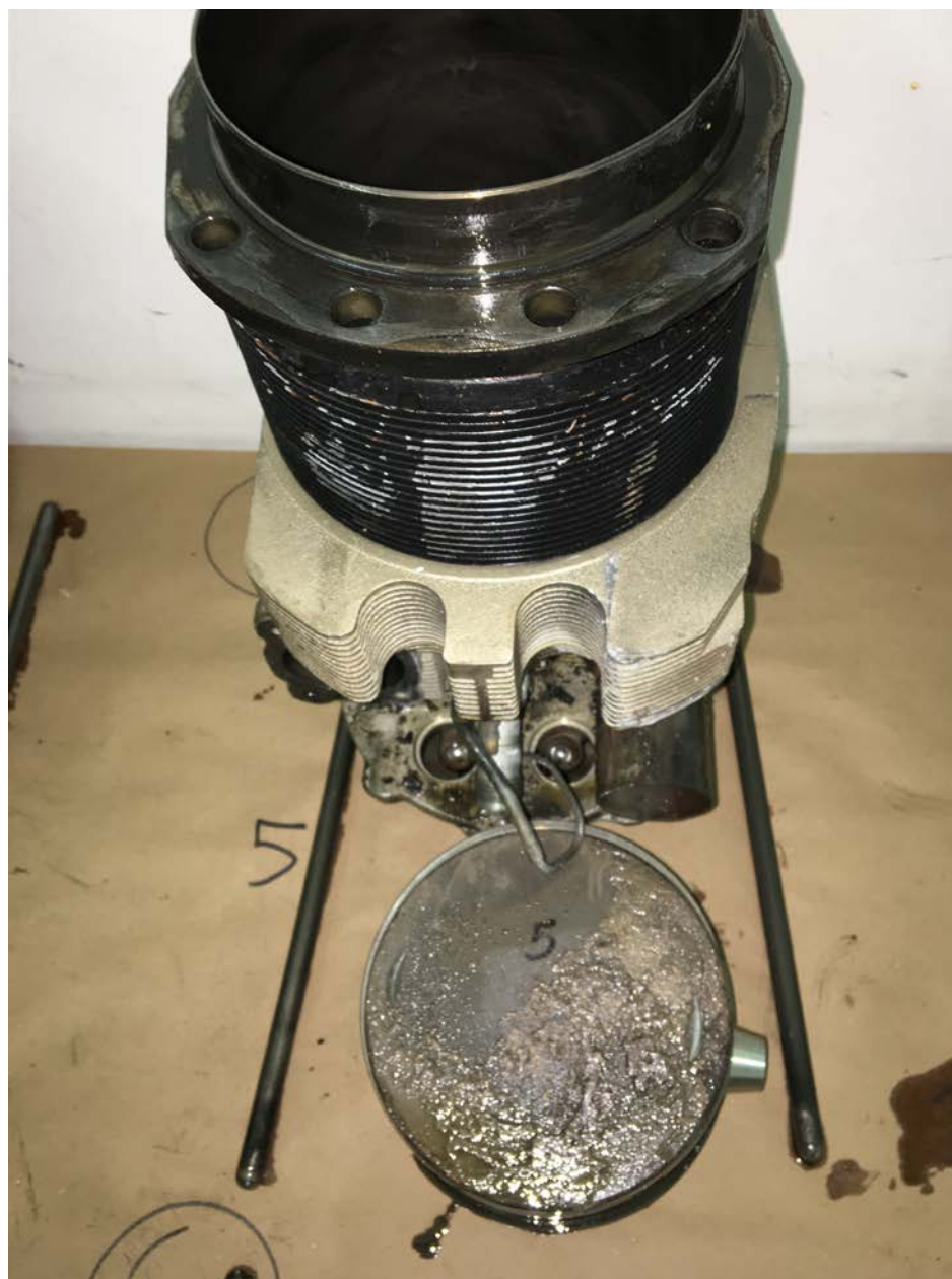
Photo 9 – Number 5 cylinder assembly showing piston valve impact damage.
