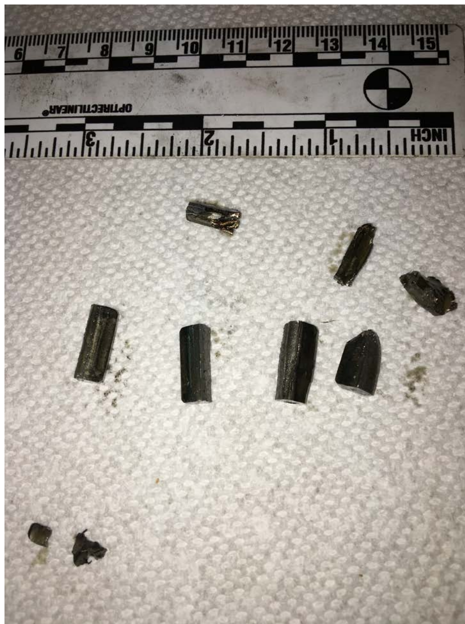
Photo 8 – View of gear teeth with ruler for scale.
