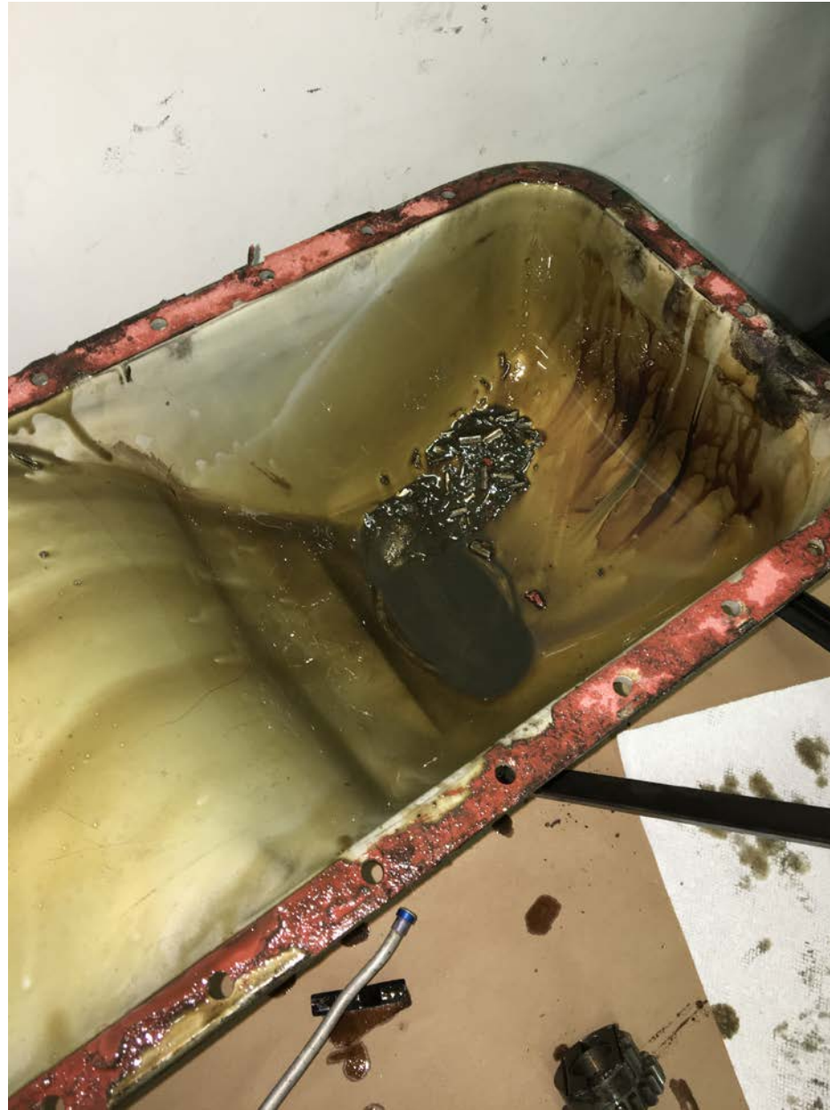
Photo 7 – View of metal and gear teeth in oil sump.
