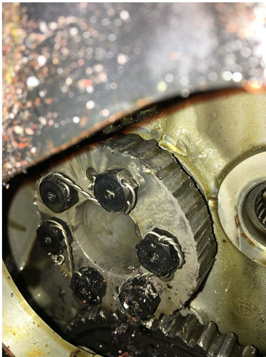
Photo 6 – View of damaged crankshaft drive gear through engine accessory section.
