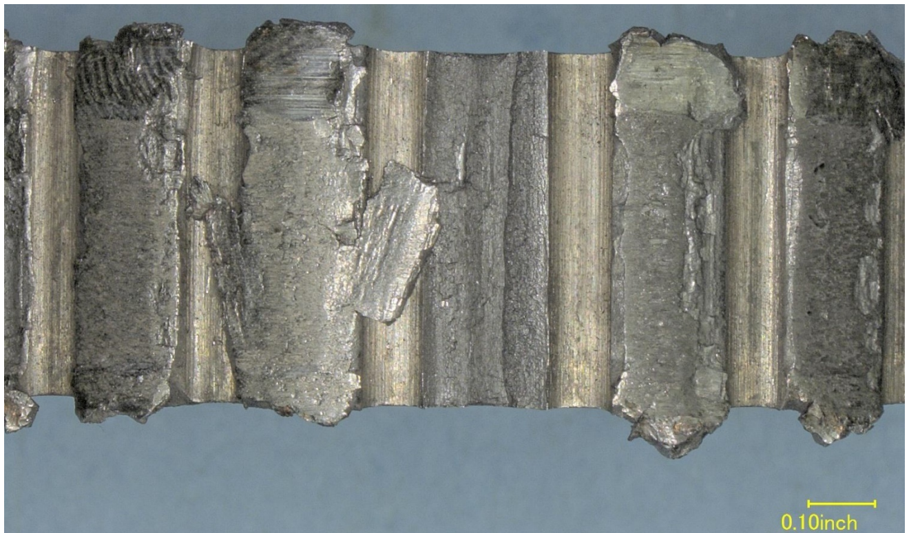
Figure 20 – View of the fractured gear tooth in Figure 14, located 180° opposite of the fractured teeth in Figure 15.
