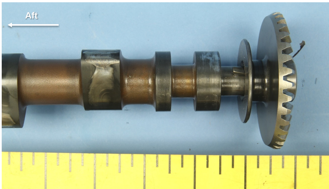
Figure 11 – Some of the journal bearings and lobes of the forwardmost part of the camshaft, including the governor bevel gear.
