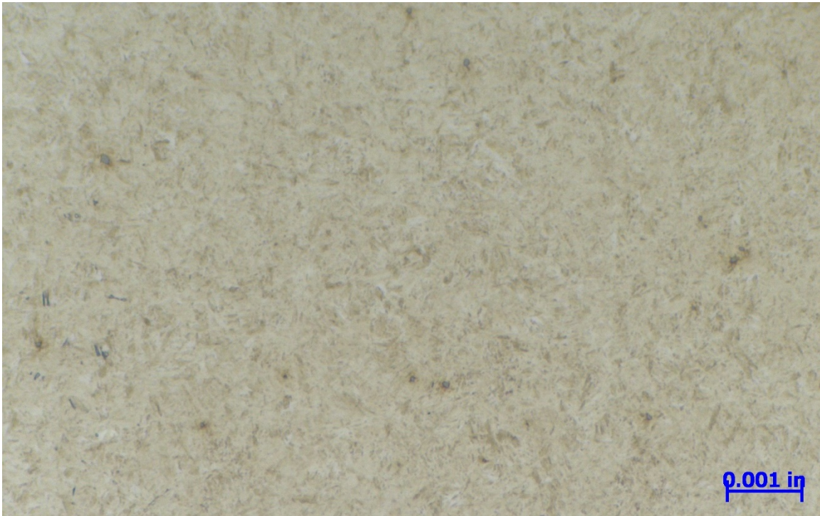
Figure 25 – BF optical micrograph showing a typical area of the surface microstructure showing high carbon phases (~500X, etched 2% Nital).
