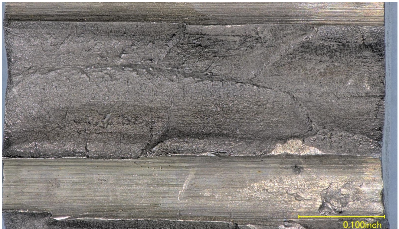
Figure 16 – Closer view of the fractured tooth exhibiting progressive cracking, later determined to be fatigue.
