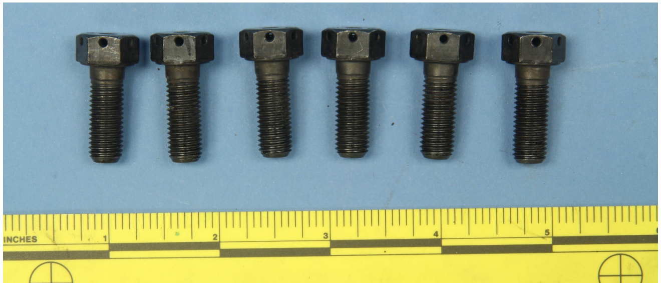
Figure 4 – The loose six attachment bolts, after cleaning to remove oils and particles.
