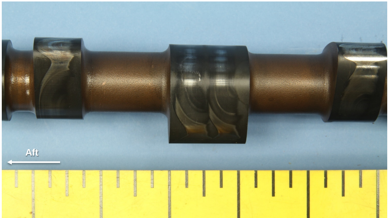
Figure 10 – Some of the journal bearings and lobes of the camshaft, viewed forward of the position in Figure 9.
