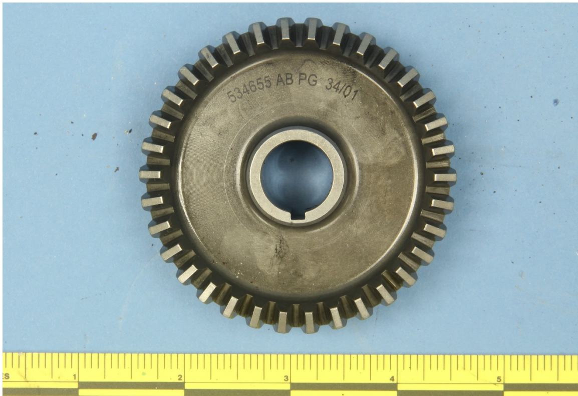
Figure 12 – The bevel gear from the forward side of the camshaft assembly, after removal from the camshaft.
