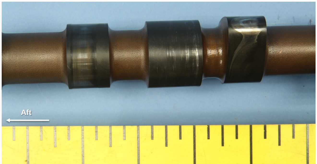
Figure 9 – Some of the journal bearings and lobes of the camshaft, viewed forward of the position in Figure 8.
