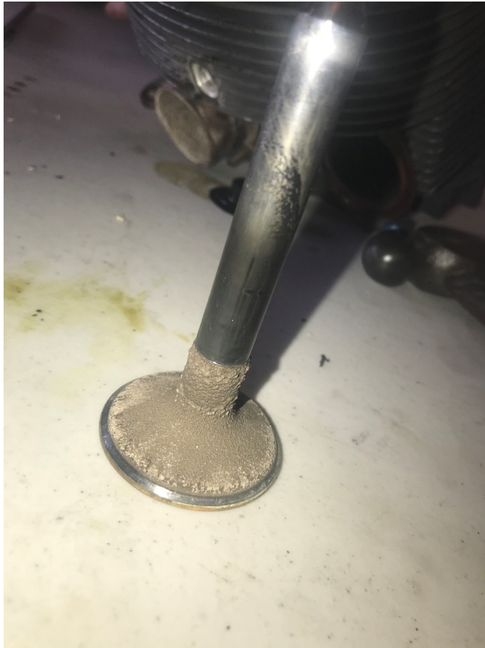
Photo 2 - Intake Valve from the No. 4 Cylinder (Photo Courtesy of FAA)
