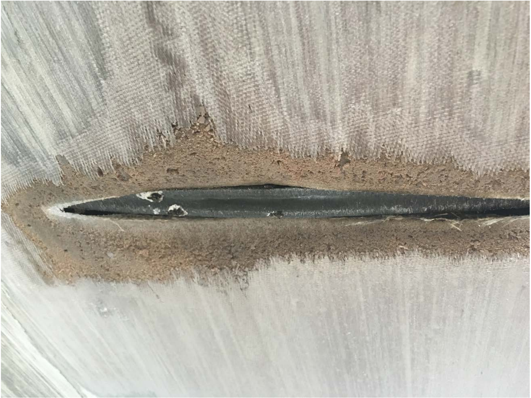
Photo 2 – Damage to the belly of the airplane. (Photo courtesy of the FAA)
