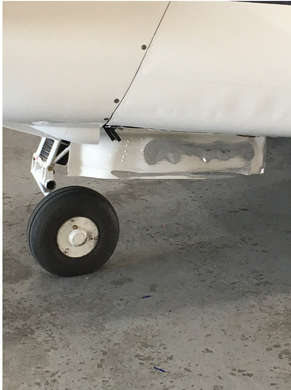
Photo 1 – Damage to nose gear door. (Photo courtesy of the FAA)
