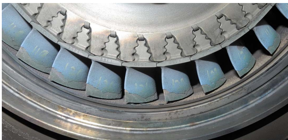
Figure 12. Damage to the first stage gas generator turbine blades.
