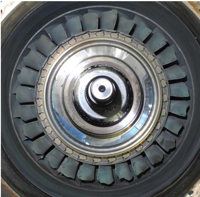
Figure 10. The No. 2 engine second stage gas generator turbine blades exhibiting missing tips.
