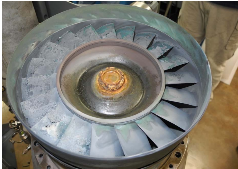
Figure 7. Damage observed on the turbine inlet stator vanes for the No. 2 engine.
