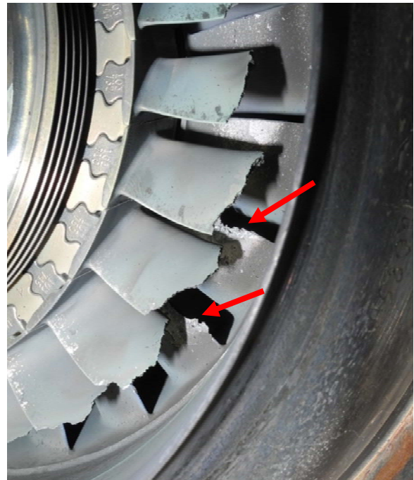
Figure 11. A close up showing partial melting of the second stage nozzle guide vanes for the No. 2 engine.
