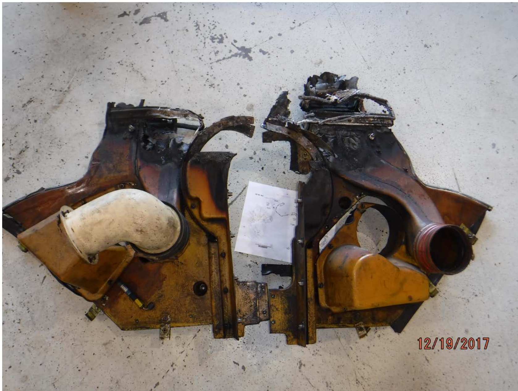
Photo 16 – Aft View of Oil Cooler Assembly. Note Soot and Thermal damage. (Courtesy of Sikorsky)
