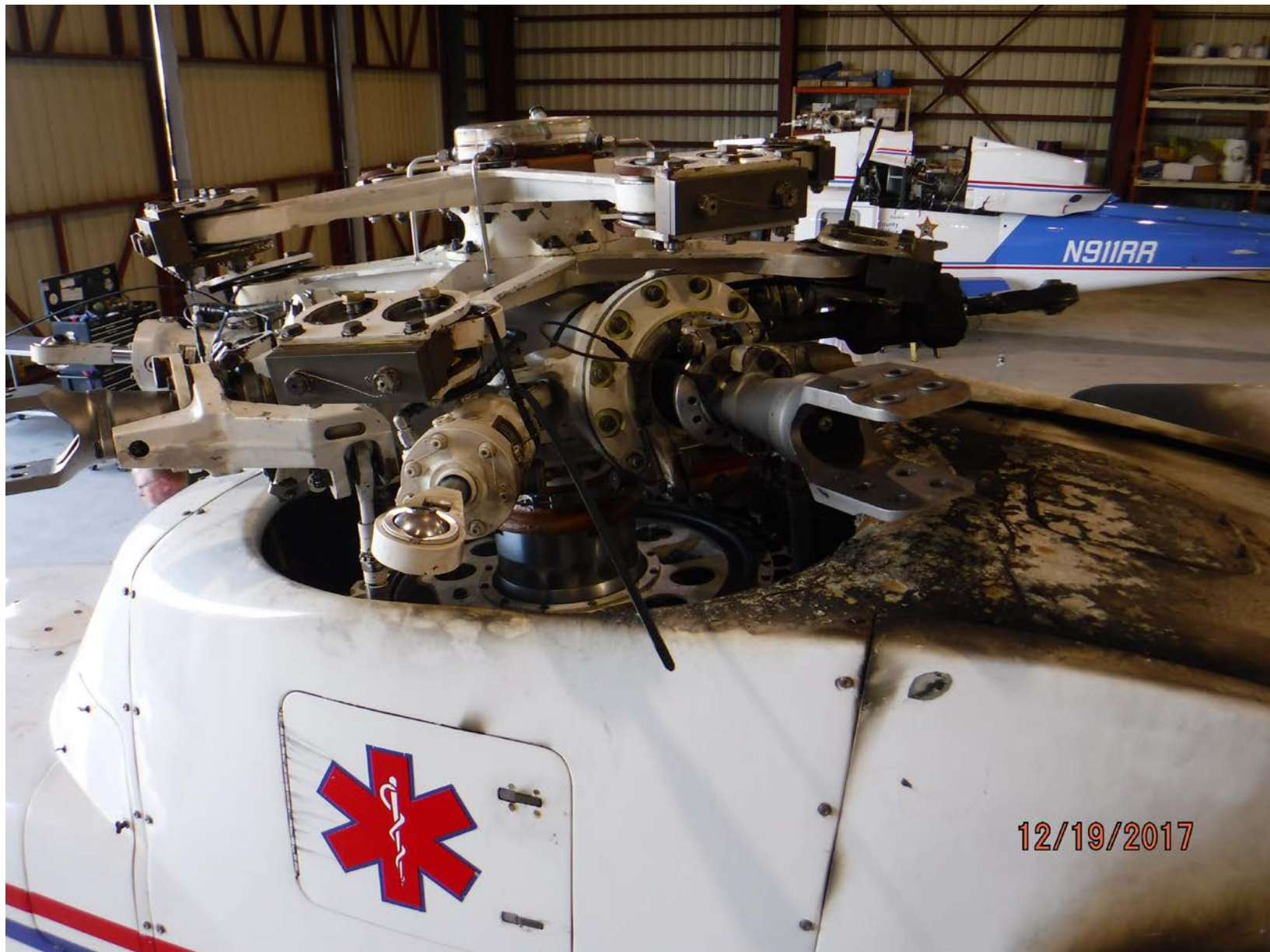
Photo 4 – Top View of Rotor Head and Engine Cowl Thermal Damage. (Courtesy of Sikorsky)
