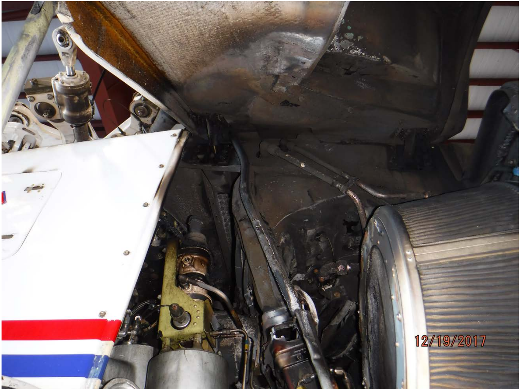
Photo 15 – Number 1 Engine Intake Area Soot and Heat Damage. (Courtesy of Sikorsky)
