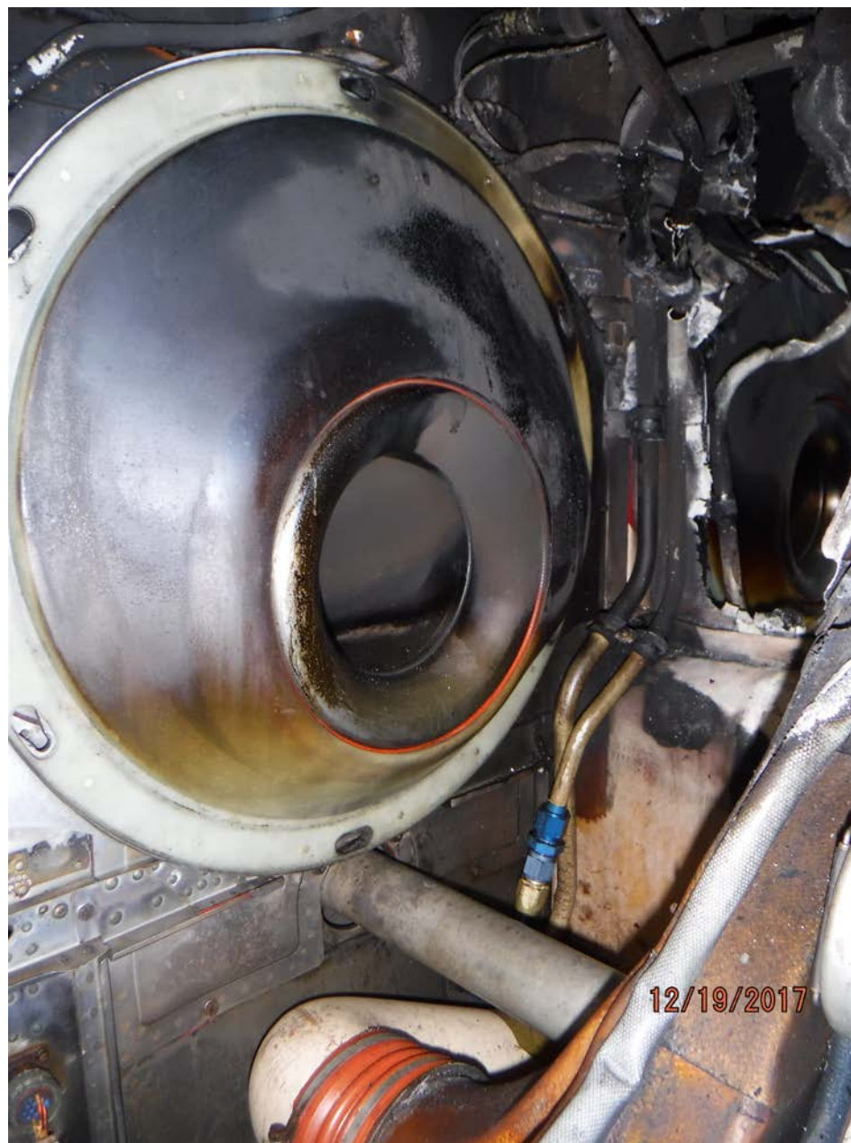
Photo 13 – Number 2 Engine Intake with Barrier Filter Removed. (Courtesy of Sikorsky)
