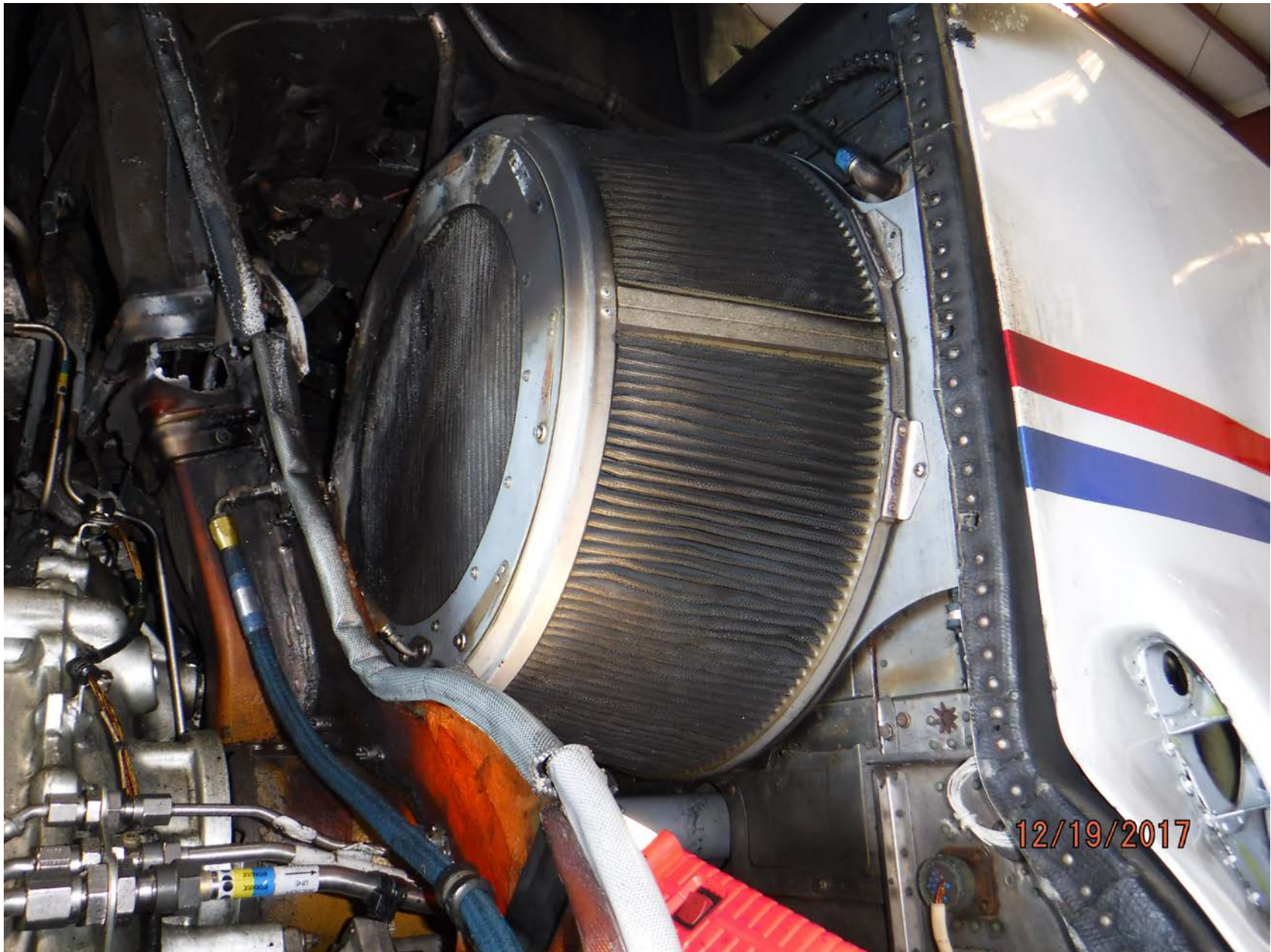
Photo 14 – Number 1 Barrier Filter Installed. Note Soot and Heat Damage. (Courtesy of Sikorsky)
