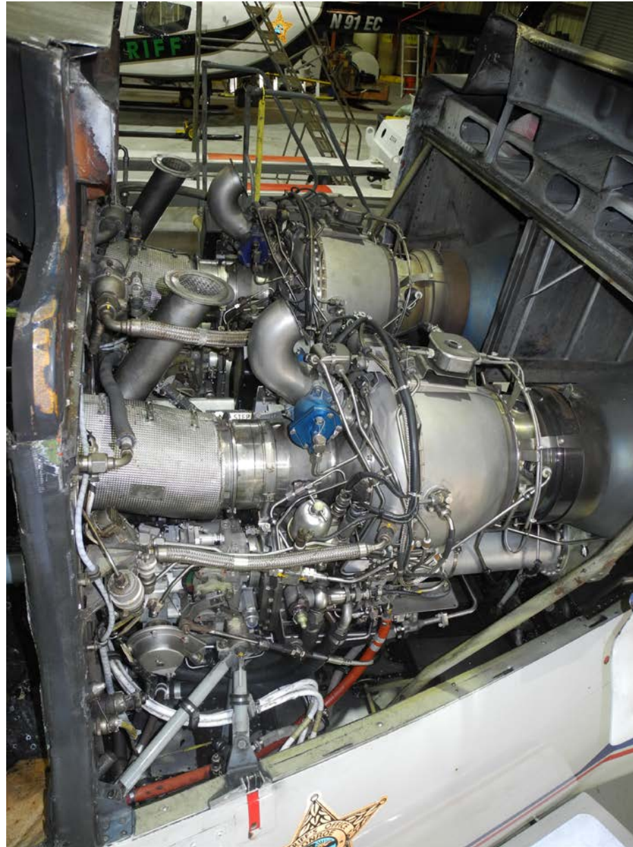
Photo 19 – View of Engine Exterior Condition. Left Engine in Foreground.
