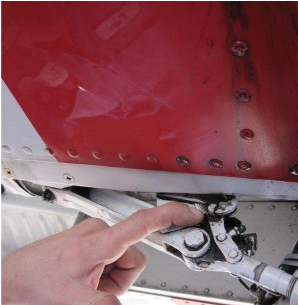
Photo 4 – Left Main Landing Gear Drag Link (FAA Photo)
