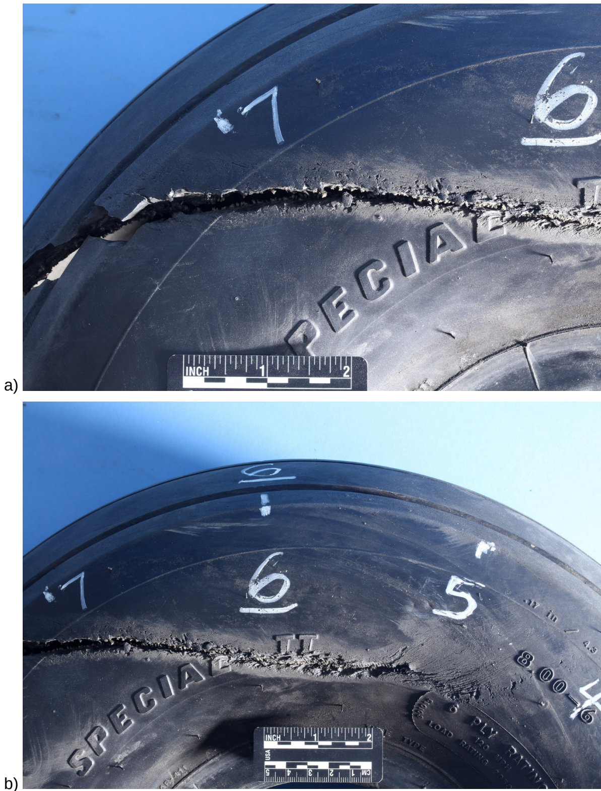
Figure 4: a) and b) Images of the fracture along the NSS starting near the 7:30 position and ending near the 5 o'clock position.
