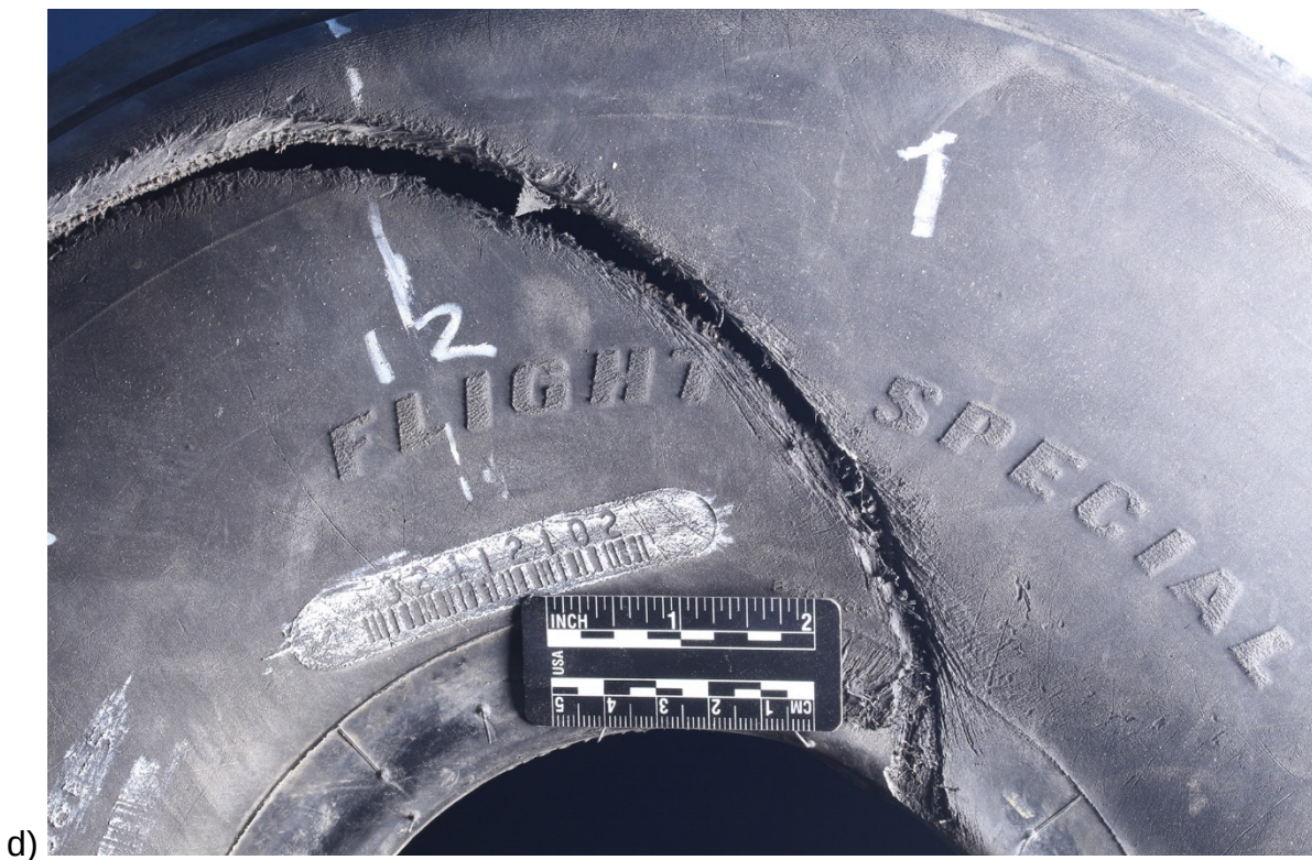
Figure 5 (cont.): c) between 11 o'clock and 12 o'clock; and d) between 12 o'clock and 1 o'clock where the fracture diverted into the sidewall.
