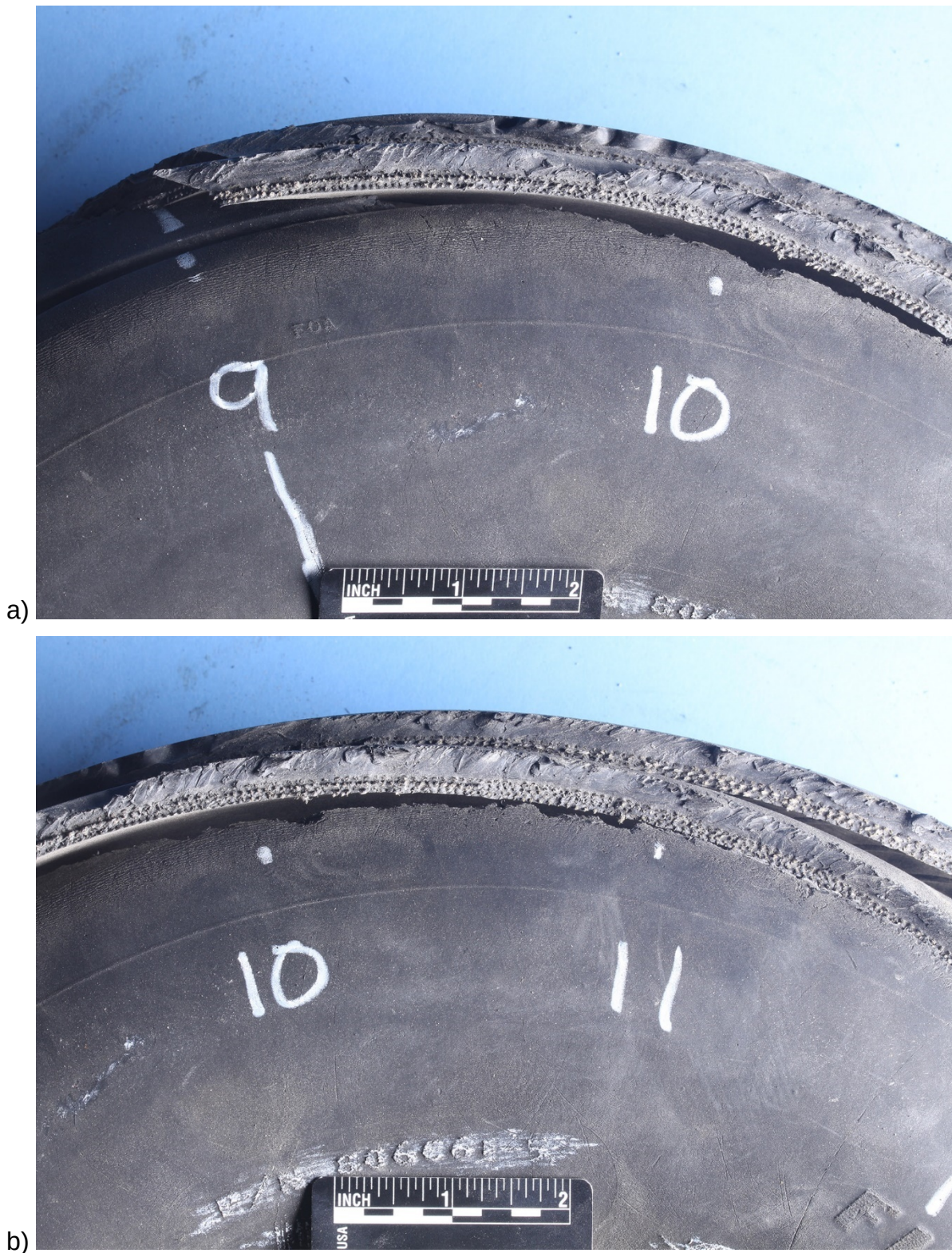
Figure 3: Images of the fracture along the SS shoulder: a) between 9 o'clock and 10 o'clock; b) between 10 o'clock and 11 o'clock;
