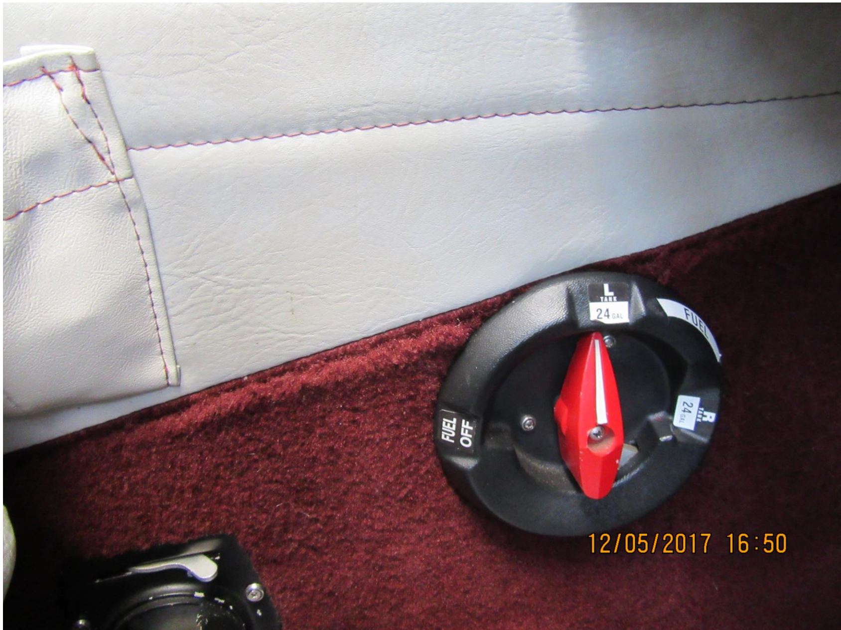
Photo 3 – Fuel selector valve (FAA)
