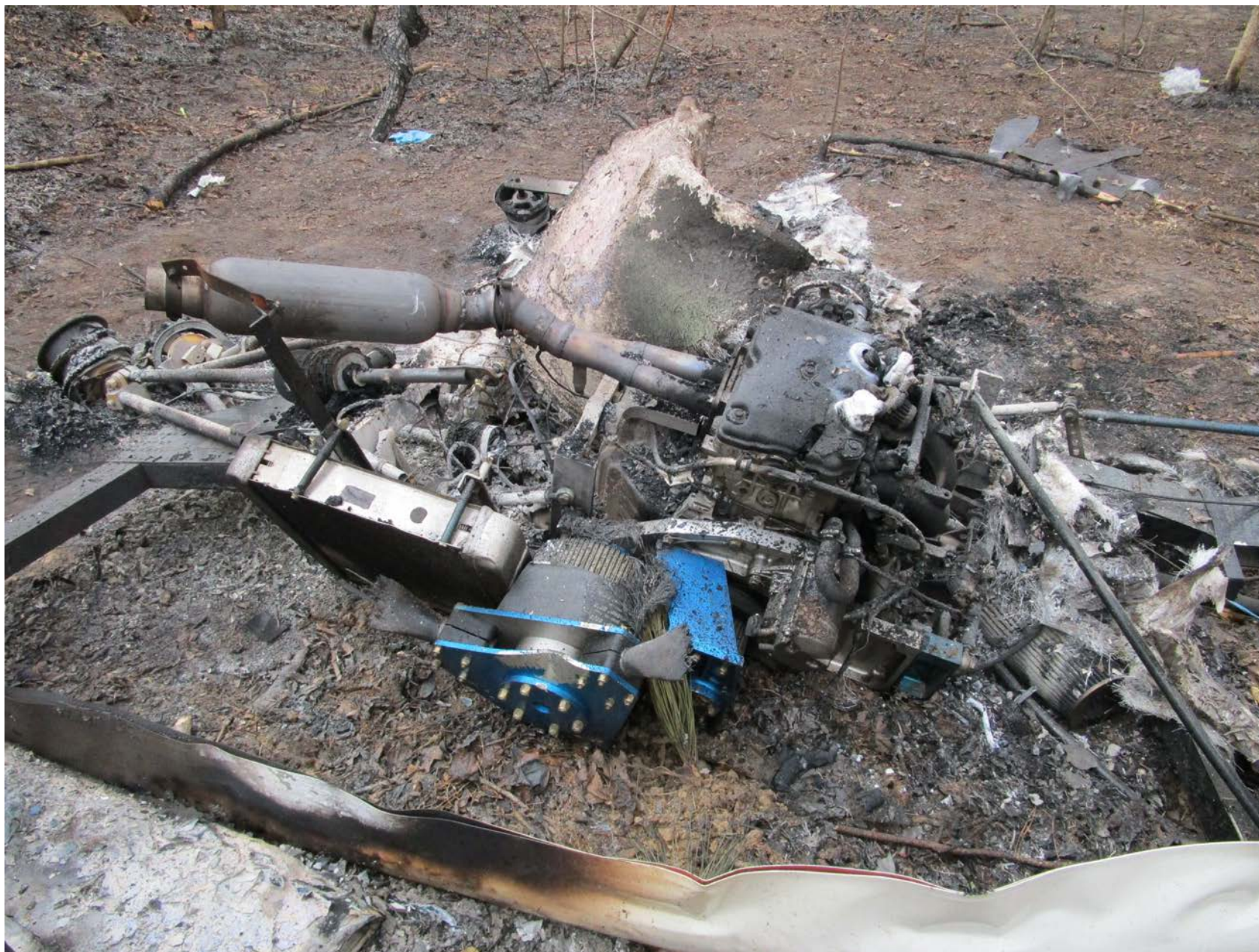
Photo 4 – FAA Digital Photograph. View of the Heat Damaged Engine Assembly, Propeller Hub, 2 shattered Propeller Blades, and Section of Main Rotor Blade.
