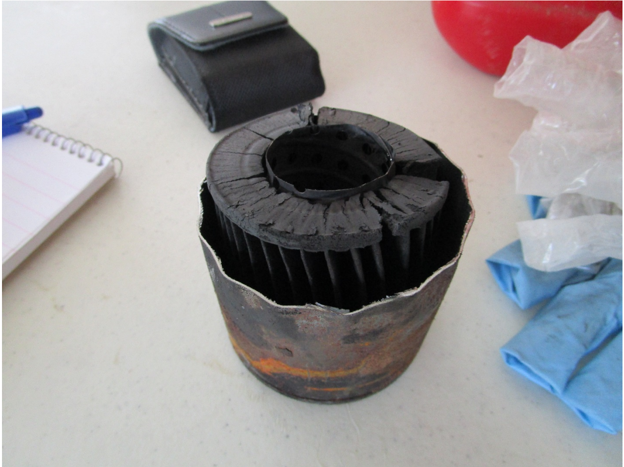
Oil filter cut open, heat damaged due to post crash fire.
