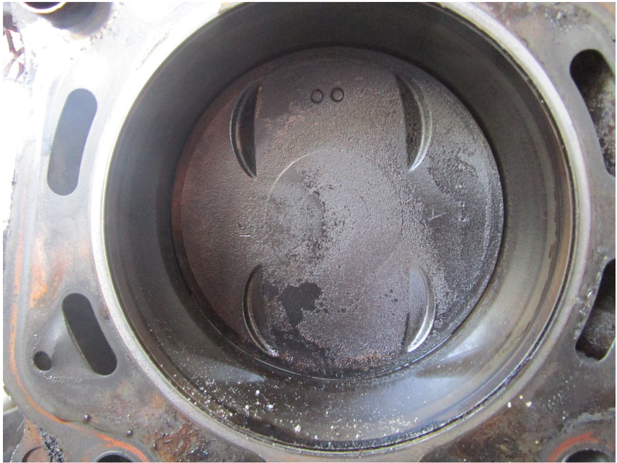
Right front cylinder/piston, again debris was introduced during disassembly.
