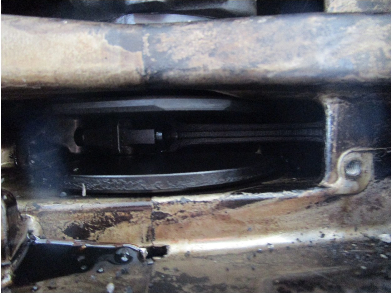
Close up of the rod connection to the crank shaft. #4
