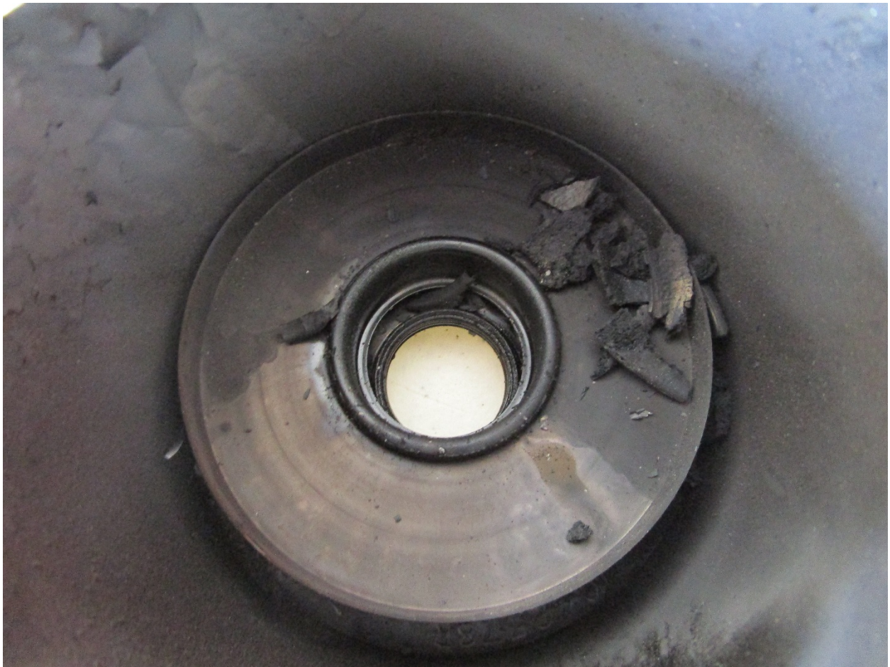
Inside of oil filter housing, debris from brittle oil filter element.
