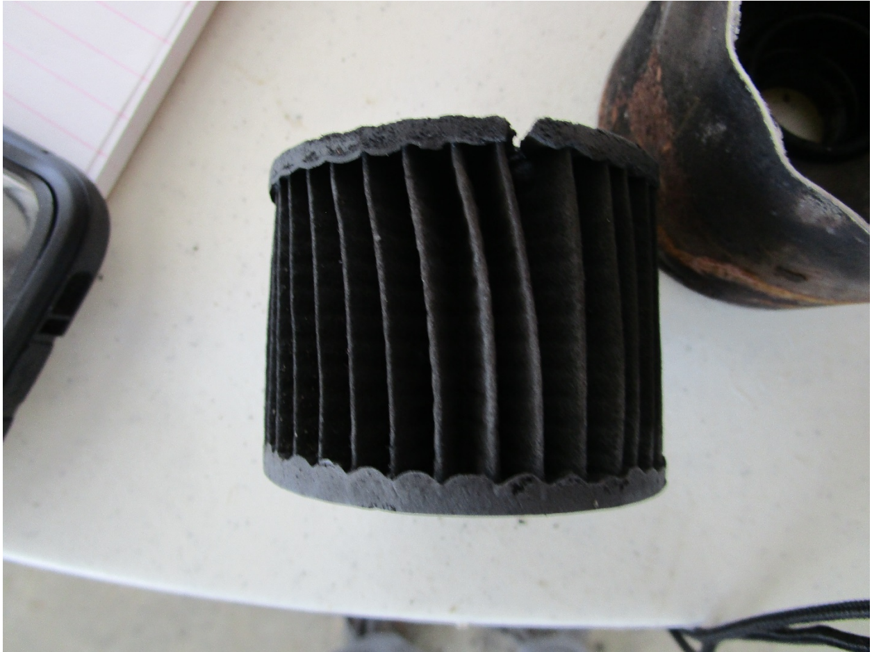
Oil filter element brittle from heat due to post crash fire. No metal found in filter.
