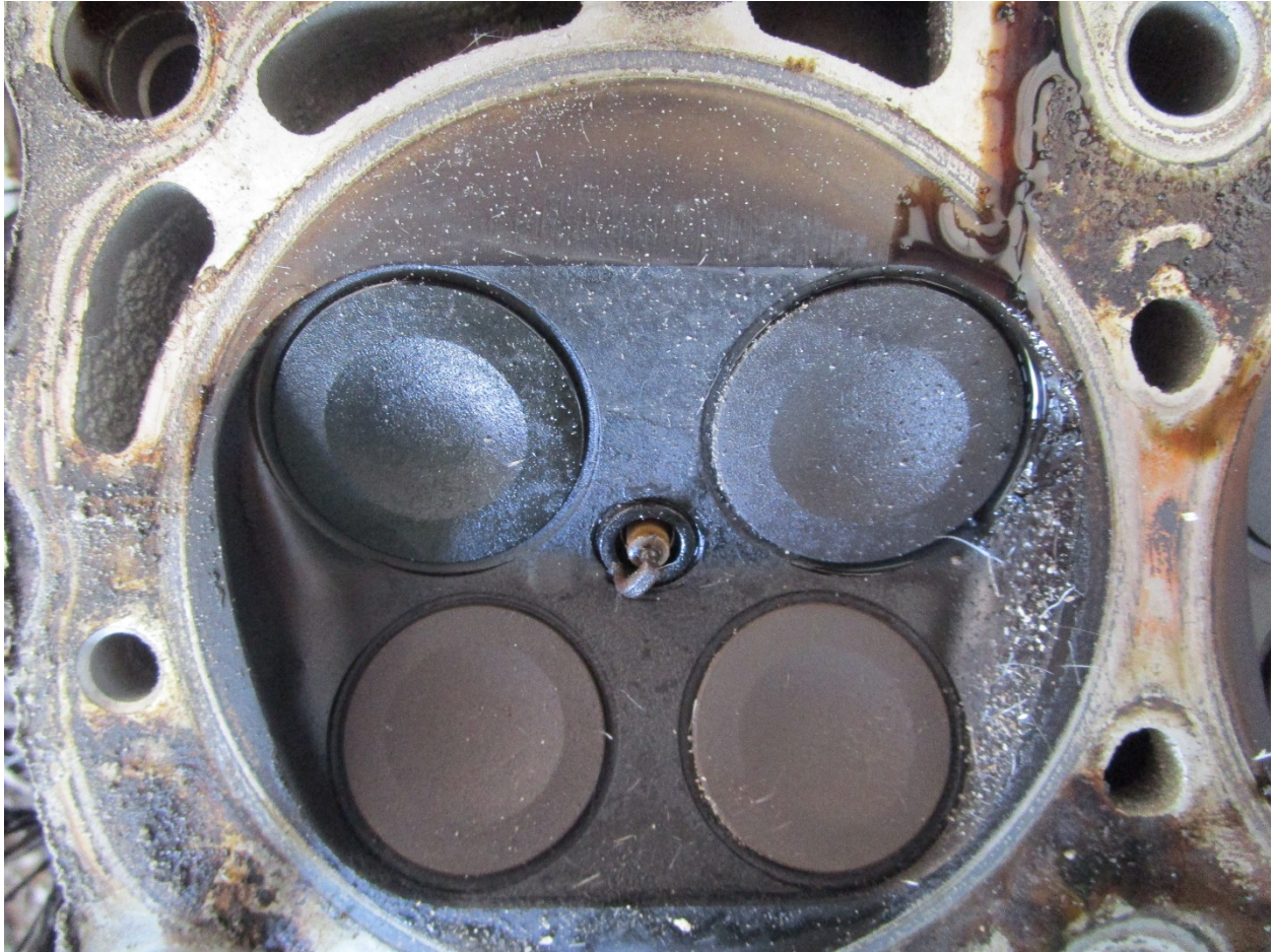
Right front cylinder head/valves/spark plug tip. All showed no abnormalities.
