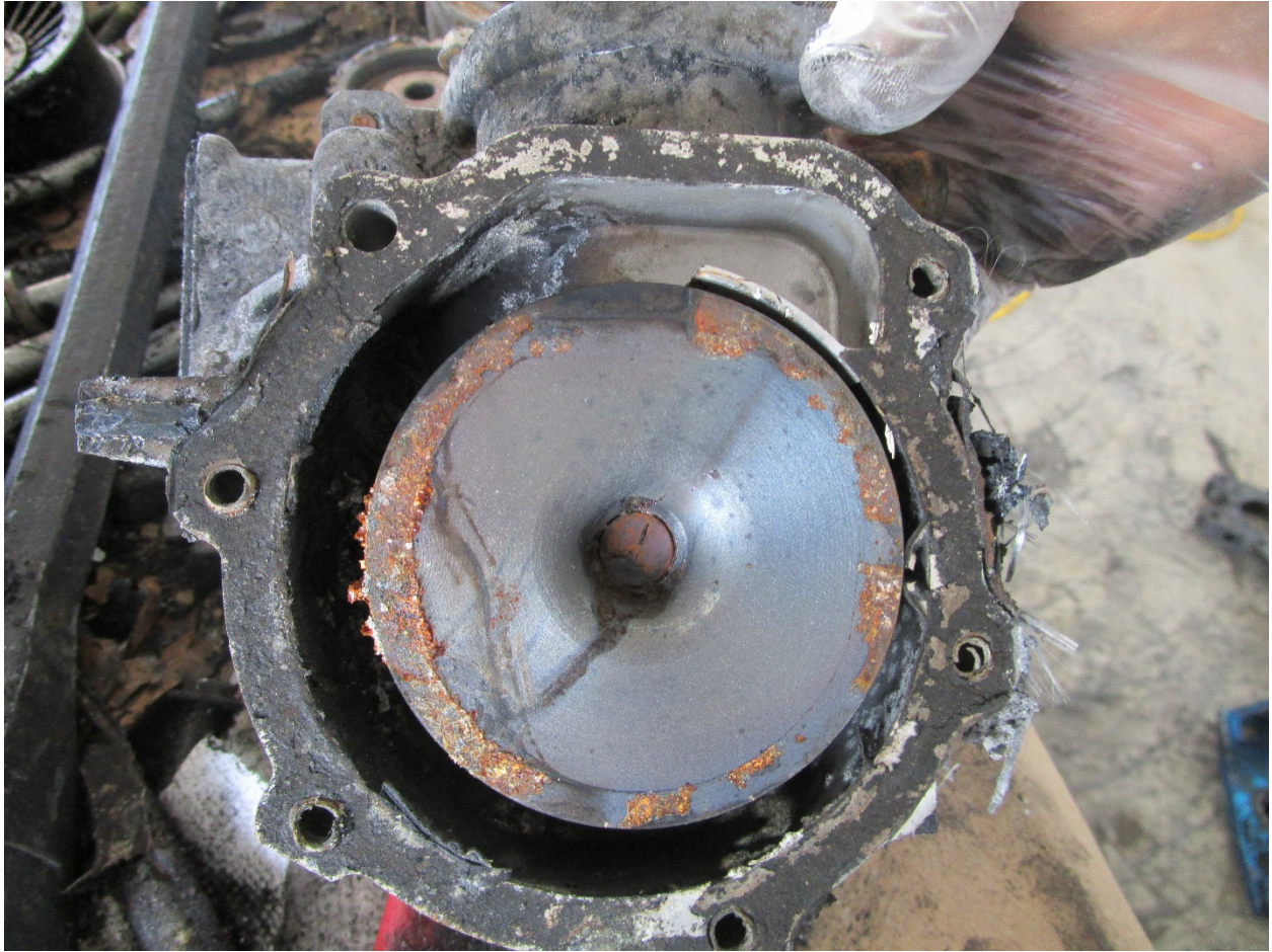
Water pump assembly, would not rotate due to corrosion and damage from crash.
