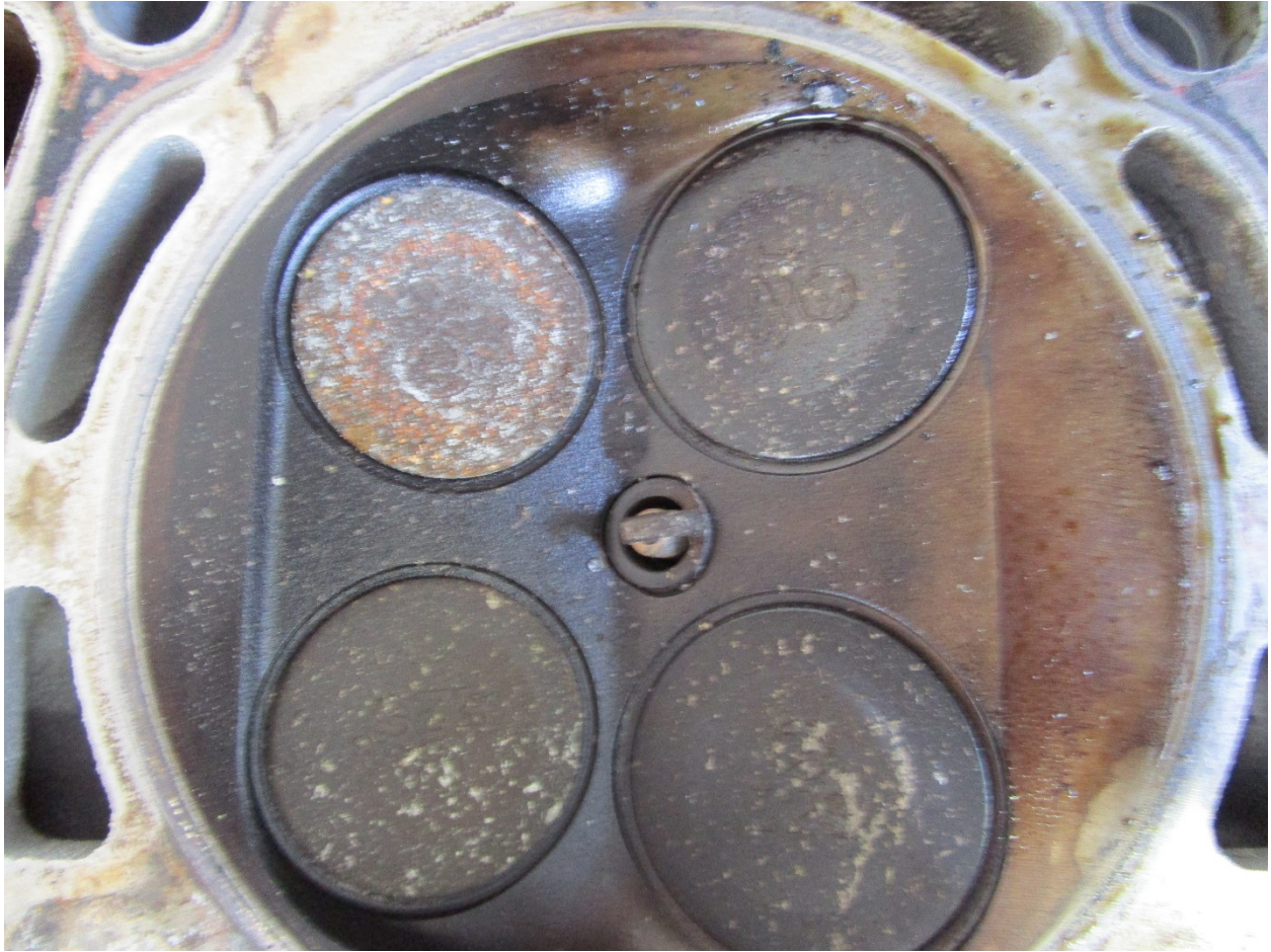
Cylinder head from the right rear cylinder, again indicated normal wear and spark plug tip showed no abnormalities.
