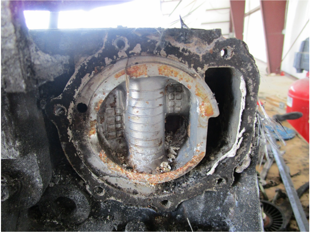
Water pump housing on the front of the engine, debris introduced during disassembly.
