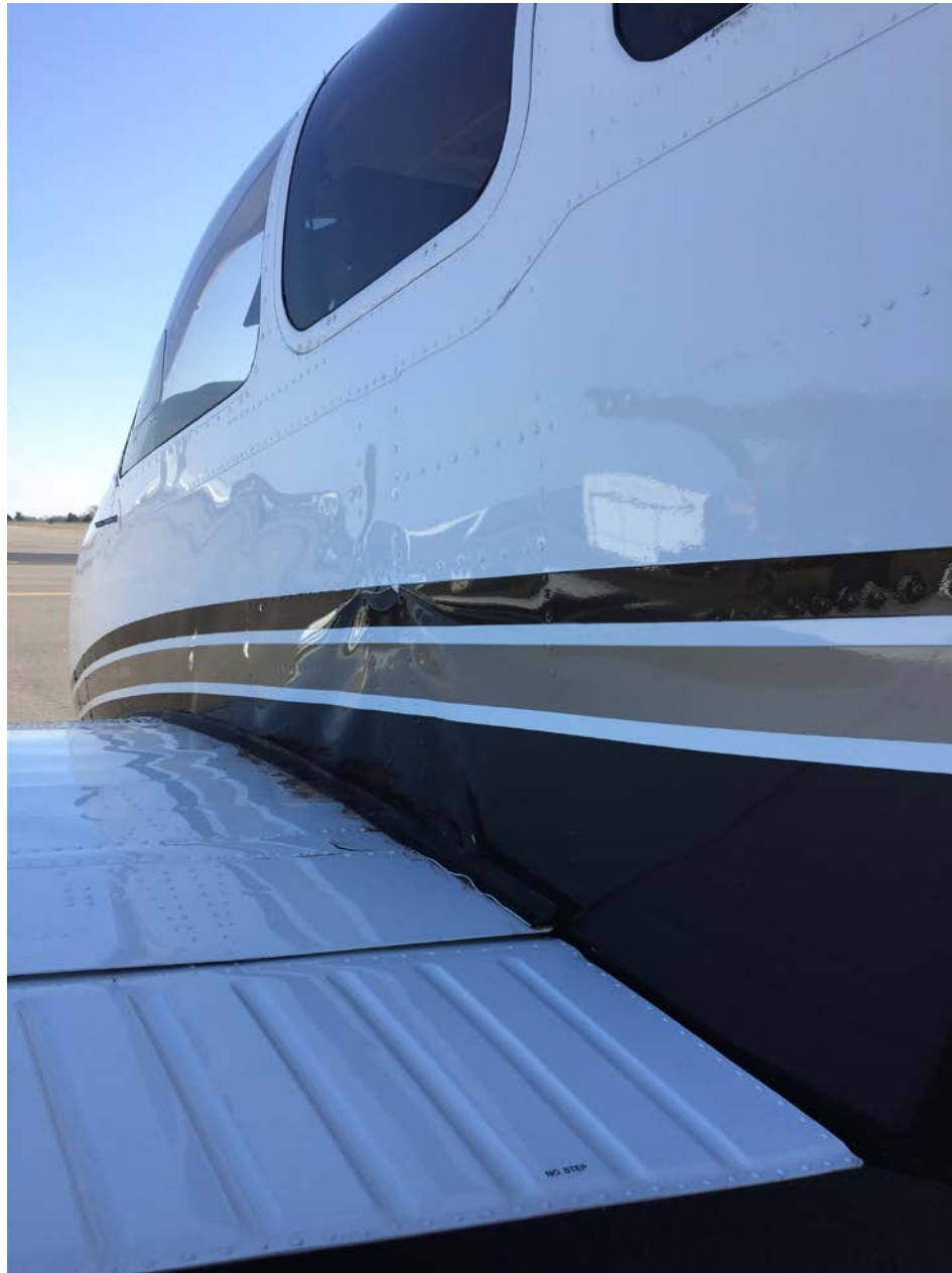
Photo 3 – View of the left side of the fuselage over the left wing root displaying airframe buckling (Courtesy of the FAA)
