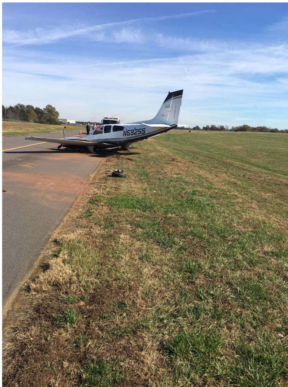
Photo 1 – Left side view of airplane on taxiway with left main landing gear wheel separated (Courtesy of FAA)
