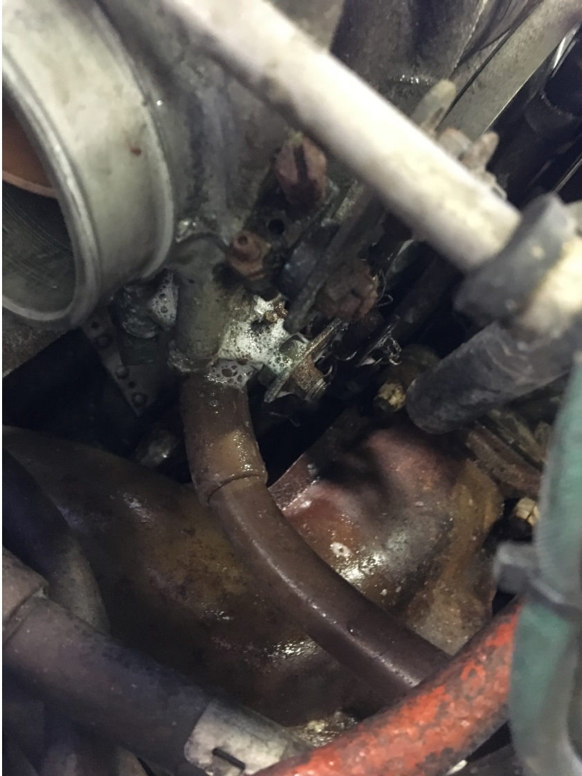
Photo 2: Leak at the mixture control arm on fuel injector system
