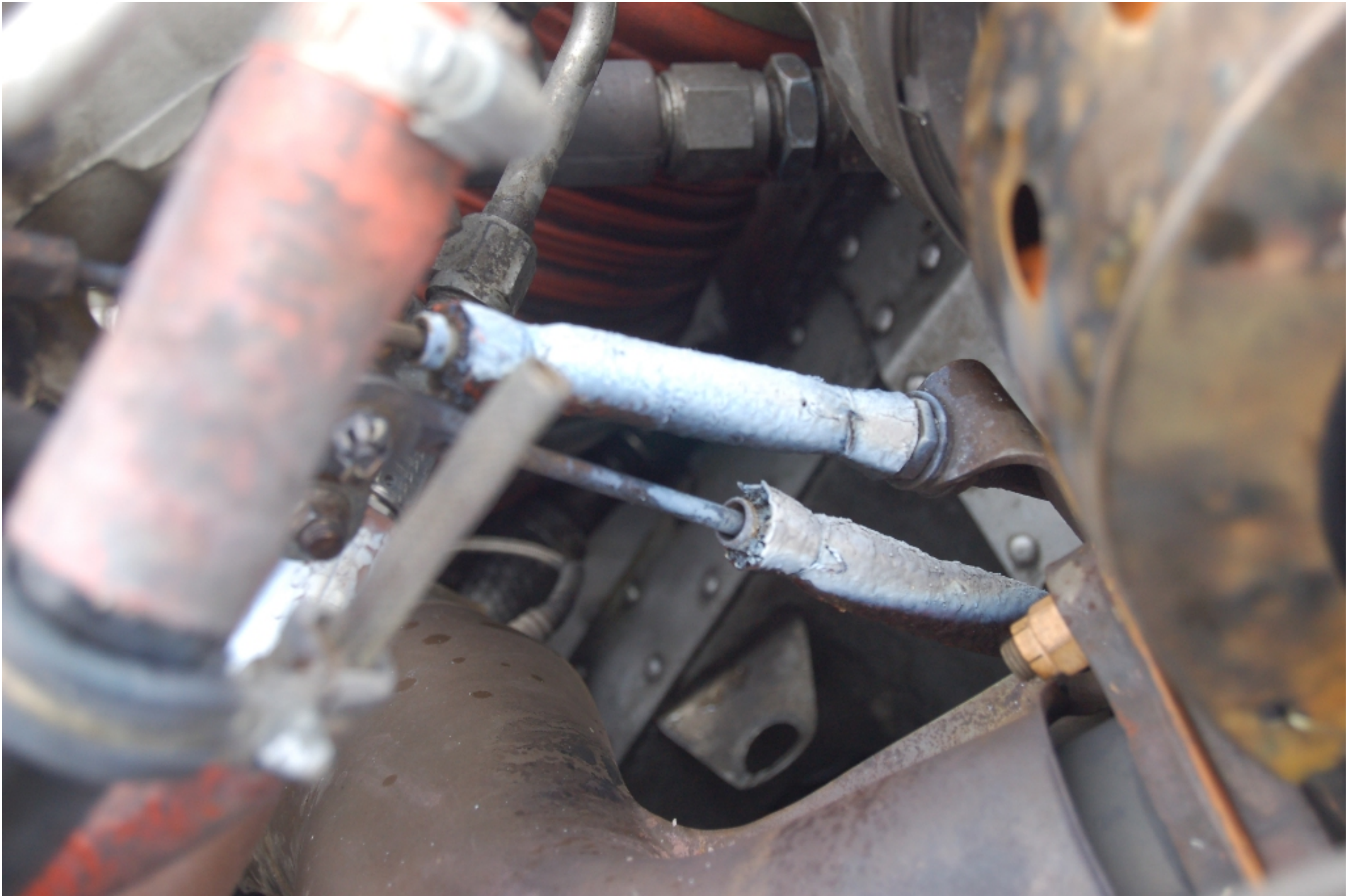
Photo 4 – Discoloration on Left Engine Components (FAA Photo)
