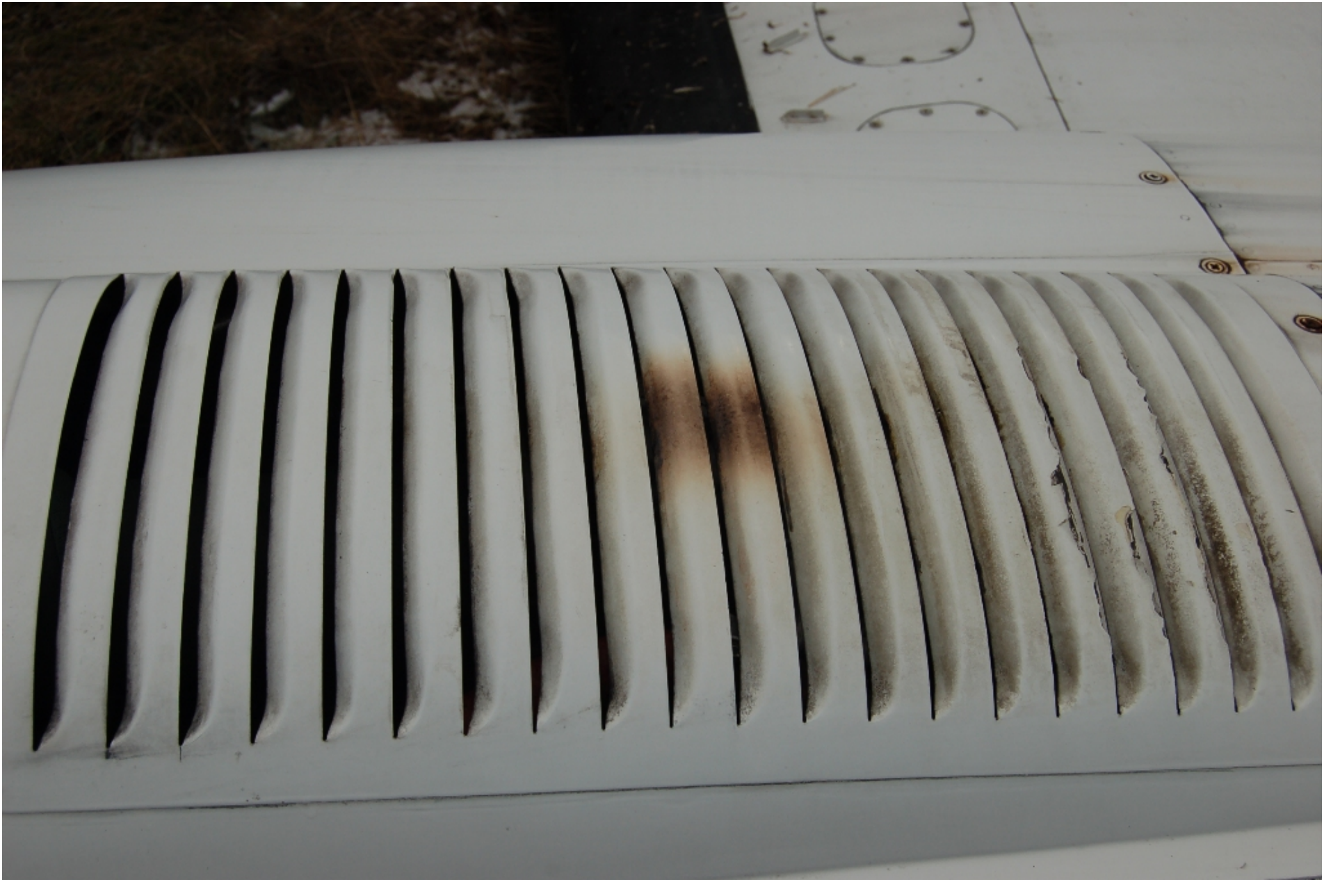
Photo 3 – Fire/Heat Discoloration of Left Engine Nacelle Louvers
