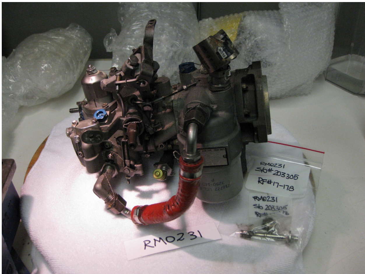
Picture 1. View of Fuel Pump and Fuel Control Unit
